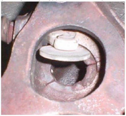
This is a very common problem with Turbochargers, especially Internally wastegated ones. Over time, the heat just breaks down the cast, and it starts to crack. This one was so bad I could see light all the way through it. Most of the time you can still use turbos if they have hairline cracks, But when they are this bad, and causing boost problems, its time to get a new exhaust housing.
