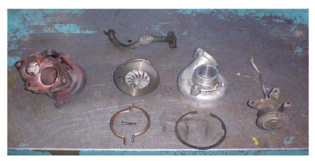
Exhaust Housing - Turbine (center section) - Compressor - Internal Wastegate
