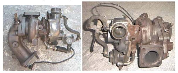
You can see how small and compact this turbo is, which makes it very easy to work with. It is both Oil and water-cooled. Some people chop the O2 housing downpipe section in half so they can get a better angle with the downpipe.
