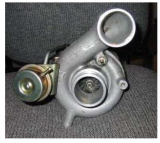
The Compressor housing makes the T-25 turbocharger very easy to work with.
