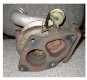
The exhaust housing is the same on all the DSM turbochargers (4g63) You can see how much smaller the exhaust wheel is than the 14b Turbo. The wastegate is also different than the 14b turbo, and they cannot be interchanged.
