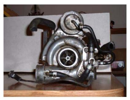
The IHI RHB5 Turbo, a few different styles of this turbocharger, This turbo is the Ford Probe/Mazda MX6/ 626 Turbocharger. It has a circular inlet flange, and wastegate that is set at 8psi.
