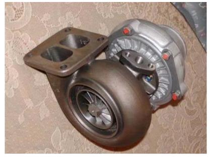
The Big Bad Boy Turbo, T4 turbo. Their are many series of these turbos, I am not fimilar with that many of them, since I have never used one. These are for very large HP applications. Mainly v6 or v8's. Some heavily built race Honda B/D series motors can be used with these, mainly for drag racing.
