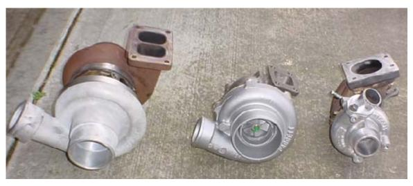
T4 Turbocharger (Diesal Truck) - T3/04e Turbocharger - 14b DSM Turbocharger
