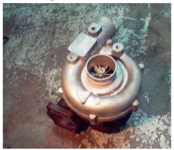
This is the KKK Turbocharger, The KKK turbo comes from Germany, many European cars use these turbos. Audi/VW/Porsche and others. This turbo shown the KKK 26 I belive, is similar to a basic T-3 turbo. The inlet flange is identicle to the T-3 turbo. But some other KKK turbo's have very odd looking inlet flanges.
