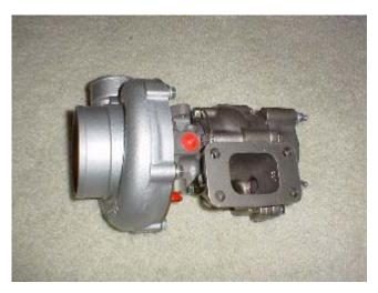
Hybrid Turbochargers, T3/T4 Turbos... The concept of using a small center section to spool fast and using a large Compressor for more cfm. These turbos are one of the best to use. Especially on B-series Motors. T3/T4's can support anywhere from 300-450hp. Some can come internally gated or external. This is a .70ar compressor .63 exhaust
