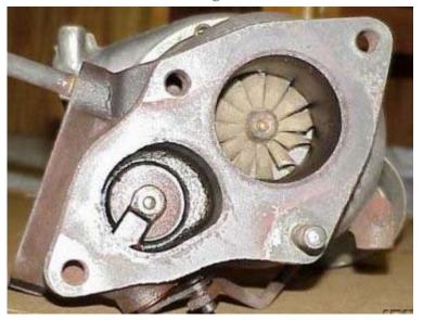
This is what makes the 14b such a great turbo, the exhaust wheel is one of the largest for a factory Turbo'd 4cyl cars. You can see the wastegate flapper to the left.
