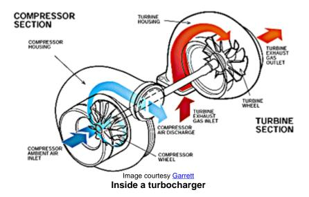
On the other end of the shaft that the turbine is attached to, the **compressor** pumps air into the cylinders. The compressor is a type of centrifugal pump -- it draws air in at the center of its blades and flings it outward as it spins.
