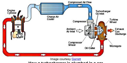
How a turbocharger is plumbed in a car
