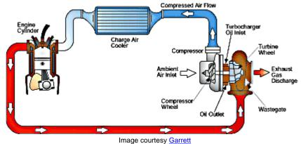
How a turbocharger is plumbed (including the charge air cooler)
