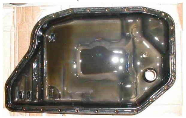
The fluid is drained, and the pan is off! There is a good amount of sediment in the bottom of the pan. The four small rectangles are magnets to collect any steel particles. Mine had some sludge on them, but it appeared to be normal wear.
