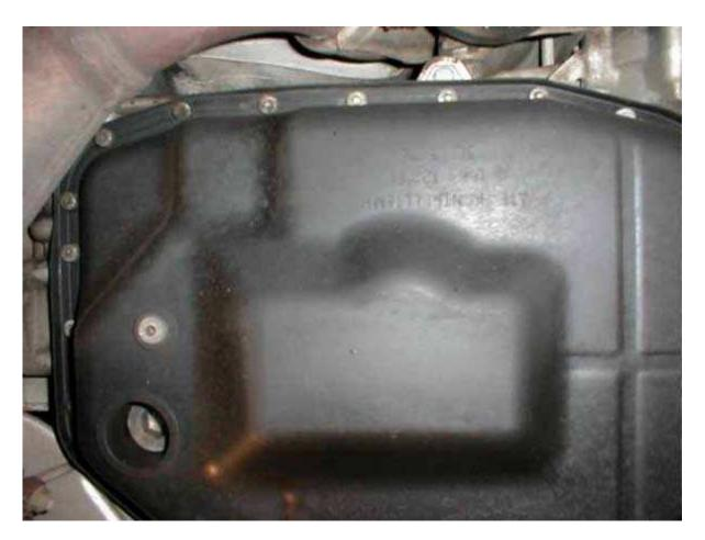
This is the transmission pan. The small bolt is the drain, the large one is the fill. The bolts are Torx bolts, size T-27. Why Torx and not Allen? Why T-27 instead of the more common T-25 or T-30? We must all make sacrifices to the Audi Gods.
