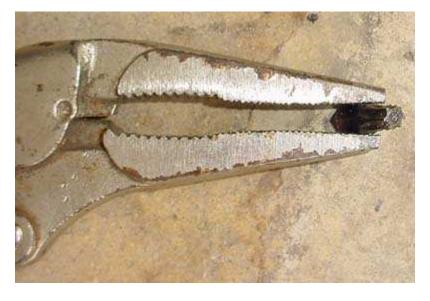
Ground down T-27 bit in vice grips. This will allow you to get the two hidden T-27 screws out without dropping the exhaust.
