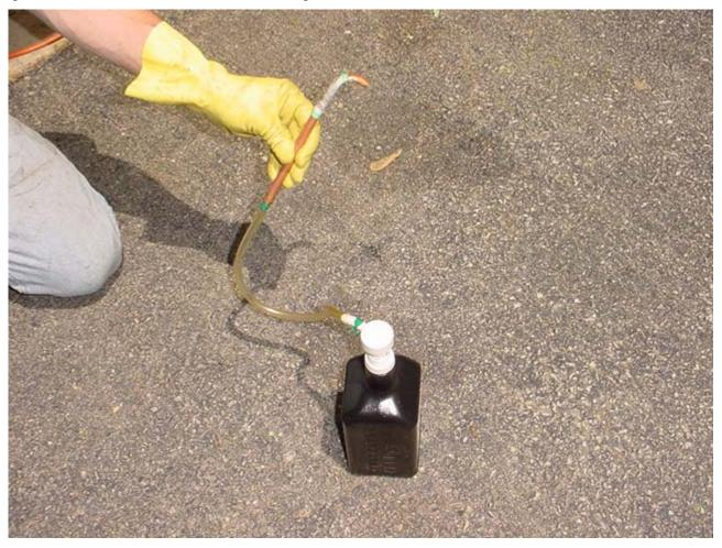
Marine pump with copper tube fitted to pump oil into the transmission.
