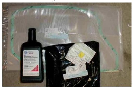
These are the parts you need: pan gasket, new screen, and super special VW/Audi transmission fluid (at \$12 -15/quart, you should buy 8 quarts). Remember to also buy new crush washers for the drain and fill plugs (I didn't and if the originals leak I will be very mad).
