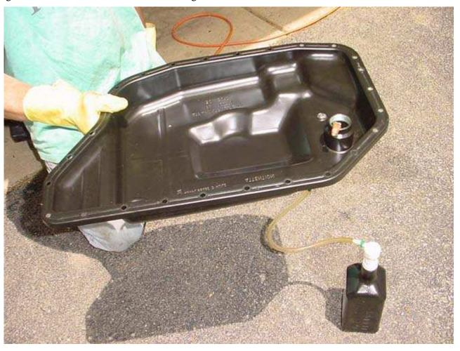
How pan stand pipe works to control level. Fluid is pumped into the transmission pan until the level reaches the top of the stand pipe. It then overflows out of the transmission. This level is higher when the car is not running versus running due to the hydraulic pump pumping fluid through the transmission.
