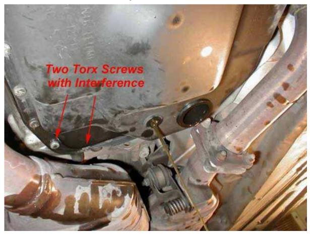
Transmission fluid draining. Be prepared for about 6-7 quarts to drain. Note that the Audi fluid is not red like every other transmission fluid. It's sort of yellowish green. Mine was in much better condition than I anticipated. It was still clear, not burnt and did not smell rancid or overheated.
