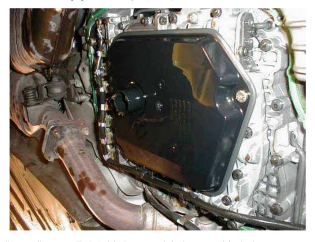
The filter is still bolted to the transmission with two bolts. Remove them and it comes down. Note that there is a rubber o ring on the output of the filter. Note that those two bolts are different than the trans-pan bolts (shallower head).
