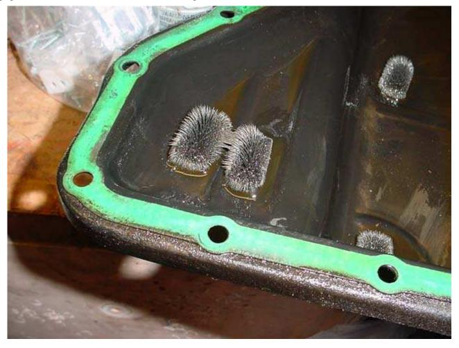
Pan magnets completely full of metallic particles. Is this an Audi Chia Pet??
