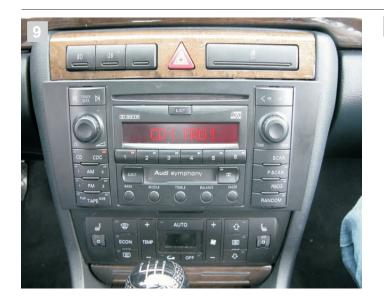
9. Verify all connections and re-install the radio back into the vehicle by sliding it into the tray until it locks into place. Route the docking cable as desired.
