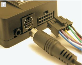
7. Connect the vehicle specific cable's 8-pin molex connector and iPod Docking Cable to the DICE module.
