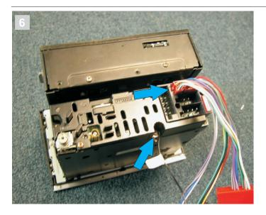
6. Insert the vehicle specific cable into the specified connector. Make sure the connector is fully inserted and that it snaps in place.
