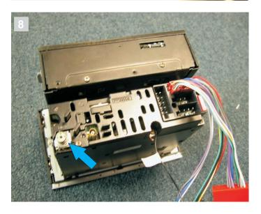
8. Connect the remaining adapters and antenna leads back into the radio and prepare for re-installation.
