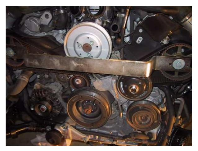
D6. Mark the harmonic balancer so you know which way it goes (probably not 100% necessary as it has its own mark, but what the heck) and remove it from the end of the crank shaft.
