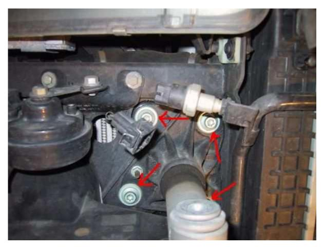
B19. Lift on whole lock carrier and slide it outward a few inches. Have something to support it with as it is fairly heavy. Now hinge it left a little bit like it is a gate. Be careful not to stress the hoses or connections. Just make enough room that you can work behind it. Figure out a good way to support it there for a while.
