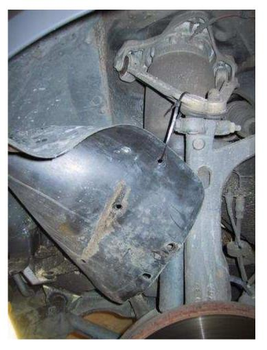
A2. Now look behind the liner toward the front bumper. What you are after are the three 10mm nuts on each side aligned in a vertical column. Remove them with an extension on your ratchet.
