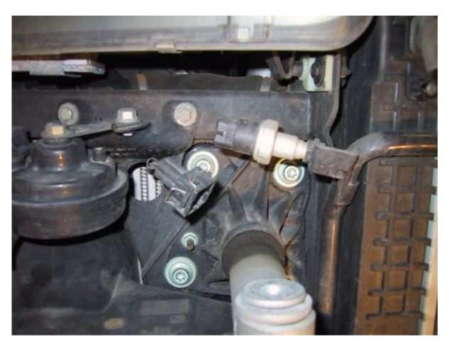
B8. Disconnect electrical connector on two horns left and right.
