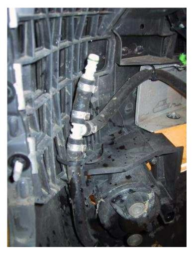
A8. Pry the bumper (with strong hands) away from the fender at the wheel well to pop it out of the guide that it is mounted to. I had difficulty with this and was surprised how much force I had to use to free the bumper from the bumper guide. Pop out both sides.
