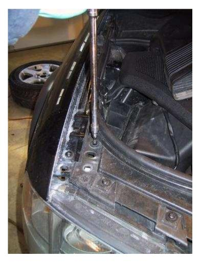
B17. Remove 2x T-30 torx bolts oriented horizontally in sides near turn signals.
