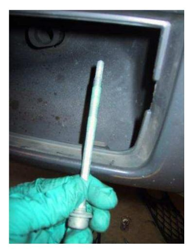
A5. Remove 2x per side T-20 torx attaching bumper to the 'bumper guide' where you peeled back the fender liner.
