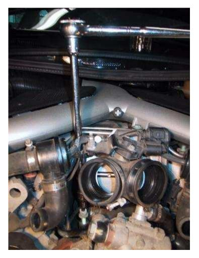
D16. Remove water pump. 2x 10mm nut including dipstick nut already removed and 9x 10mm bolts.
