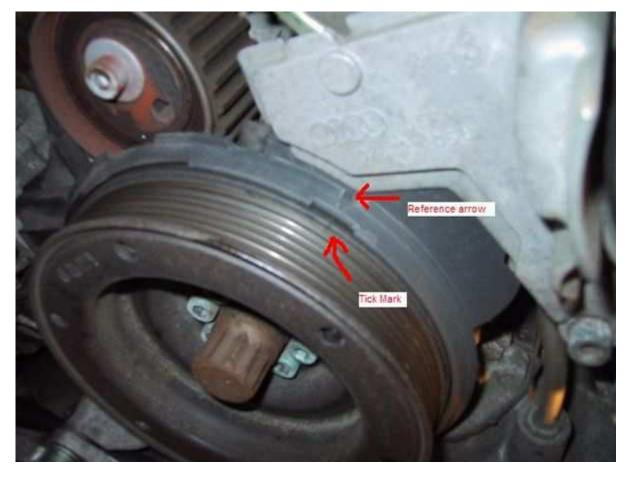
When you get the mark lined up on the crank pulley take a look at the wing like brackets on the outside of the cam sprockets. If the larger holes are OUTBOARD as in this picture you are **not at TDC** and the cam lock bar will not fit on this way.
