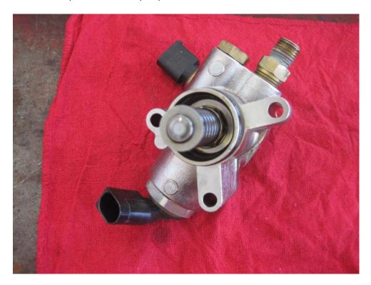
16. Per Bentley manual it is recommended that you replace the round fuel pump seal. The following photo shows the seal to be replaced. Audi part number for the seal is 06E 127 248. It costs \$9.68 from my dealer.
