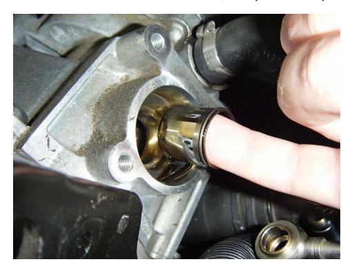
The cam lobe can be seen in the following picture. In this particular case there's hardly any wear on the surface of the lobe.
