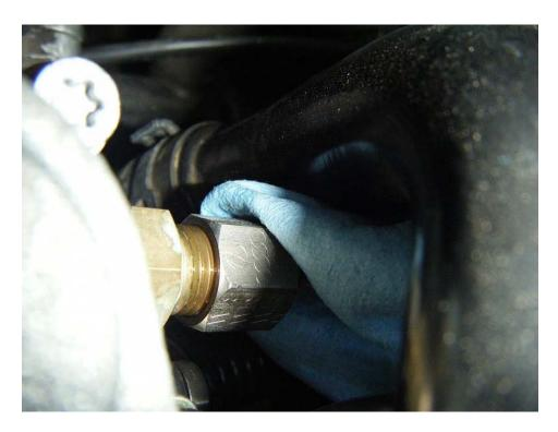
The fitting is off and the line is out of the pump fitting:
