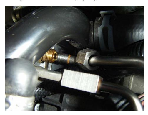
10. Now, using 12-point 8mm torx bit remove the banjo bolt from the pump
