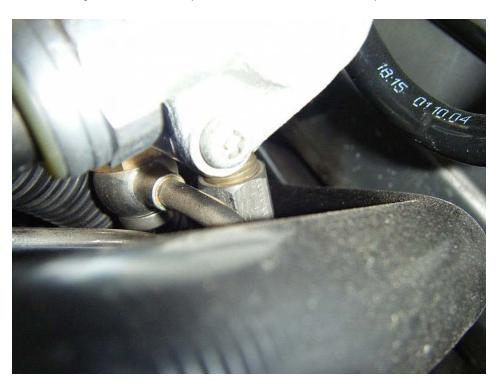
9. First, remove the high pressure line. Make sure to stuff a paper towel/work rag underneath the fitting to catch any fuel spray and drips. Use a 17mm open wrench. Suggestion: use a short wrench so that you can easily maneuver it under the coolant line, electrical wires and hoses. The fitting isn't too tight so the force applied to twist it is minimal.
