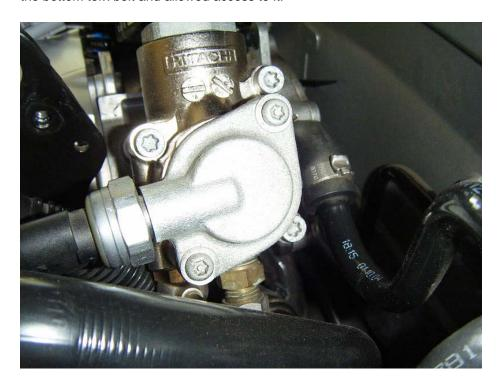
A sample setup to be used to remove the torx screws holding the pump pictured in the photo below. I used something very similar. Do not remove the torx bolts just yet!
