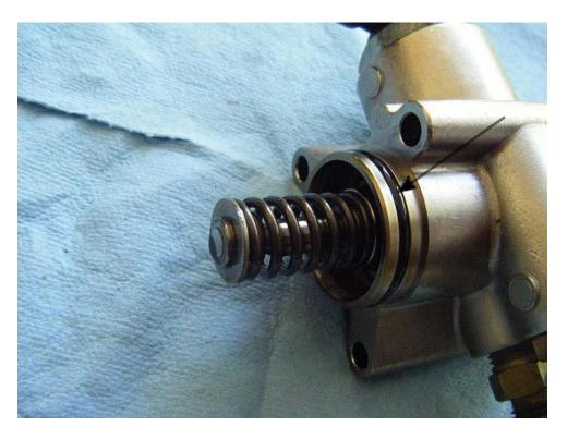
17. Time to put a new cam follower in place. Audi part number for the cam follower (sleeve) is 06D 109 309 C. It cost me \$43.20 from dealer. Carefully place the new follower into the pump opening.
