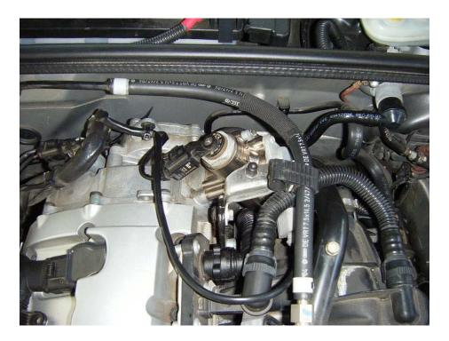
2. Remove the plastic clip holding the flexible low pressure fuel line from the mount on the engine. Then open the clip and slide it along the hose and remove it from the hose.
