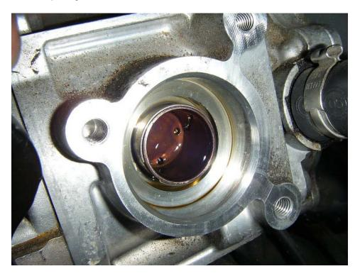
18. Place the three torx bolts into the pump and set the pump in place to be secured. Once the pump is fully seated and all three bolts are in finger-tight, use a torque wrench to tighten them evenly to 10Nm or 7.4lb-ft. The bolts are quite long; over-tightening them could stress them and cause a failure that would put the pump on quite a bind. If you are unsure about what torque the bolts are in, remove them one at a time and re-torque them to make sure.
