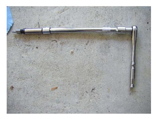
In the setup pictured above the person used a 10" 1/2" drive extension with a 3/8" to 1/2" adapter and a 1/2" to 3/8" adapter. Overall length is equal to a 12" 3/8" drive extension. Plus/minus an inch or so would suffice.
