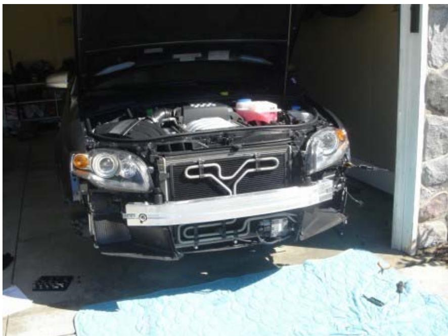
2. Remove Bumper Bracket Frame Bolts & loosen bumper bracket guide nut, but do not remove. (2 locations)
