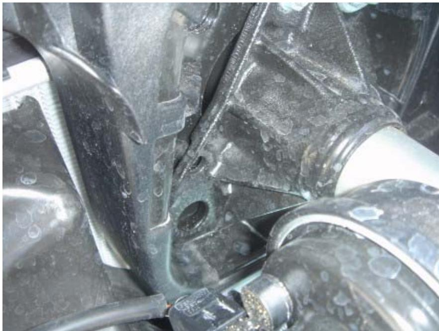
3. Locate OEM Snub beneath engine bay (adjacent radiater wall).
