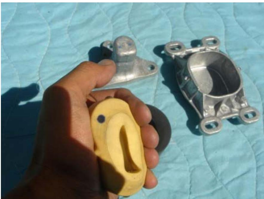
7. Install ECS Snub onto Snub male bracket.
