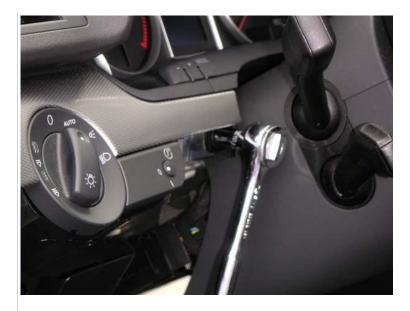
Once you get the bolts out, you need to remove the headlight switch assembly. To do this, you must turn the headlight switch just to the left of the "Auto" setting and push in, you will feel when you are in the right place because it will go in about a half an inch. Then turn to the right about 10 degrees and pull straight out. This took me a couple of tries, but when I got it right, I could feel it.
