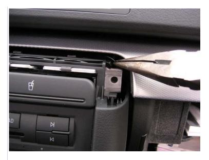
The whole thing pulls out straight. You may need to tilt the bottom of the trim upwards
