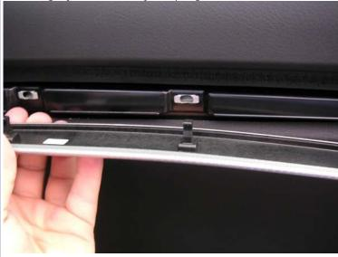
When you get to the end, the final clip slides out in the direction of the door hinge. Just simply push it towards the hinge and it will pop right out. The two rear doors have enough of an overhang that you do not need to use the screw driver to get them going. Just use your fingers to get the first one going.
