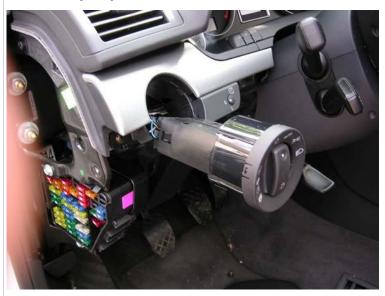
The lighting assembly of course has a few wires plugged into it. So too does the interior light dimming switch just to the right. Both can be easily unplugged and the unit themselves pushed through the trim (away from the dash). Once those are free, just put the lighting pieces into the new trim and re-secure everything. Do not put the lower dash back yet as you will need to access one of the bolts it covers when you replace the next trim piece.
