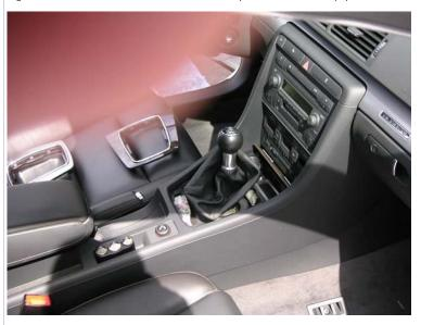
The trim piece just pulls straight up. It is secured by 4 little clips that fit into holes like
