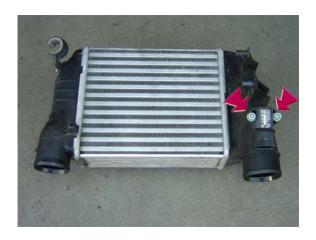
26. Remove sensor from stock intercooler an place it in a safe location for use at a later step.
