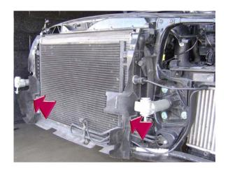
16. Remove the radiator ducts.
