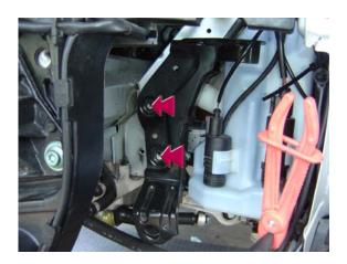
27. Remove the two hex bolts from the stock intercooler mounting bracket.
