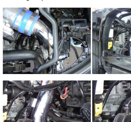
43. Slip the 2<sup>nd</sup> large hose clamp supplied onto the throttle body silicon piece and slide in the upper intake pipe. Tighten the hose clamp enough to still allow for the pipe to rotate freely inside the hose. Ensuring the pipe has been pushed in all the way rotate it in a clock wise fashion until the pipe comes as close as possible to the headlight tray without actually touching it. This is illustrated in the two lower images.
