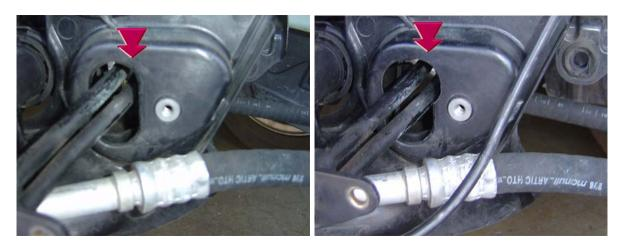
33. Use a rotary tool to enlarge the top portion of steering pump hole.
