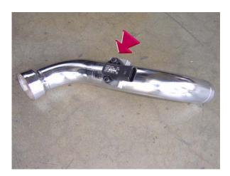
41. Attach the intercooler sensor to the flange located on the metal intake piping using the supplied black allen screws.
