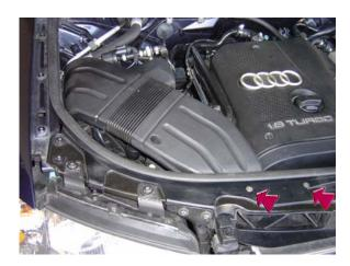
8. Remove screws for airbox channel & remove the channel.
