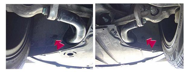
I. Remove the inner two screws on the inside of the fender liner, on both the left and right side.
