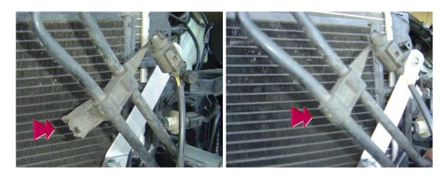
32. Use a rotary tool trim off the excess mount of the power steering cooler.
