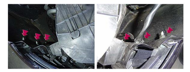
10. Remove the three 10mm nuts on the inside of each fender, underneath the headlights that fasten the bumper.
