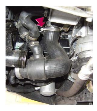
4. Loosen the clamp connected to the turbo outlet hose. Rotate it counterclockwise to relieve the tension. Do not disconnect.
