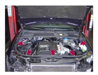
17. Completely remove the rubber hood seal that surrounds the engine bay.
