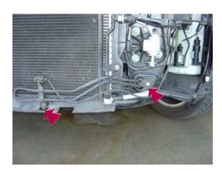
31. Remove the crew and bolt holding the power steering cooler in place as indicated by the arrows.
