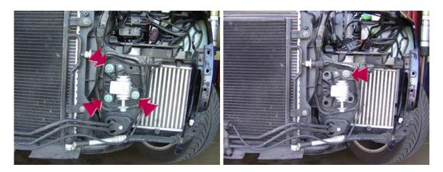
20. Remove the 3 torx 45s from around the bumper supports. Put one of the screws a few threads into the open service position. Repeat this on the passenger side as well. Pull the entire assembly forward. It will slide back 2 inches, and the weight will be supported by the service position screws. Do not put any additional weight on the assembly.
