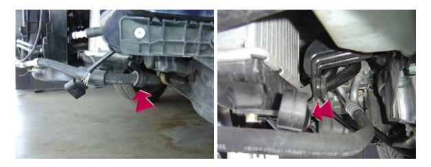
22. Snap off the ac hose from stock intercooler clamp.
