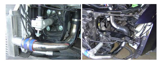
44. Attach lower intake pipe to the intercooler, line up the two intake pipes up and connect them together with the supplied 90 degree elbow. Be sure to tighten all hose clamps.
