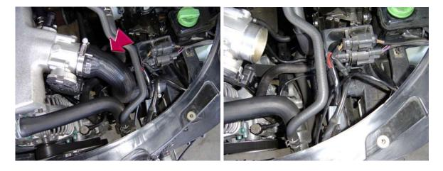
18. Remove the hose between the stock intercooler and intake manifold.
