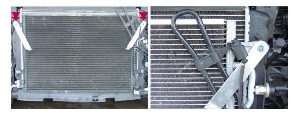
35. Remove the two top torx screws from AC condenser. Loosely mount intercooler support brackets on both sides and do not make them completely tight. Note: the power steering cooler needs to be placed underneath the driver's side bracket.
