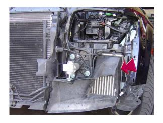
15. Remove the stock intercooler duct.
