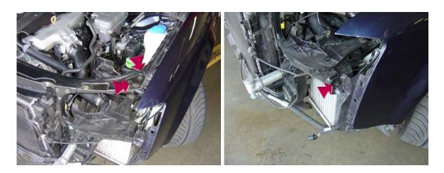
19. Remove the torx 30 screws on the top, and torx 30 screw from the side complete this on both the drivers and passenger of the car.
