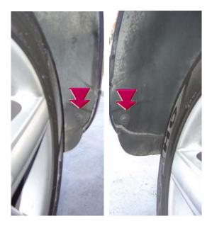
6. Remove the outer most screw on both the drivers and passenger fenders as indicated in the image. Turn the steering wheel to the left/right to assist.
