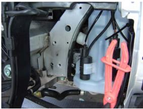
29. With the driver side fender liner removed undo the bolt from the rear of the washer reservoir that holds the intercooler mounting bracket in place as indicated by the arrow. Once removed slide the intercooler support bracket through the front and replace the removed bolt as it helps support the washer reservoir now secure the fender liner.
