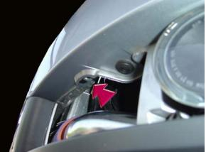
13. Using an allen wrench, loosen the two main bumper support bolts. Note: These bolts only need to be loosened enough to allow for the bumper support to slide forward there is no need to remove them completely.
