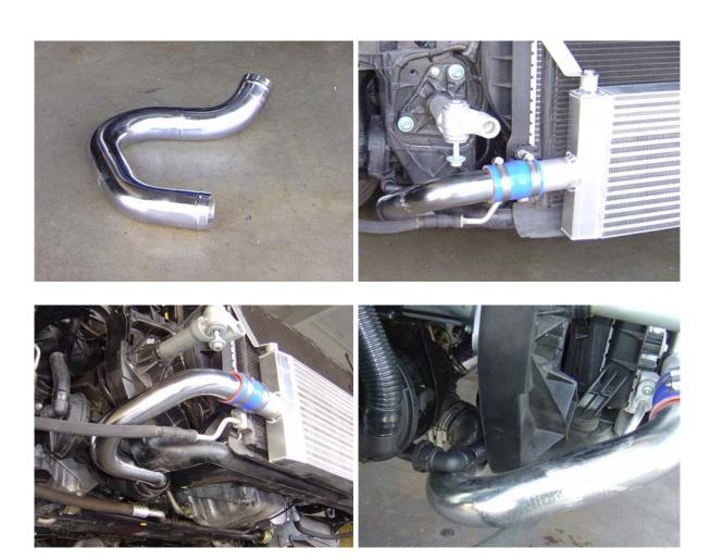
38. Slip a clamp over the passenger side silicone hose and install the intercooler piping as indicated by the images. Before tightening the clamp rotate the pipe as clock wise as possible to gently push up against the smog pump. Have someone hold the pipe in place pushed up against the smog pump while you tighten the clamp on the silicone hose.
