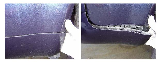
II. Gently pull outward to separate the lower bumper trim from the fender on both sides.
