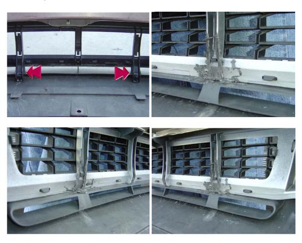
**45.** Using a rotary tool trim off the two areas indicated by the arrows. Note: this also applies to models equipped with the ultrasport front bumper.
