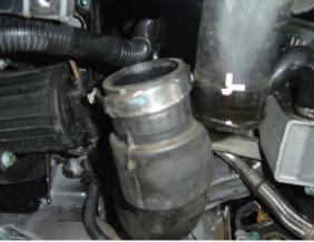
3. Disconnect the turbo outlet hose that is connected to the stock intercooler piping and move it to the side as shown.
