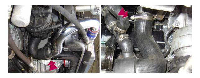
39. Slip the factory turbo outlet hose onto THE FMIC piping and tighten the factory hose clamp. Now tighten the factory clamp previously loosened at the turbo outlet. Note: Be sure not to slide the factory turbo hose too deep as the FMIC piping will block access to the diverter valve outlet connected to this hose.
