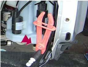
14. Pull the bumper forward and disconnect all wiring harnesses. Drain or plug the headlamp washer line.
