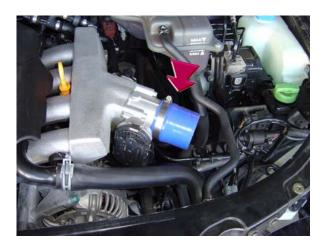
40. Slip the 2.5 silicone hose onto the throttle body and secure in place using of two larger hose clamps supplied with your kit.
