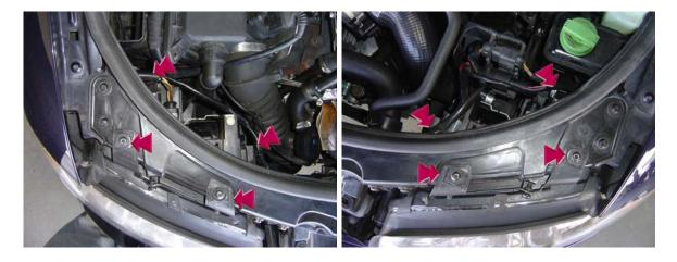
9. Remove both headlights by removing the torx screws. Disconnect the wiring harnesses.
