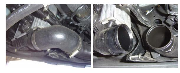
5. Disconnect and remove  $90^{\circ}$  elbow from the drivers side stock intercooler piping.
