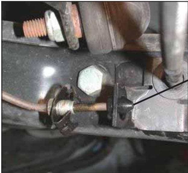
**Remove the hard line fitting, and place one of the rubber caps over the end of it, to control fluid loss during the installation.**
