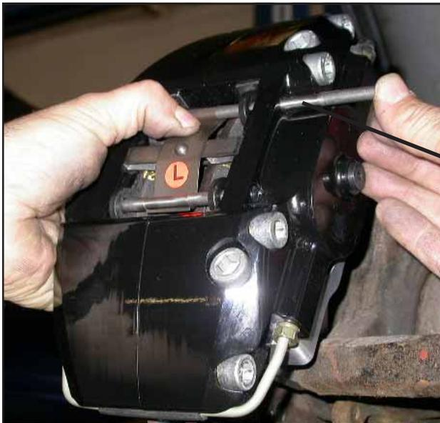
Slide the upper pad-retaining pin into the groove at the top end of the spring clip, and push it through to the inboard side of the caliper.
