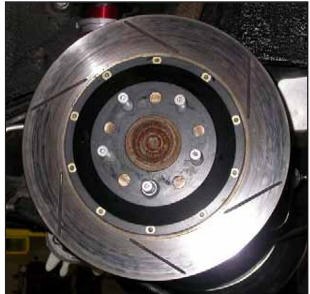
***Note: Take care to ensure that the rotor assembly is on the correct side of the car, as reversing the rotors will severely decrease the cooling capacity of the system. The rotors are clearly marked "L" and "R" with orange tags on the rotor hats. If the tags are not legible, the vanes inside the rotor should lean to the rear of the car on the top side of the rotor (see the following pages for more-detailed images).***
