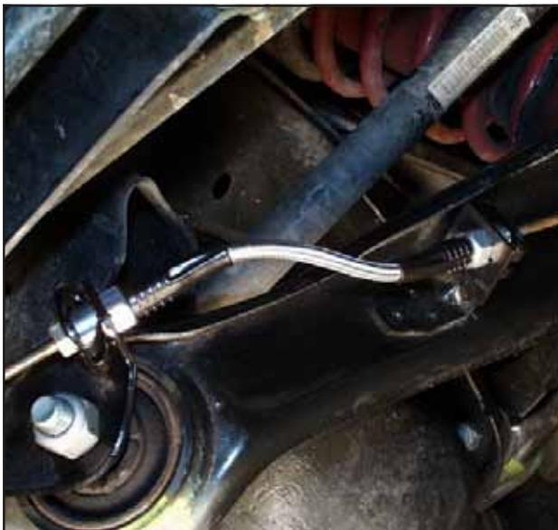
Install the shorter inboard stainless line in the same manner, but leave the fittings on both ends of the hard line loose until both ends are started. Then tighten all fittings.
