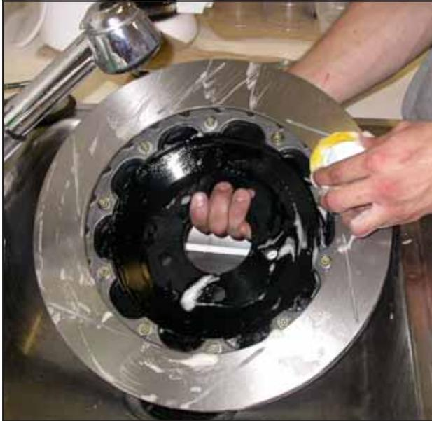
Even though the rotors may look clean, the rust inhibitor is in place, and it must be removed. Not cleaning the rotors will severely impact the performance of your new brake system.
