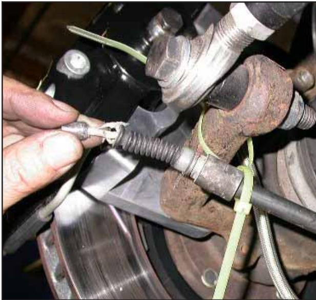
**Ensure that the end of the parking brake cable is held securely in place, and that it is not interfering with the movement of any other component.**
