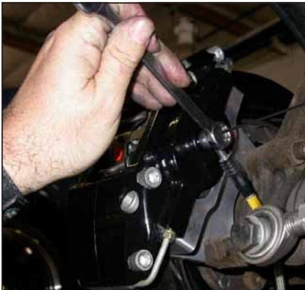
Tighten the banjo bolt to **approximately 14 lb-ft**, using a 14mm wrench or socket.
