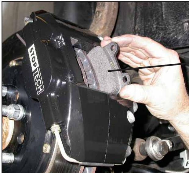
Slide the brake pads into position in the calipers, taking care to ensure that the friction side of each pad is facing the rotor.
