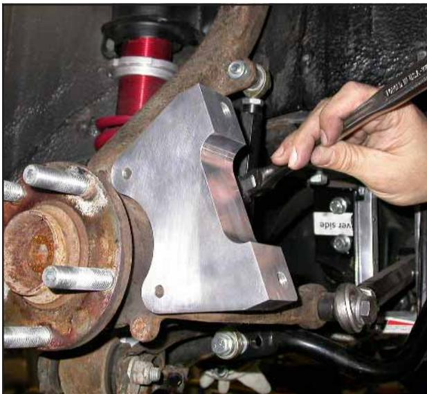
**Install the caliper bracket, using the stock caliper mounting bolts.**
