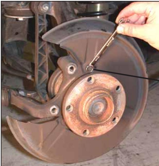
Remove the three dust shield bolts, using a 10mm wrench or socket, then remove the dust shield from the hub.
