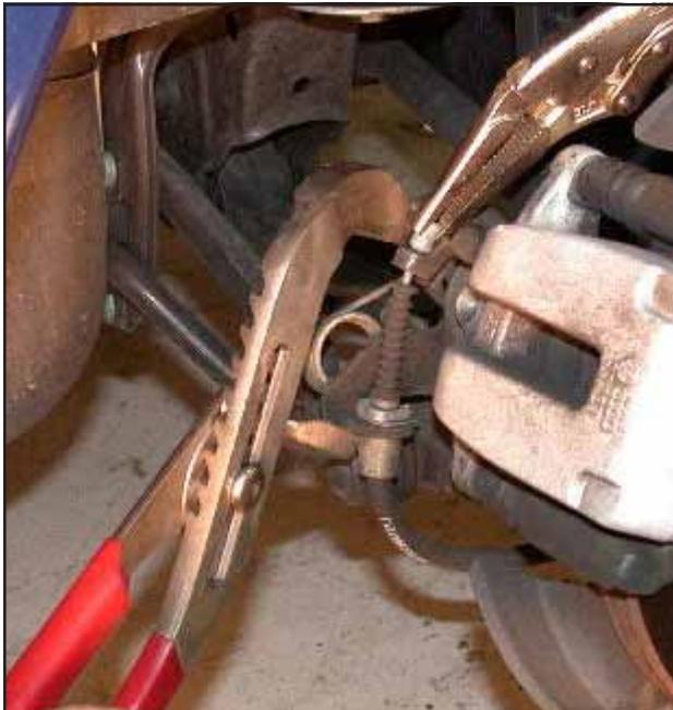
**Activate the caliper lever arm, using channel-lock pliers or a clamp to reduce the tension, then remove the cable end from the lever.**
