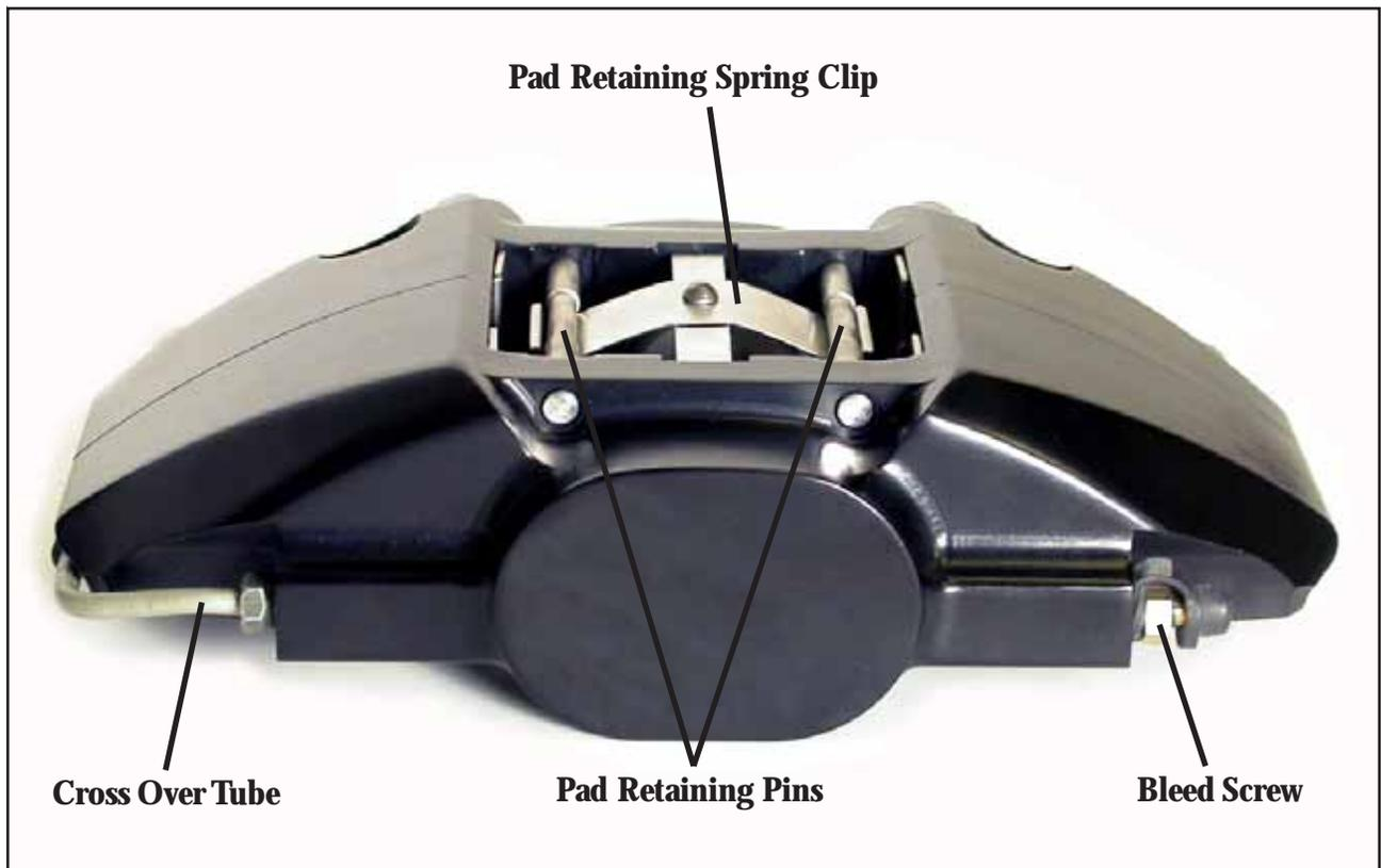
**The ST-22 original equipment caliper uses a pad that is common to two-piston opposed calipers. The Friction Materials Standards Institute (FMSI) number for the pad backing plate is D961.**
