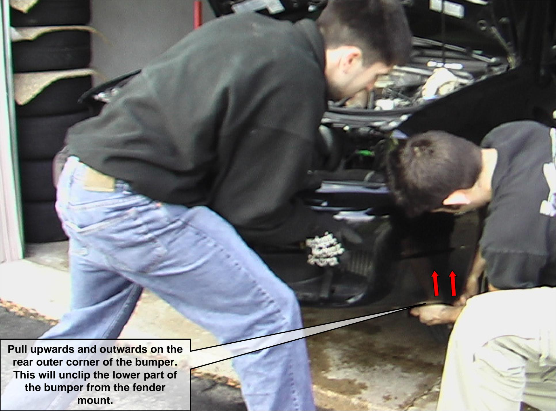
**Pull upwards and outwards on the rear outer corner of the bumper. This will unclip the lower part of the bumper from the fender mount.**
