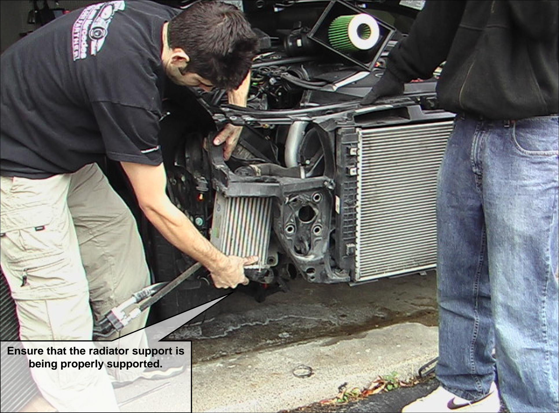
**Ensure that the radiator support is being properly supported.**
