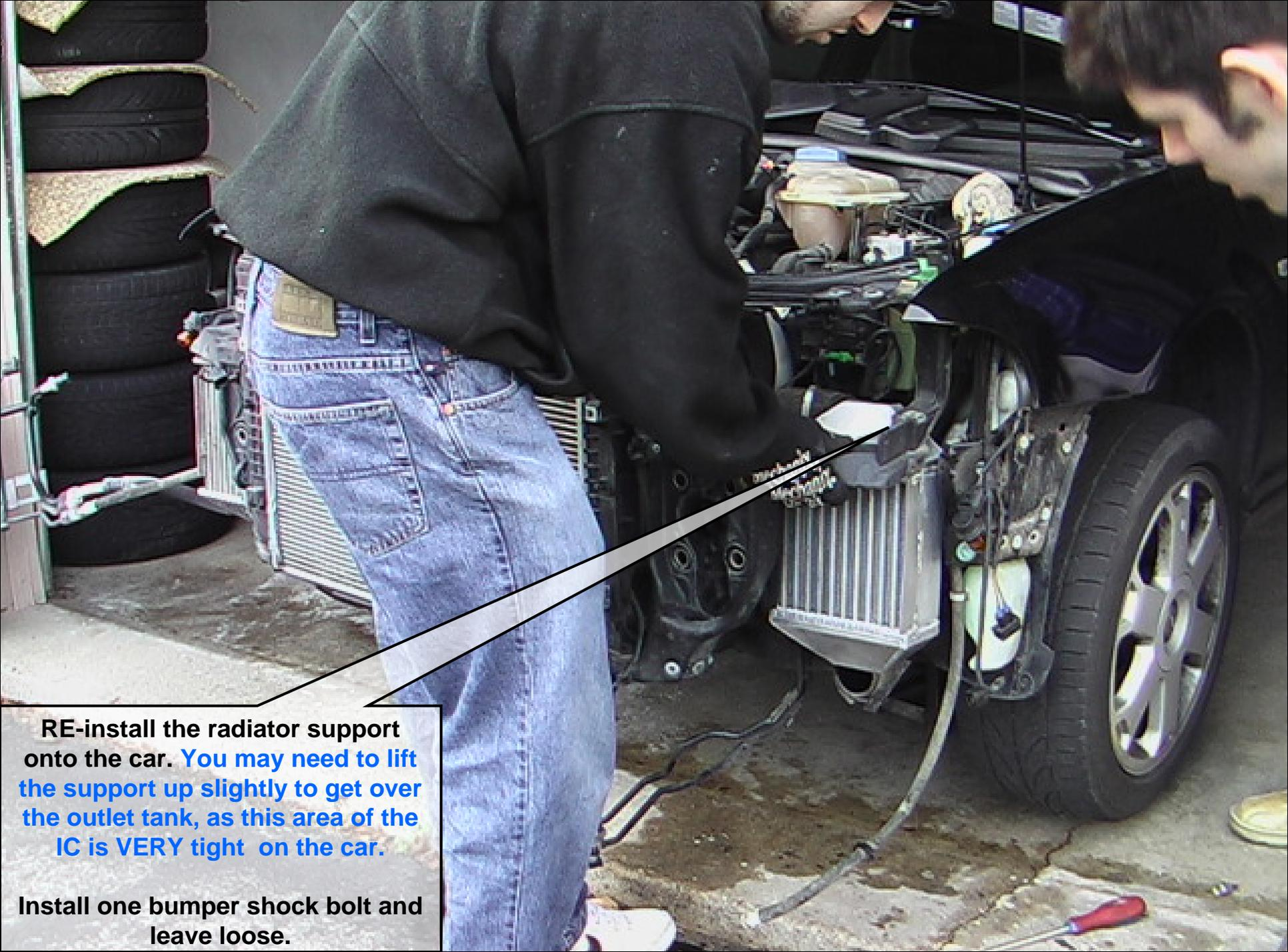
**RE-install the radiator support onto the car. You may need to lift the support up slightly to get over the outlet tank, as this area of the IC is VERY tight on the car.**
