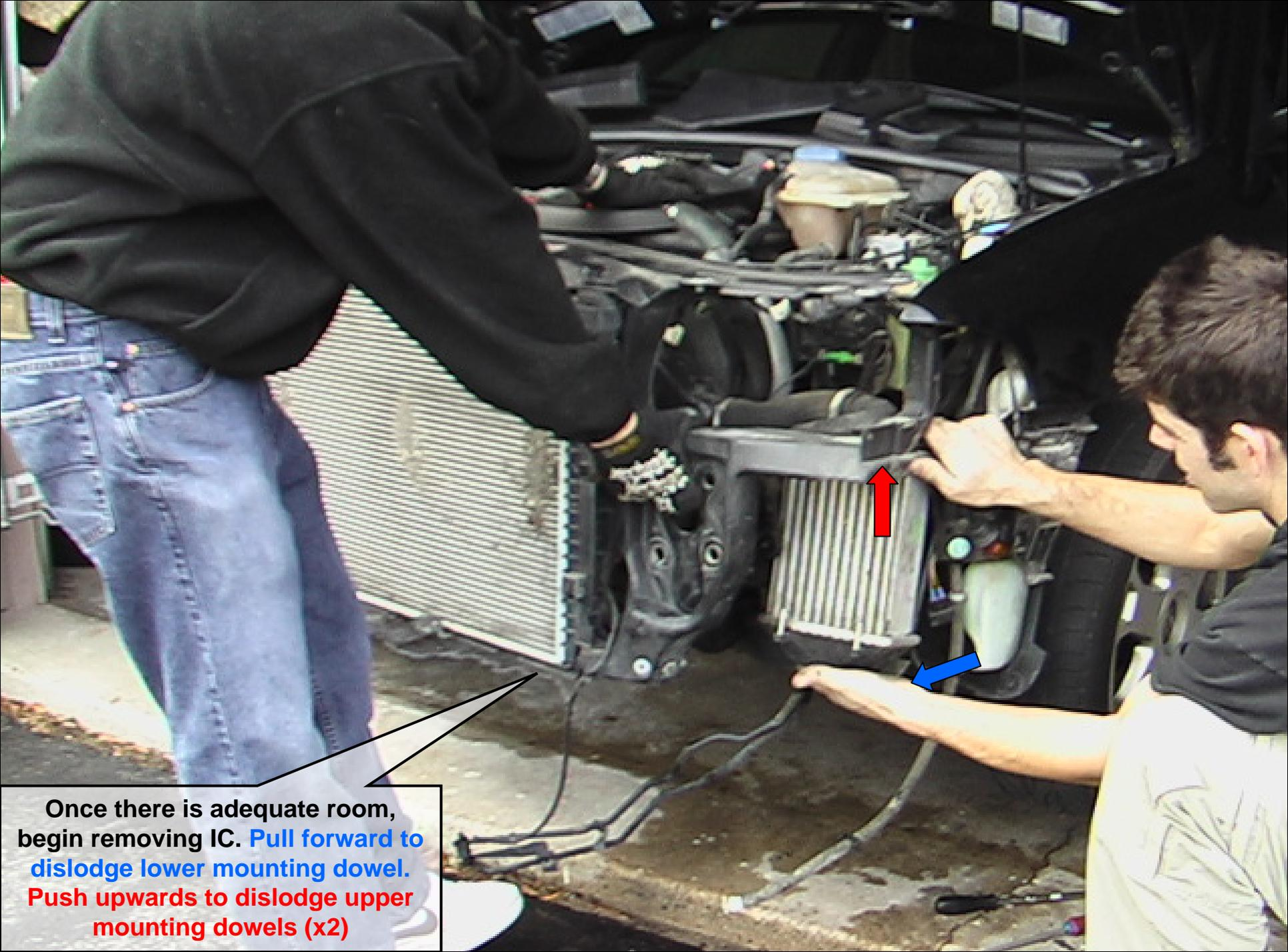
Once there is adequate room, begin removing IC. Pull forward to dislodge lower mounting dowel. Push upwards to dislodge upper mounting dowels (x2)
