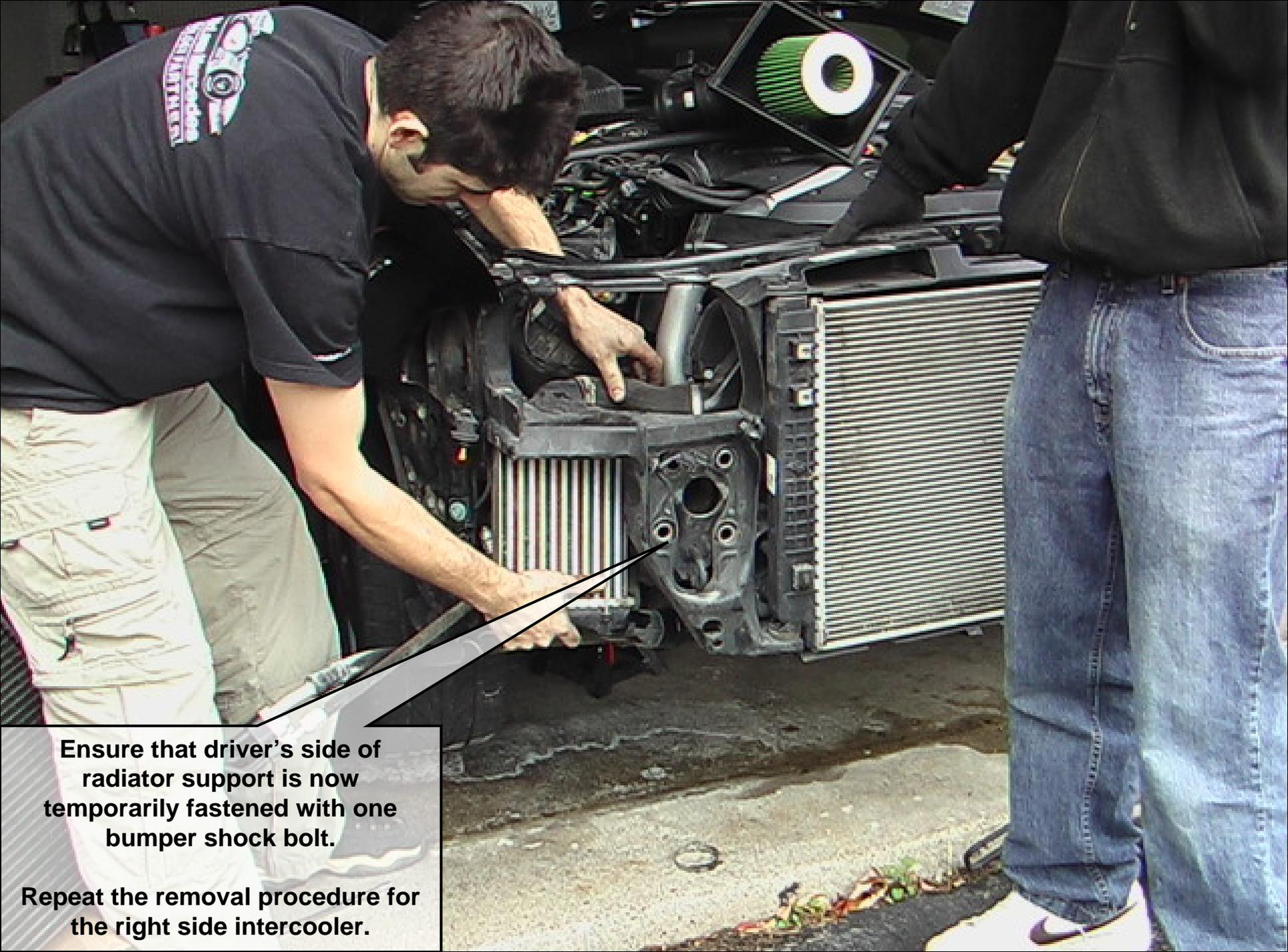
**Ensure that driver's side of radiator support is now temporarily fastened with one bumper shock bolt.**
