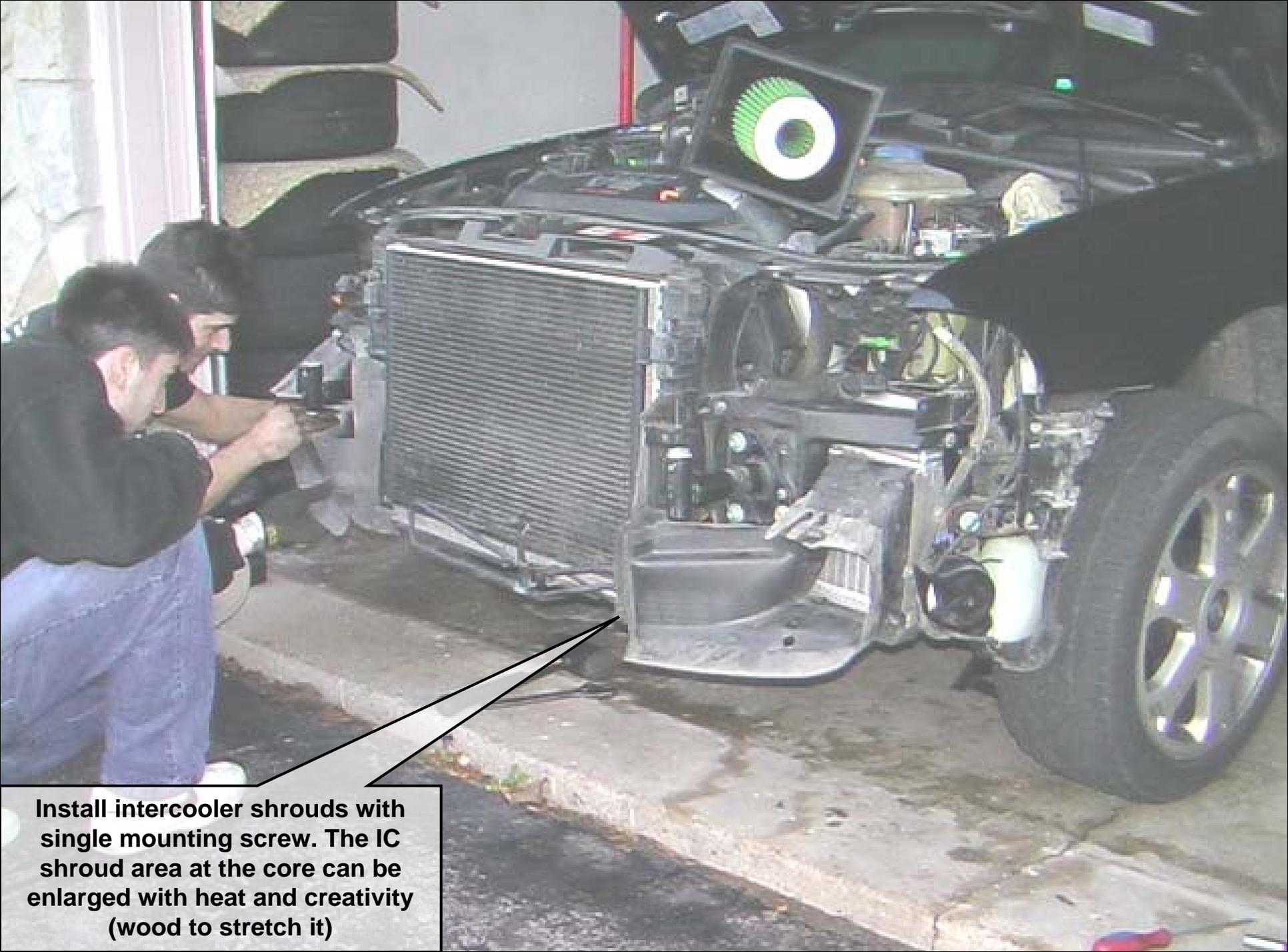
**Install intercooler shrouds with single mounting screw. The IC shroud area at the core can be enlarged with heat and creativity (wood to stretch it)**
