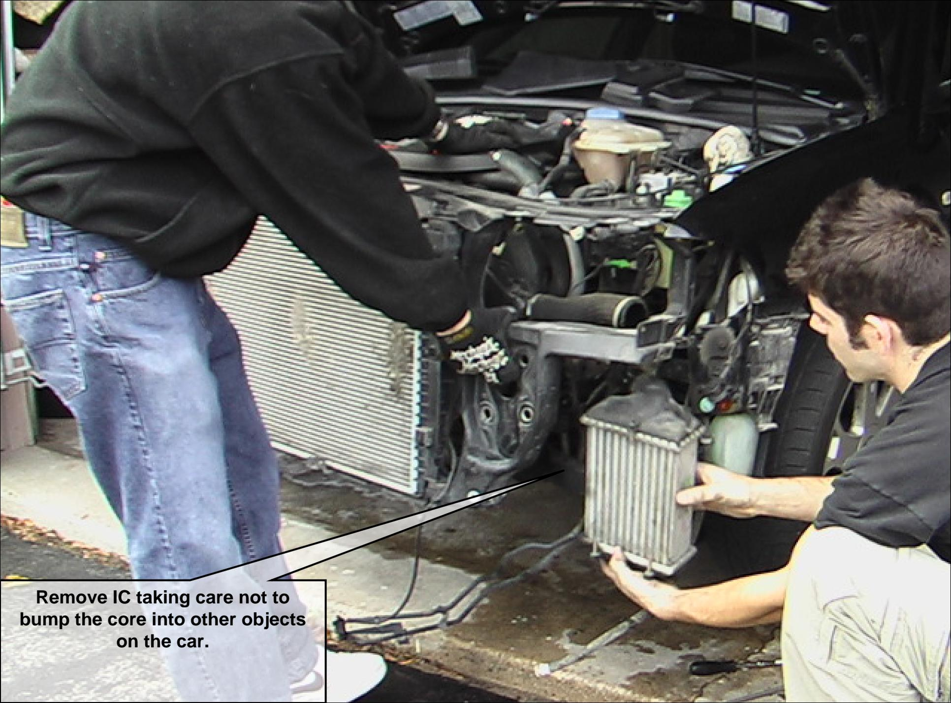
**Remove IC taking care not to bump the core into other objects on the car.**
