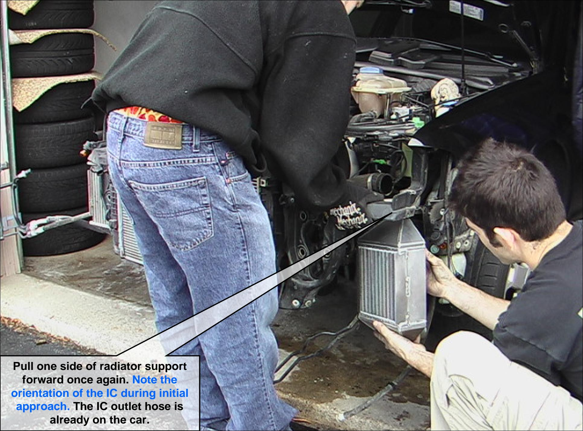
Pull one side of radiator support forward once again. **Note the orientation of the IC during initial approach.** The IC outlet hose is already on the car.
