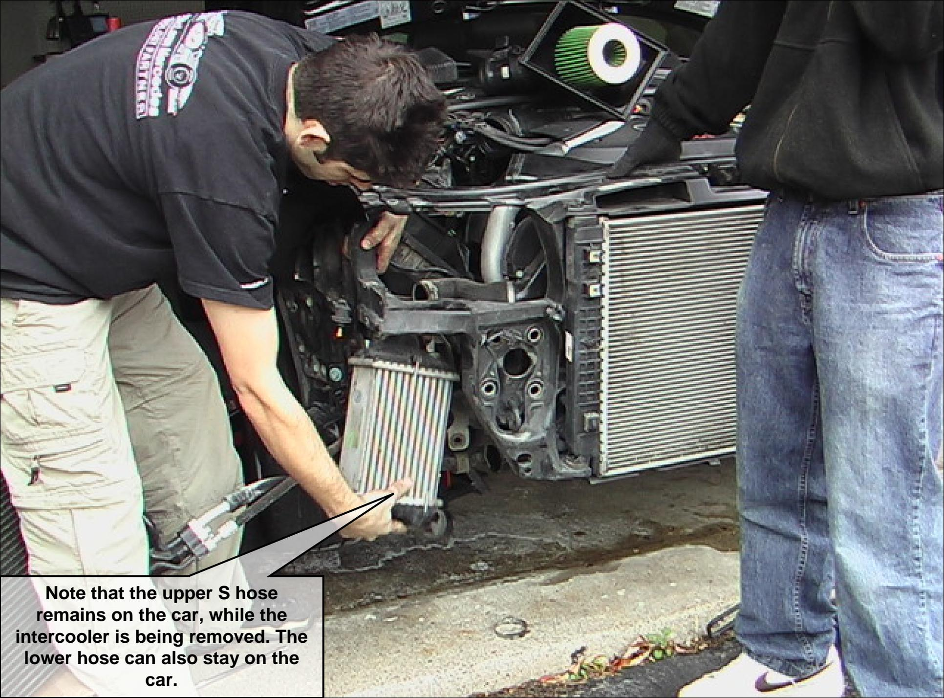
**Note that the upper S hose remains on the car, while the intercooler is being removed. The lower hose can also stay on the car.**
