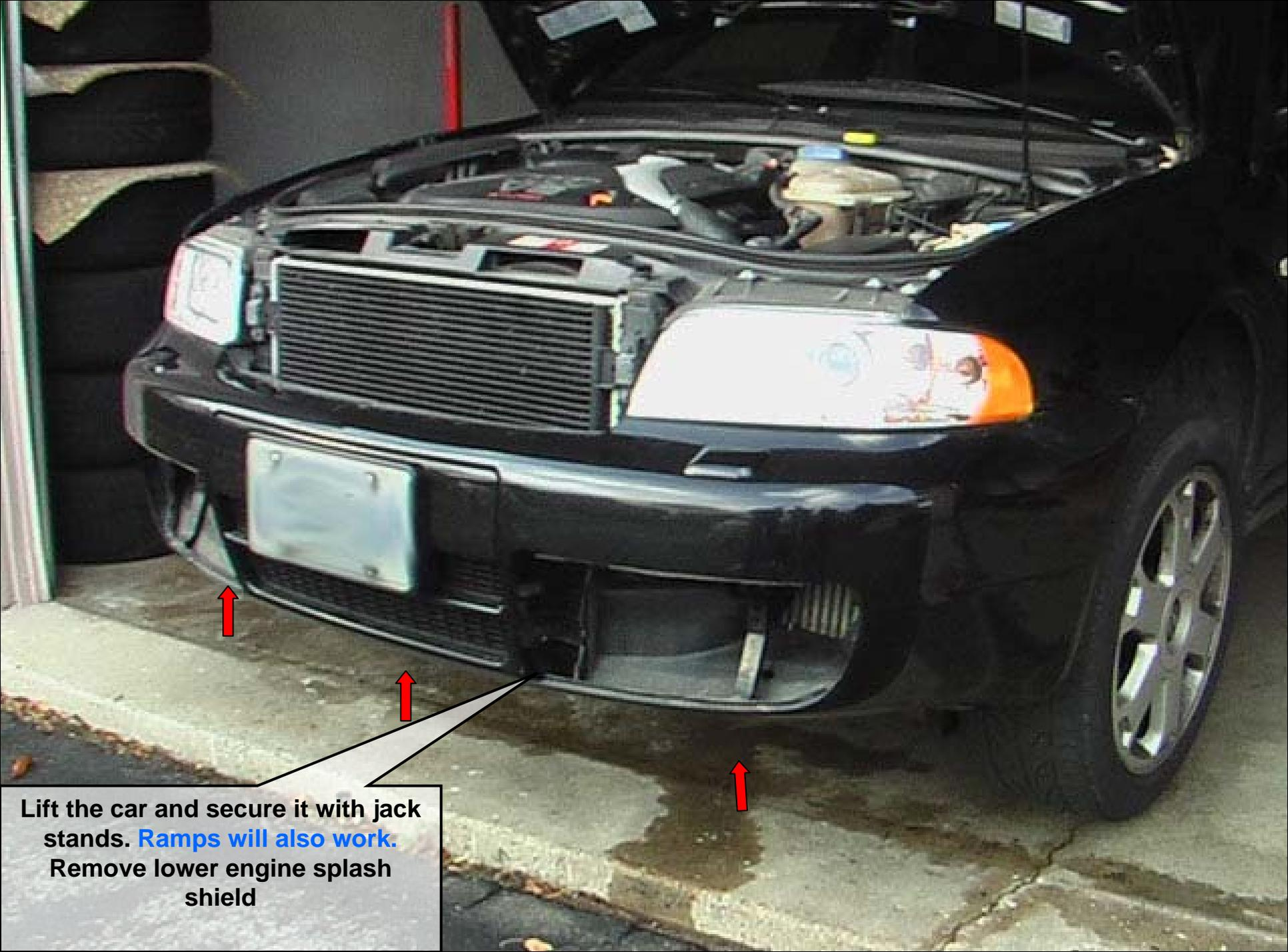
Lift the car and secure it with jack stands. Ramps will also work. Remove lower engine splash shield
