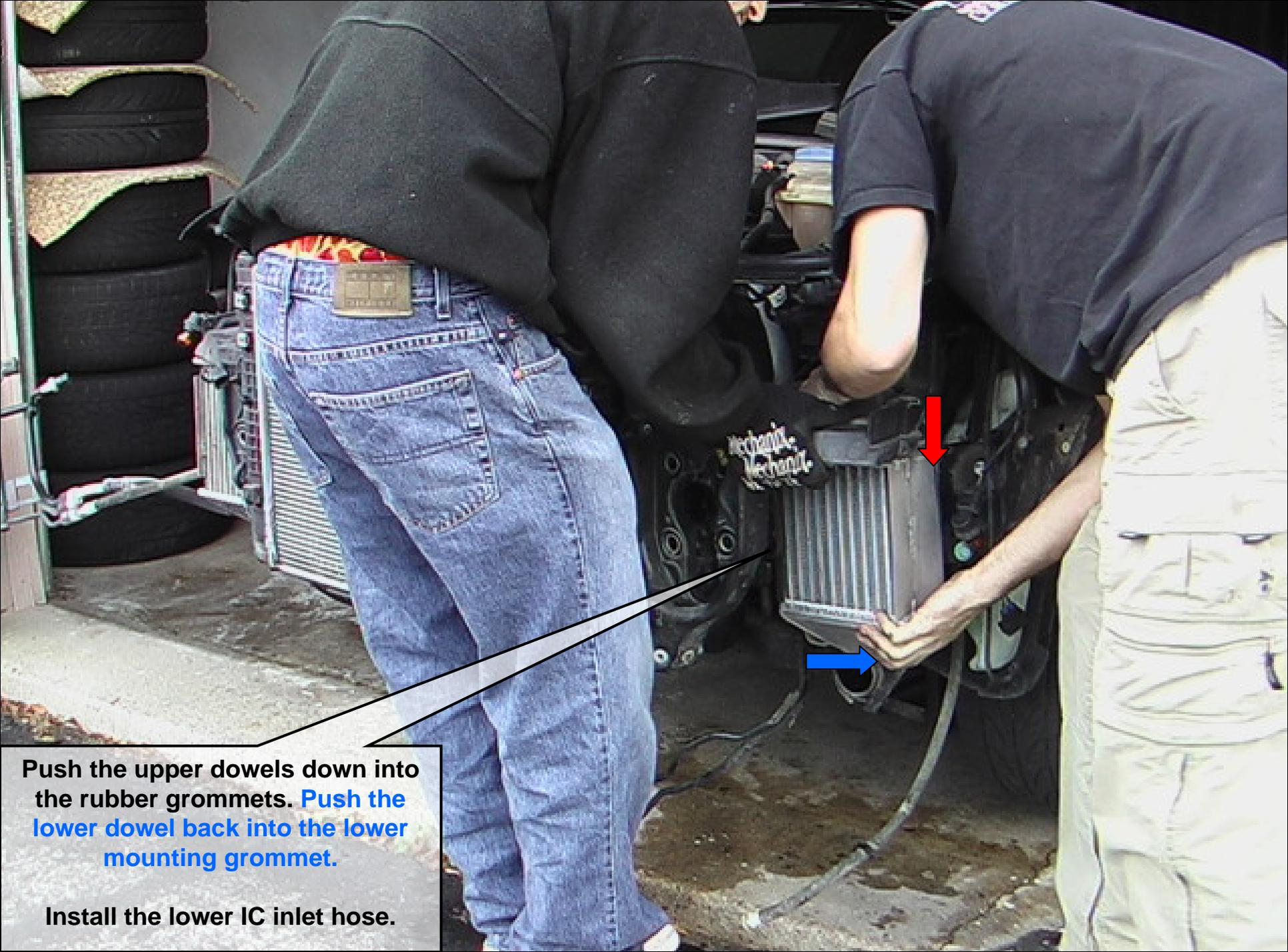
Push the upper dowels down into the rubber grommets. Push the lower dowel back into the lower mounting grommet.
