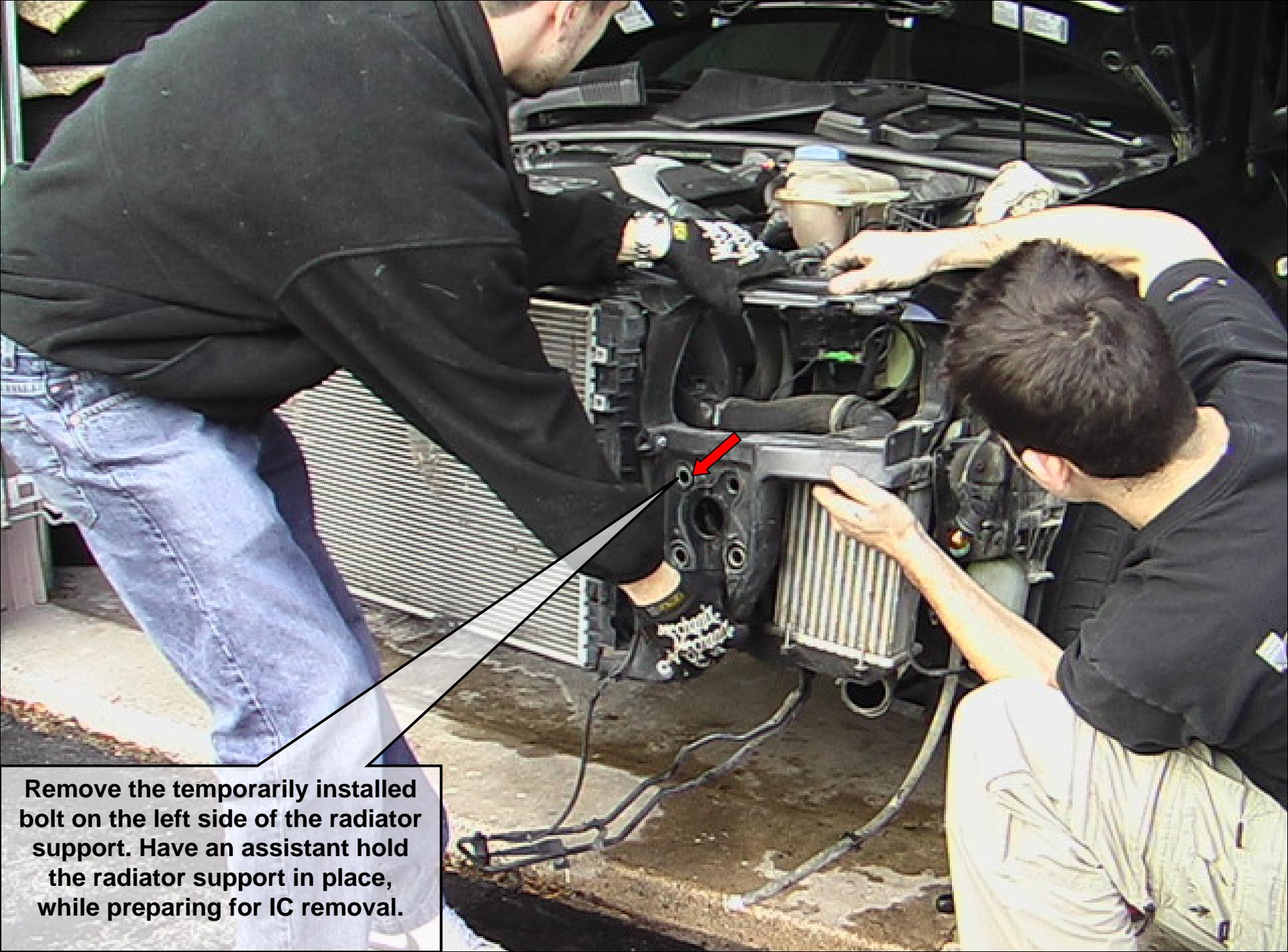
**Remove the temporarily installed bolt on the left side of the radiator support. Have an assistant hold the radiator support in place, while preparing for IC removal.**
