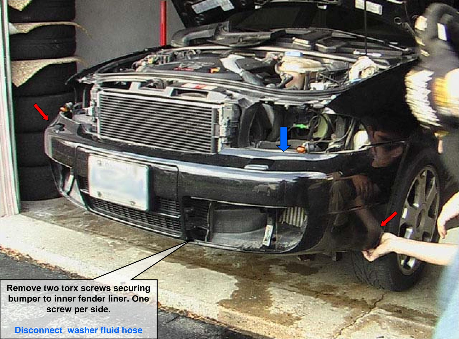
Remove two torx screws securing bumper to inner fender liner. One screw per side.
