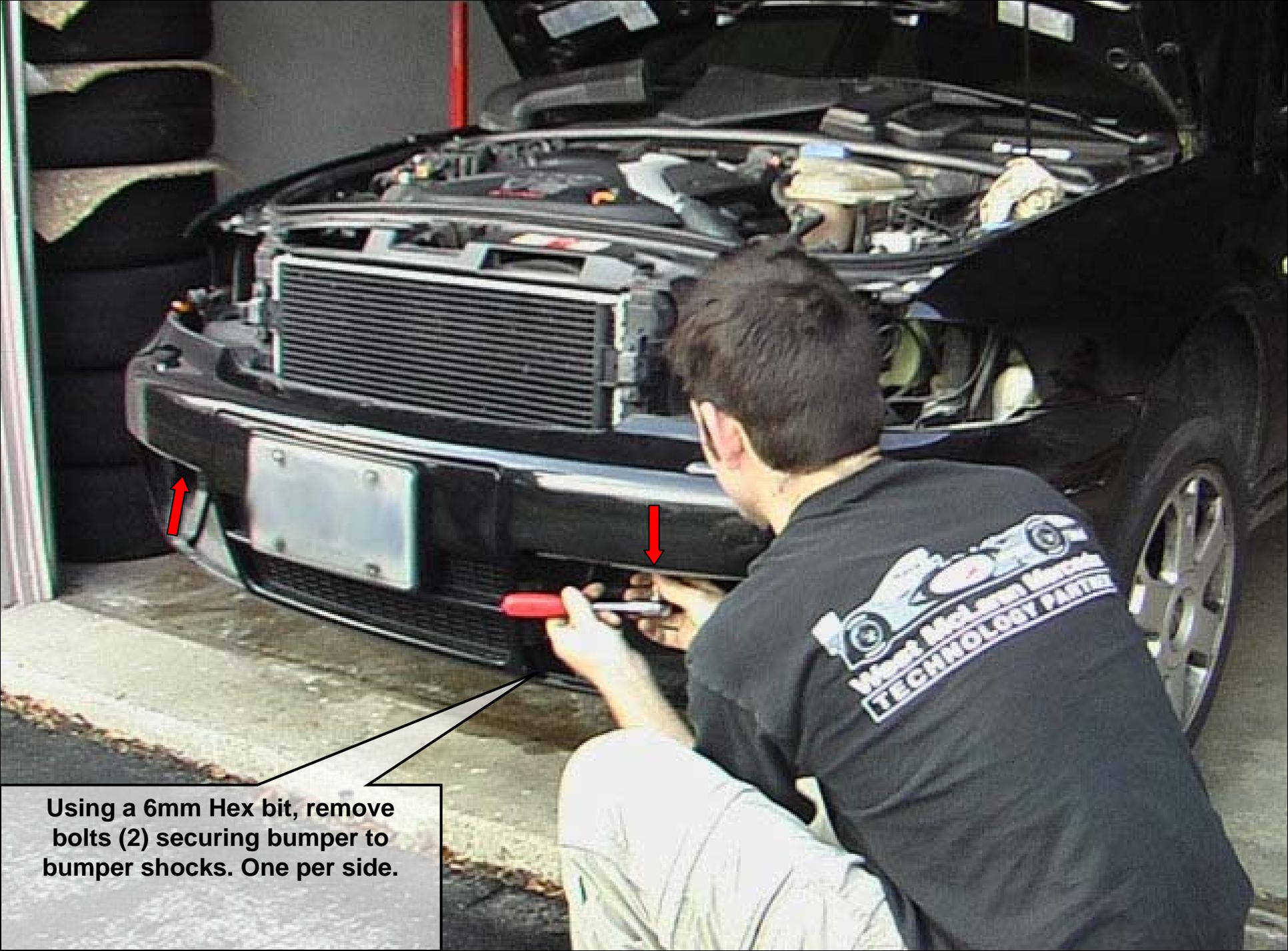
Using a 6mm Hex bit, remove bolts (2) securing bumper to bumper shocks. One per side.
