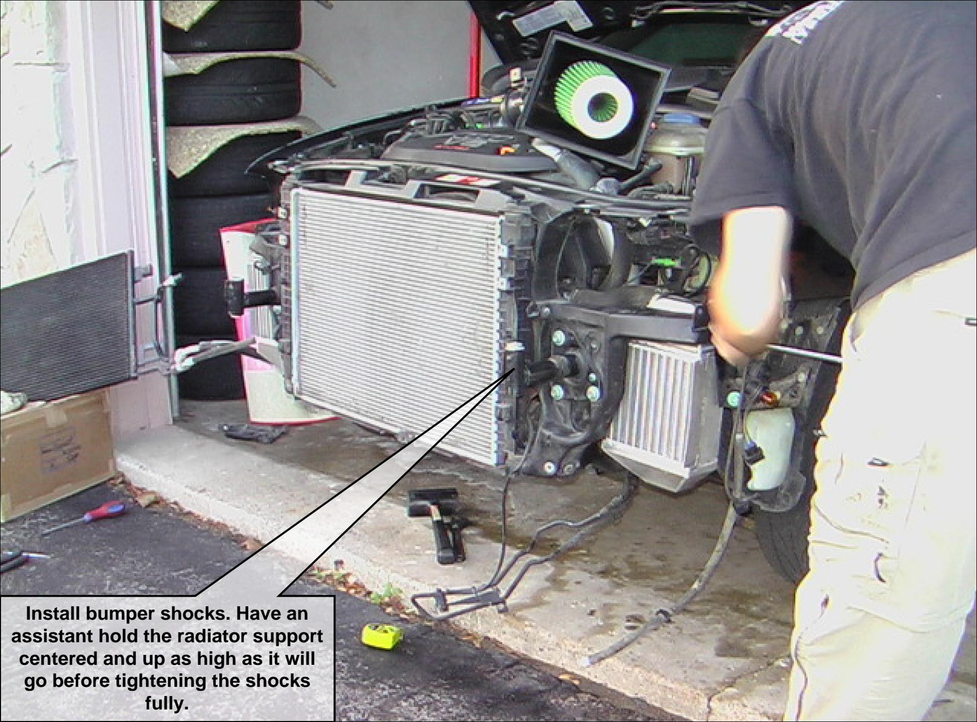
**Install bumper shocks. Have an assistant hold the radiator support centered and up as high as it will go before tightening the shocks fully.**
