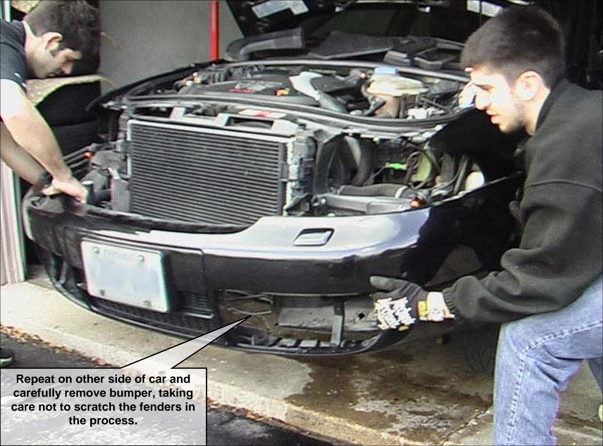
**Repeat on other side of car and carefully remove bumper, taking care not to scratch the fenders in the process.**
