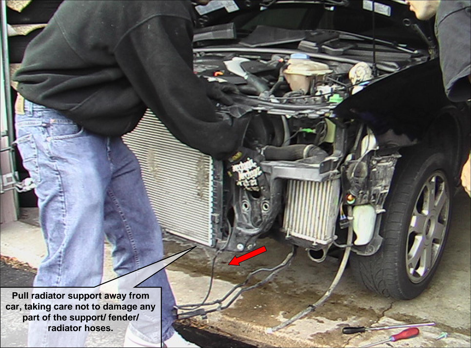
**Pull radiator support away from car, taking care not to damage any part of the support/ fender/ radiator hoses.**
