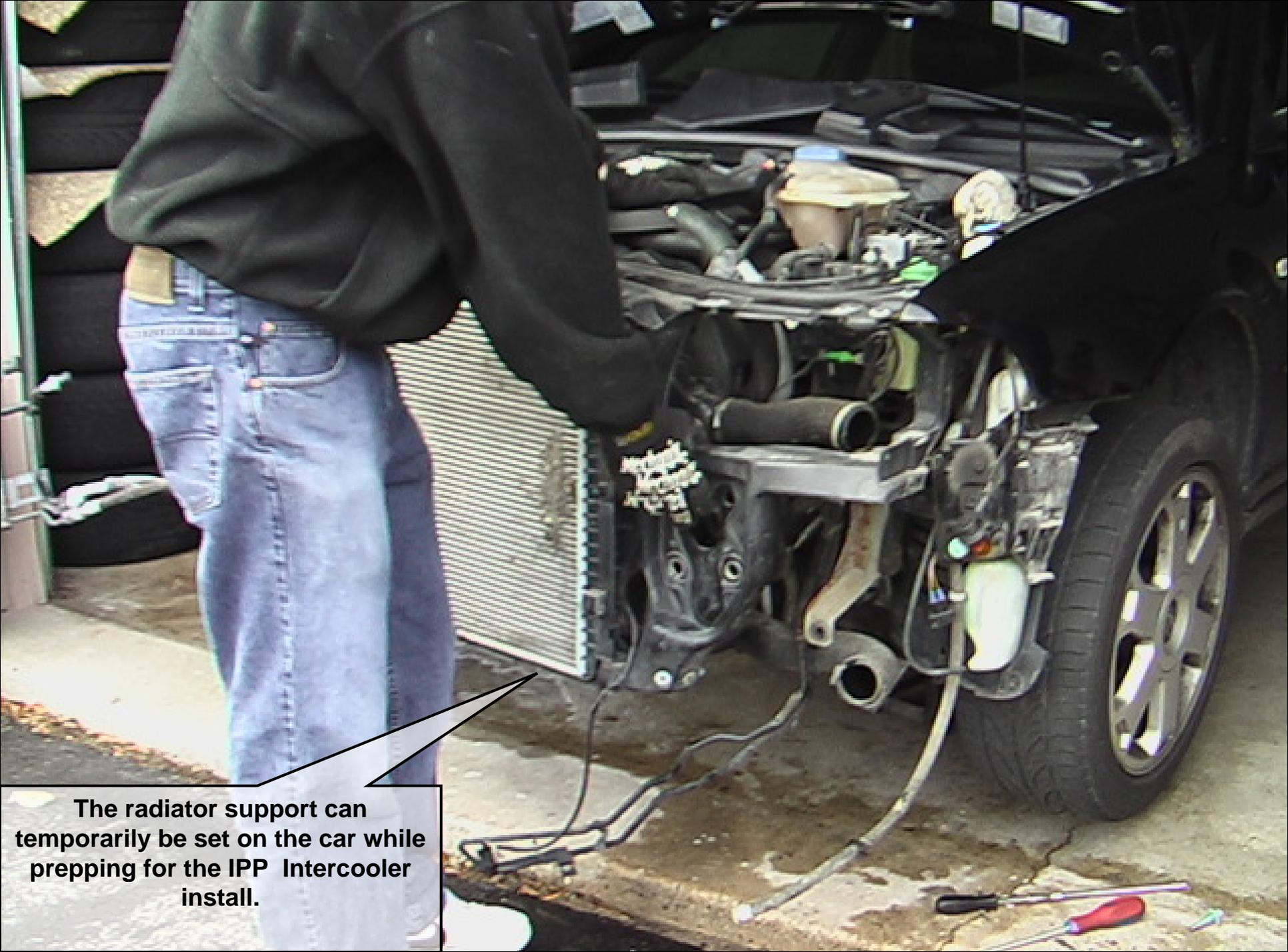
**The radiator support can temporarily be set on the car while prepping for the IPP Intercooler install.**
