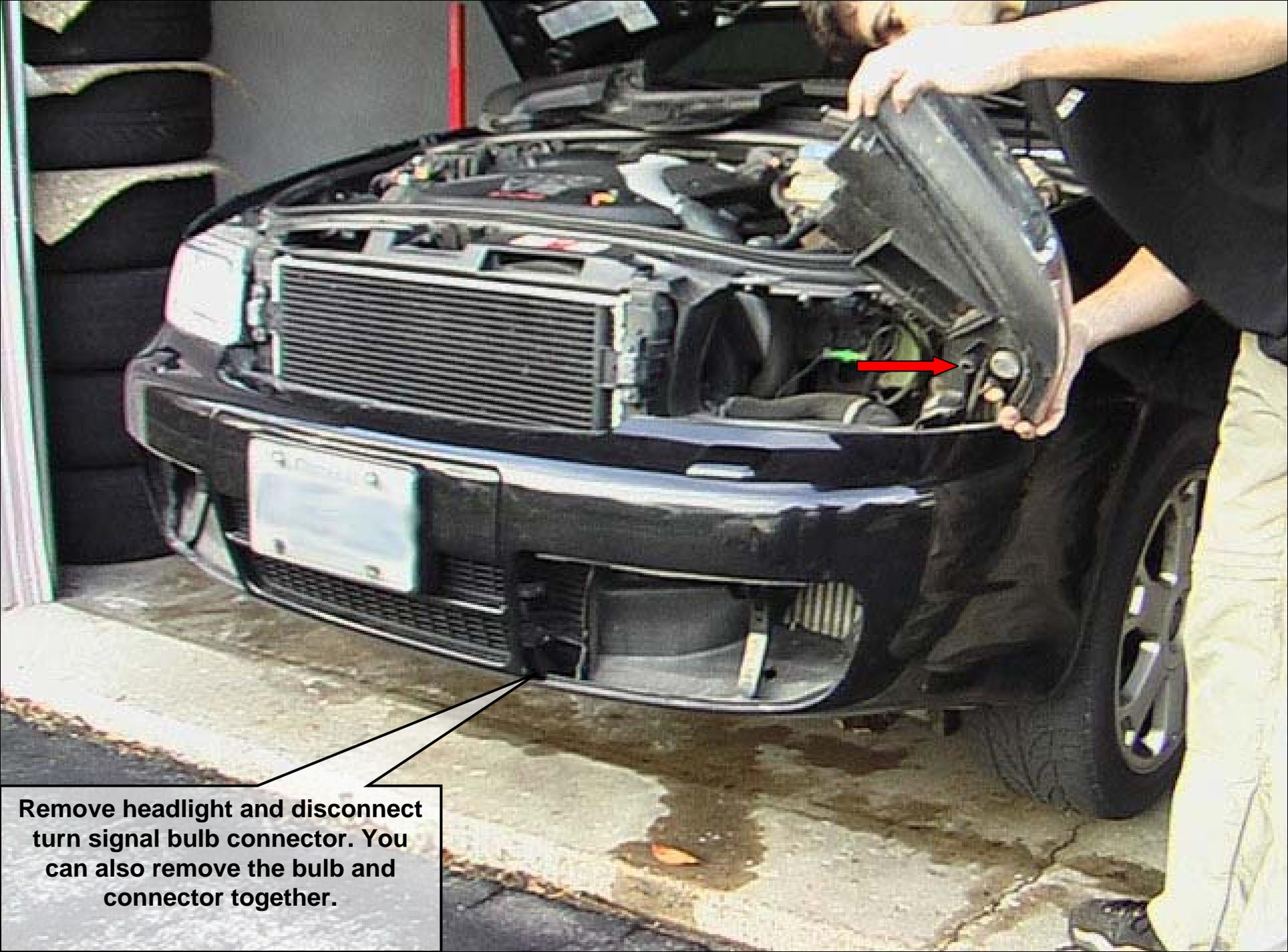
**Remove headlight and disconnect turn signal bulb connector. You can also remove the bulb and connector together.**
