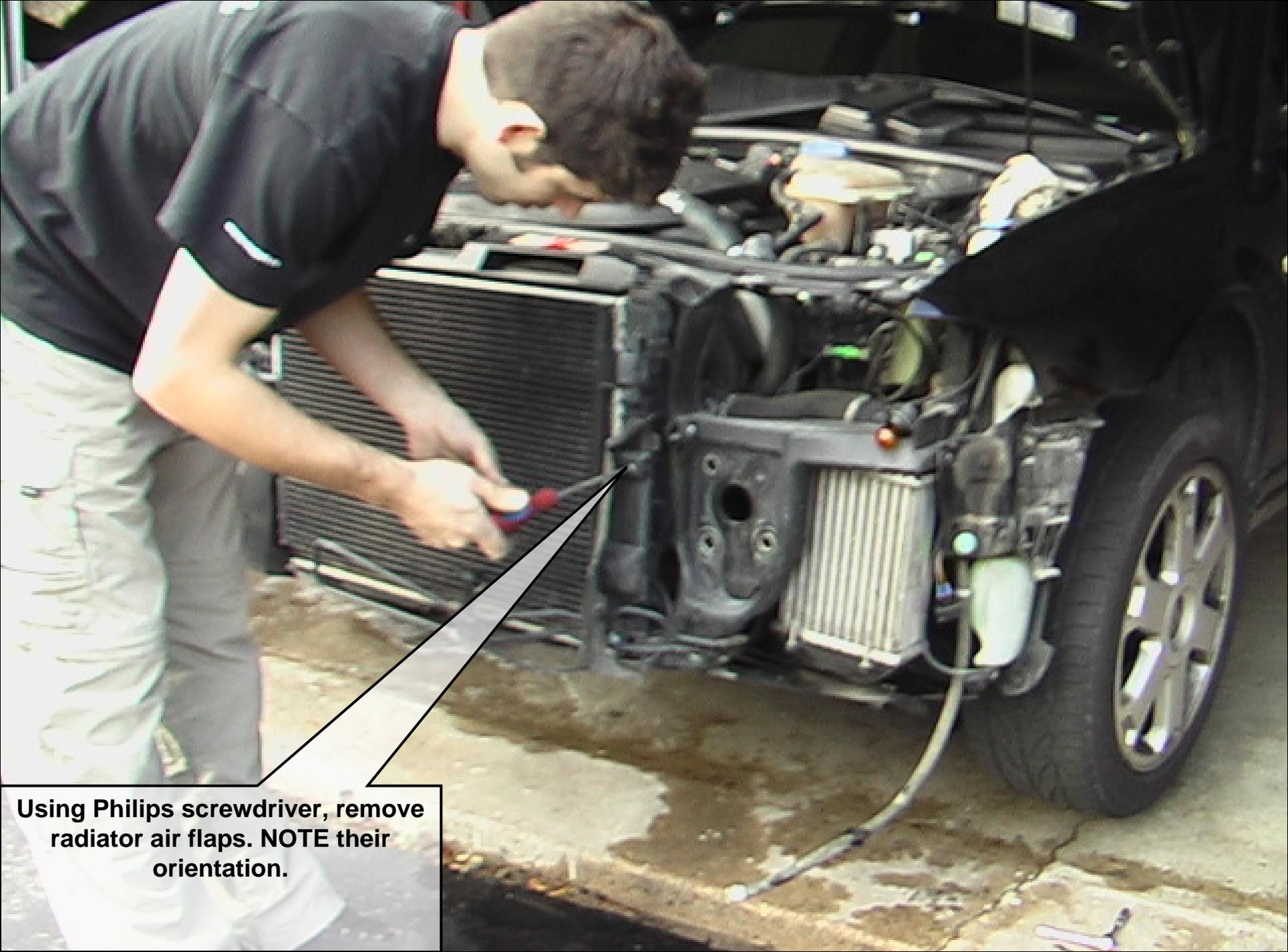
**Using Philips screwdriver, remove radiator air flaps. NOTE their orientation.**
