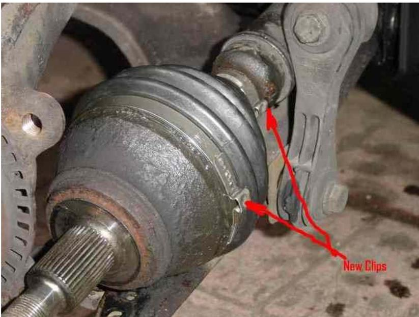
Push the gear box end of the gaiter onto it's seat.
