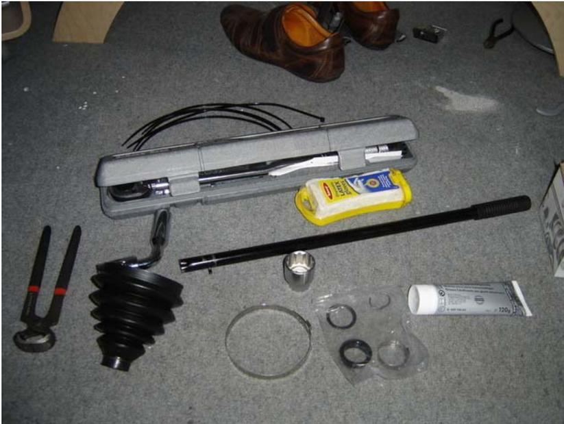
With the wheel still on the ground loosen the hub nut with the 30mm twelve point socket.
