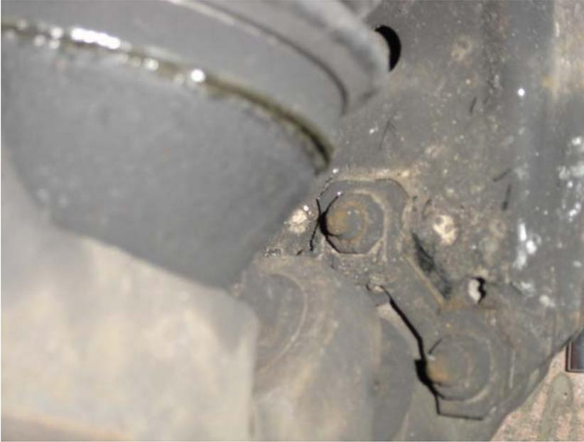
Undo the three bolts holding the lower ball joint to the hub using a 13mm socket.
