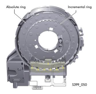
The basic components of the steering angle sender are:
