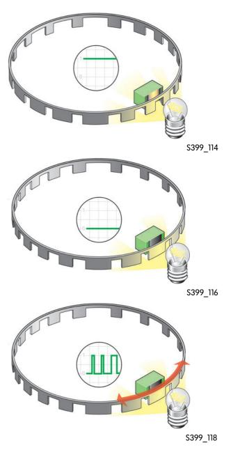
By comparing the signals, the system can calculate how far the rings have been moved. The starting point of the movement is determined by the absolute ring part.
