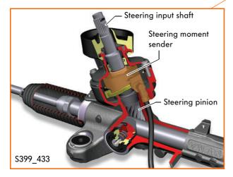
The steering moment applied to the steering wheel by the driver is the basis for calculating the assistance power that is provided by the steering system. The steering moment is measured at the steering pinion with the aid of the steering moment sender G269. The relative rotation of the steering input shaft is compared with the steering pinion and converted to an analogue electrical output signal.
