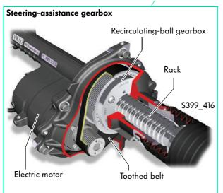
The electromechanical power steering with parallelaxis drive applies the necessary steering force to the rack using the steering-assistance gearbox. The steering-assistance gearbox consists of the electromechanical power steering motor V187, the recirculating-ball gearbox and the power steering control unit J500.
