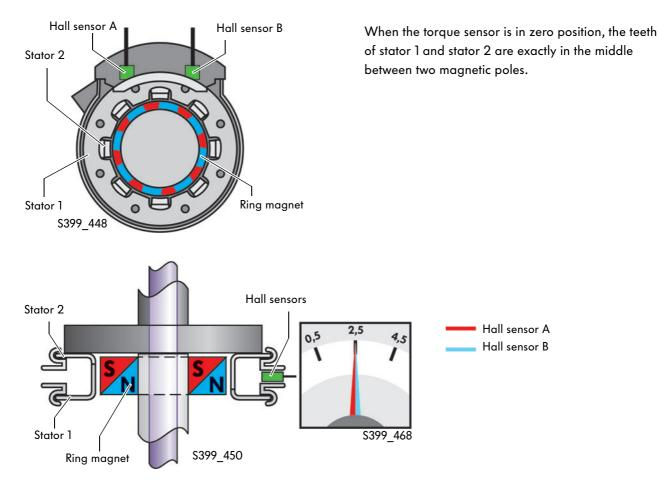
Therefore neither stator 1 nor stator 2 has a north or south alignment. A magnetic field cannot form between the two stators. The Hall sensors are supplied with an input voltage of 5V. As no magnetic field has formed between the two stators, the Hall sensors issue a signal for the zero moment of 2.5V.
