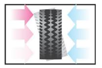
The straight-ahead driving correction provides steering assistance to relieve the driver on straight roads when there are constant cross-winds or the road has excessive camber. The different lengths of the drive shafts for the lefthand and right-hand front wheels resulting from the front-wheel drive and transverse engine layout often cause the vehicle to be pulled to one side while accelerating. The uneven tracking compensation system recognises this and counteracts it by countersteering.
