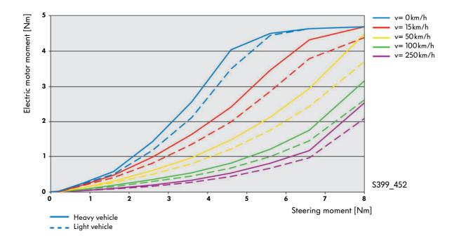
A map for a heavy vehicle (continuous line) and map for a light vehicle (broken line) for the Tiguan have been chosen as examples from the 5 maps available.
