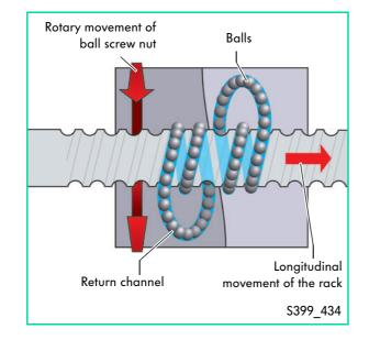
The ball screw nut is turned clockwise. The rack moves to the right.
