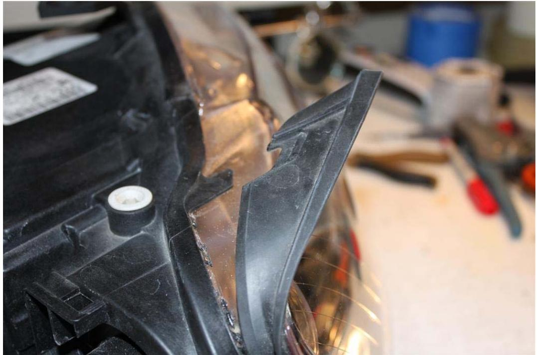
Install the headlight on a soft rag (prevent scratching the lens) and you are going to heat up the seal between the housing and the lens. No need to heat the entire perimeter, the glue used is messy enough when soft and you don't want it to stick to the chrome. Heat the area for 10 mn.
