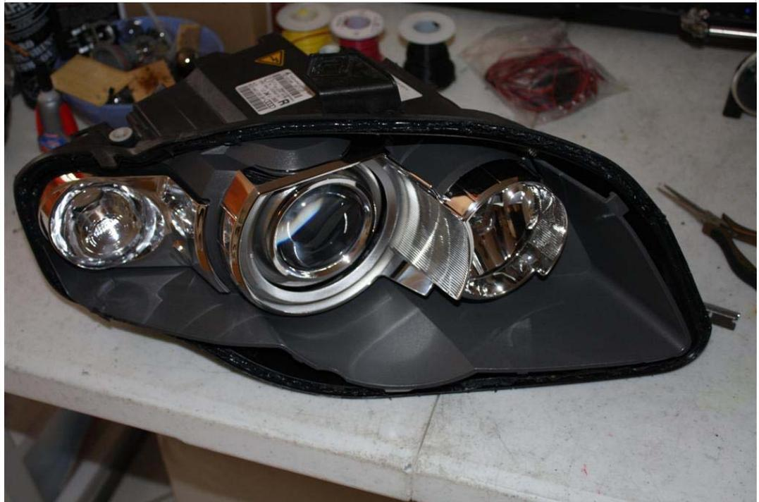
Now you need to remove the internal housing. There are 3 screws holding it in place. Location materialized in red
