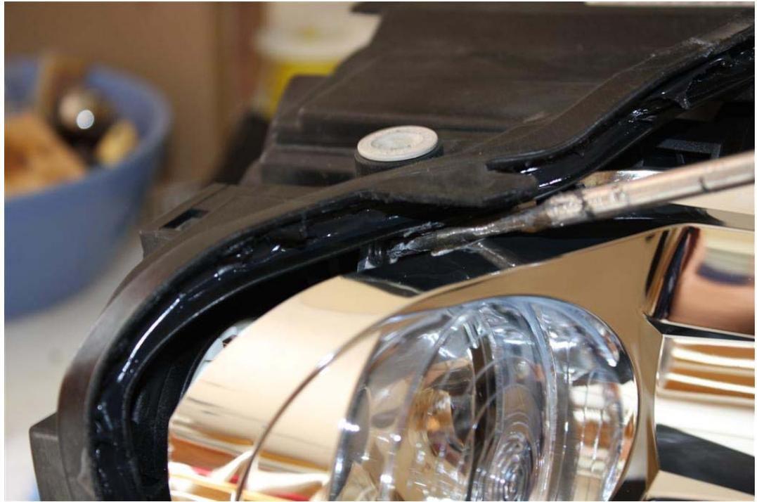
Now, you are going to separate the two plastic parts of the turn signal. Take a close look at the little plastic shaft preventing the separation
