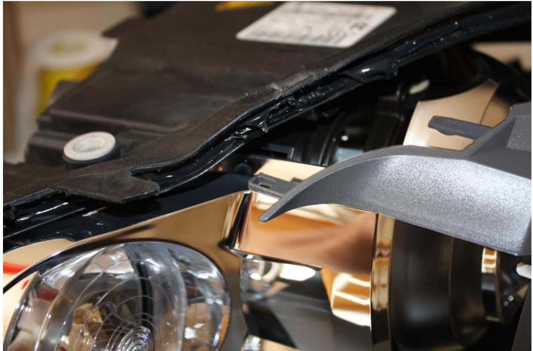
Once the housing is removed, there is an additional screw to be removed right under the turn signal.
