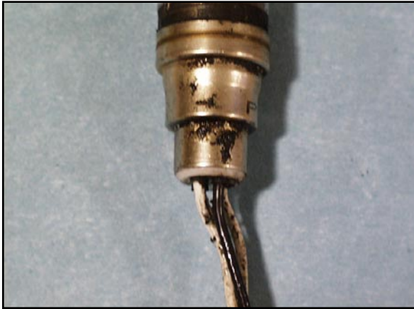
External Oil Contamination
