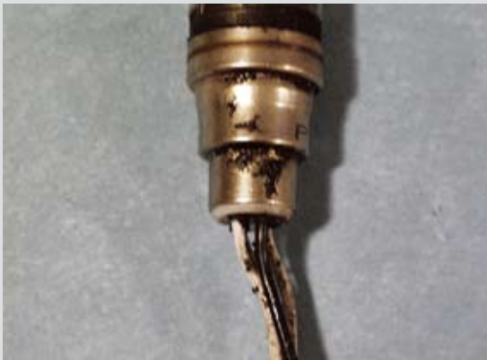
External Oil Contamination
