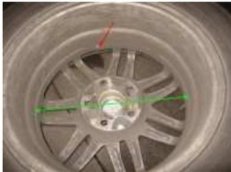
Well, in my case the problem persists removing metal grinder with calipers in these locations. The clearance was received with reserve, three millimeters.
