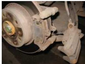
4. Unscrew hexagon 8 caliper mounting bolts to the hub, remove the caliper.
