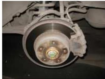
2. Old brake disc is usually due to wear a collar that prevents remove the caliper assembly with pads, so it's easier to remove the caliper frame by unscrewing the two screws.
