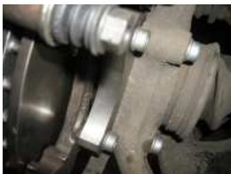
6. Look, that there was a gap between the brake disc and caliper frame.
