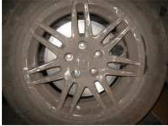
If you install winter tires still found that the caliper touches the disk due to the larger offset. I had to put a spacer made of metal, of a thickness of 10 mm.
