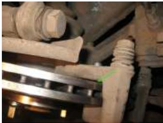
7. Install the new pads, fasten the caliper to the frame. To down piston calipers, you need to rotate around its axis while pressing on it.
