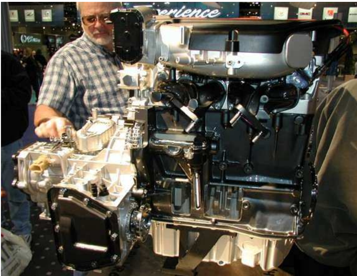
cutaway photos of the latest 12v VR6 from a car show
