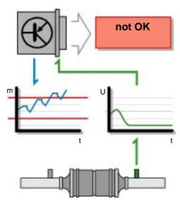
In this case too, the post-catalytic converter probe detects an oxygen increase in the exhaust emissions through a drop in voltage and indicates this to the engine control unit.
