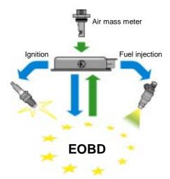
The air mass meter G70 takes over the task of determining the intake air quantity. For this reason, the induction pipe pressure sensor G71 is not necessary.
