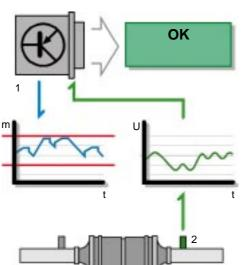
Lean fuel-air mixture and correct The post-catalytic converter probe detects an oxygen increase in the exhaust emissions through a drop in voltage and indicates this to the engine control unit.
