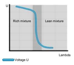
A planar lambda probe (LSF) is used for the post-catalytic converter probe.
