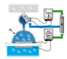
The fuel-air mixture becomes leaner. This means that the oxygen concentration in the exhaust increases and that the pump cell pumps more oxygen into the measuring area than can escape through the diffusion channel. This changes the oxygen ratio in respect of the external air and the voltage between the electrodes drops.
