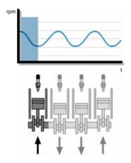
During the compression, the engine's movement energy is used to compress the fuel-air mixture. The engine's speed decreases.
