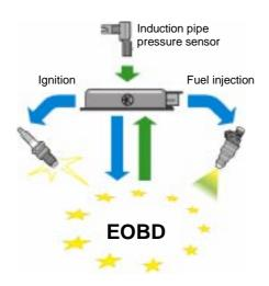
The intake air quantity is determined by the induction pipe G71 sensor for these engine management systems.
