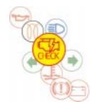
If an error should occur in the vehicle which impairs the emissions quality, the error is stored in the fault memory and the exhaust gas indicator light is turned on.
