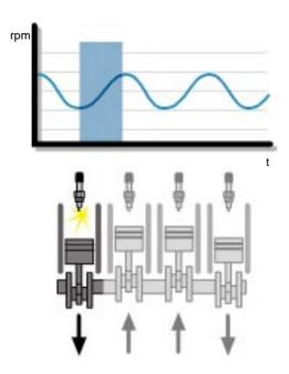
Ignition occurs after compression and the engine speed will be accelerated. In this manner, the engine speed fluctuates during each combustion due to compression and ignition.
