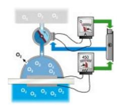
In order to re-establish the voltage of 450 mV between the electrodes, the oxygen content on the exhaust side must be reduced. The pump cell must then pump less oxygen into the measuring area. The pump performance is then reduced. The engine control unit converts the current consumption of the pump cell into a lambda value and changes the mixture composition accordingly.
