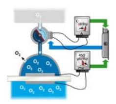
The pump cell must increase its capacity, so that the oxygen content increases in the external air chamber. The electrode voltage is reset to the value of 450 mV in the process and the current consumption of the pump is converted into a lambda control value by the engine control unit.
