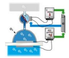
When the fuel-air mixture becomes too rich, the oxygen content in the exhaust decreases, the pump cell delivers less oxygen into the measuring area and the voltage of the electrodes increases. In this case, more oxygen escapes through the diffusion channel than the pump cell delivers.
