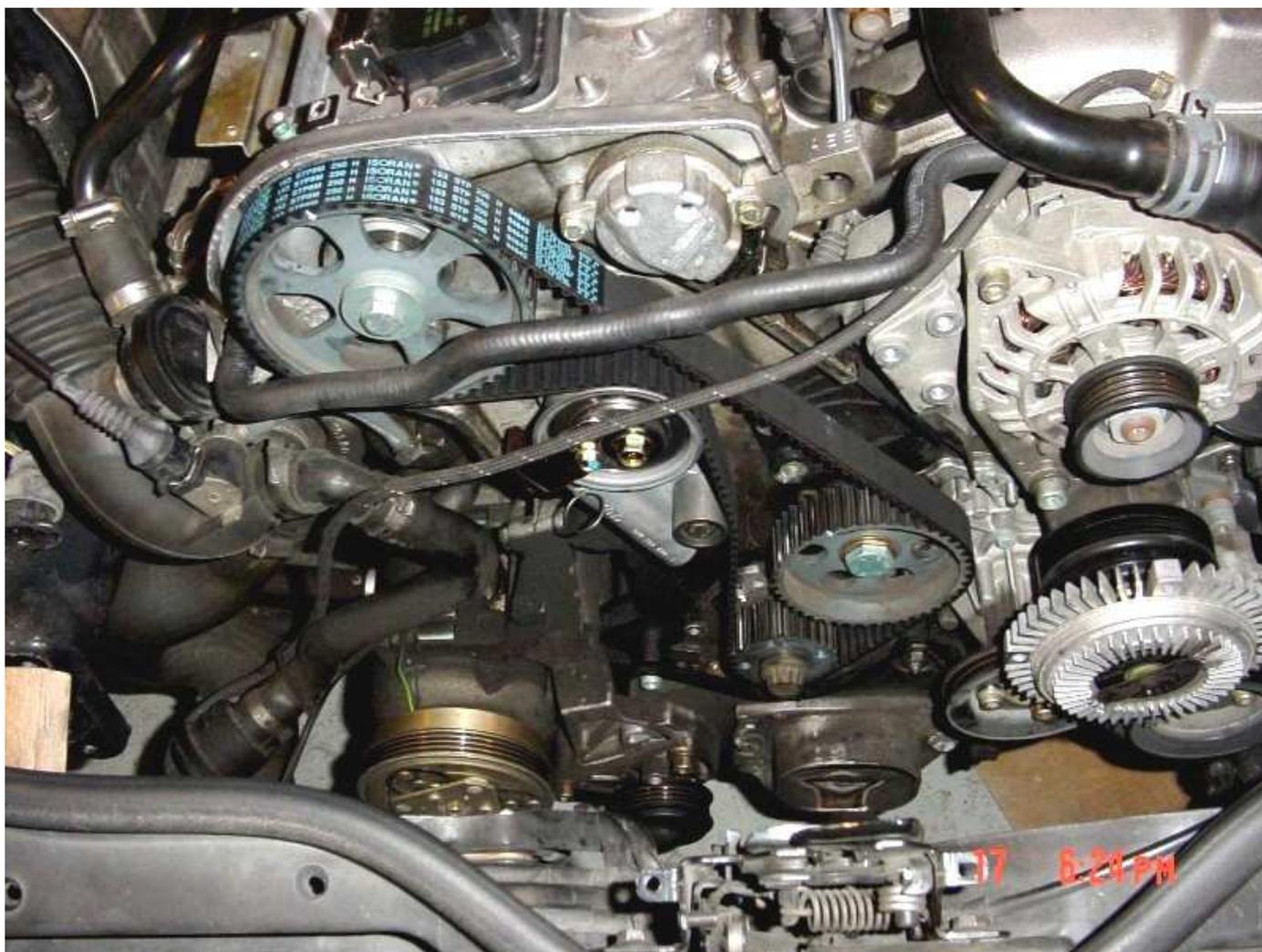
38. Now that all the timing components are assembled, take a moment to verify that the timing marks on the crankshaft sprocket and the camshaft sprocket line up correctly. If they do, you can "pull the pin" to engage the tensioner. (This is one of life's watershed moments, like getting the training wheels off your bike or cutting your child's umbilical cord, so take a moment to enjoy it!)
