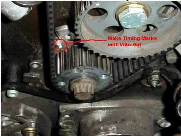
29. Visually inspect the crankshaft sprocket, camshaft sprocket and intermediate sprocket for damage or wear. Replacement of any of them is outside the scope of these instructions; you will need to refer to Chilton/Haynes for further instructions, and your dealer for the parts.
