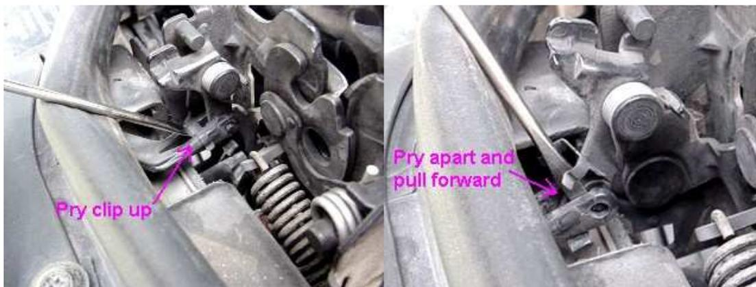
7. Front Bumper Cover: Remove the screws shown in the following photos:
