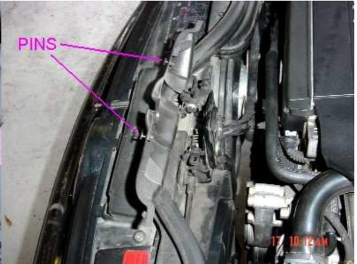
Using a small flat-blade screwdriver (or two), disconnect the plastic hood-release pull from the latch mechanism. It's a bit of a pain to get off, so be patient.
