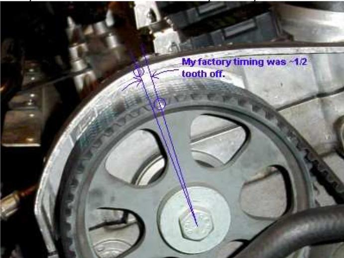
Update: A few other members have noted that on their engines the camshaft timing "leads" the crankshaft timing by about a half a tooth or so, especially after the new belt is installed. Apparently, this is part of the engine's design, so that if the belt stretches slightly over time, the timing will improve instead of getting worse.
