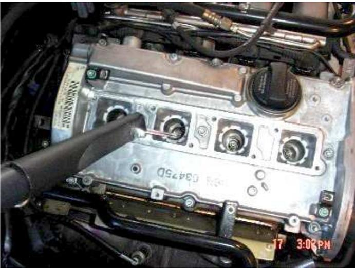
25. Using a large socket wrench or a breaker bar, slowly hand-turn the crankshaft pulley clockwise until the timing mark on the camshaft sprocket lines up with the mark on the front of the valve cover AND the timing mark on the crankshaft pulley lines up with the arrow on the lower timing belt cover. When they all line up, the engine is at TDC.
