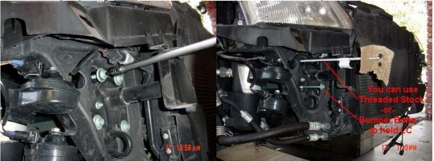
12. Unbolt the power steering oil cooler line and outside temperature sensor from the front of the LC. Also, remove the small retaining clip that secures the temp sensor's wire.
