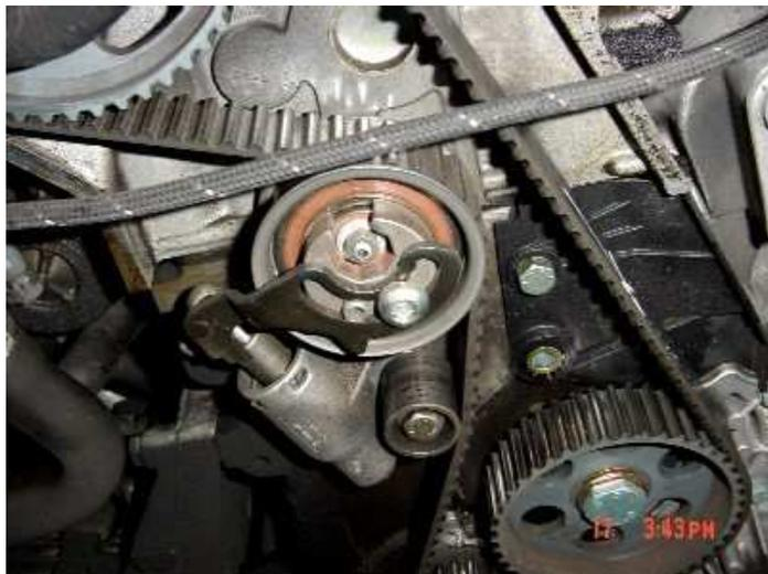
32. Remove the timing belt; try not to kink it or move either the camshaft sprocket or crankshaft sprocket. Visually inspect the belt for damage, uneven wear and contamination. Correct the causes of these conditions before proceeding.
