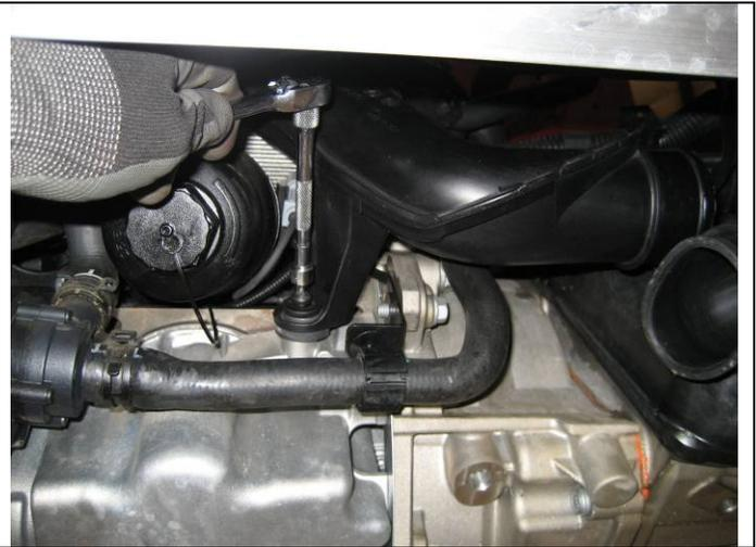
42 Remove the plastic charge pipe with throttle body boot from the vehicle.
