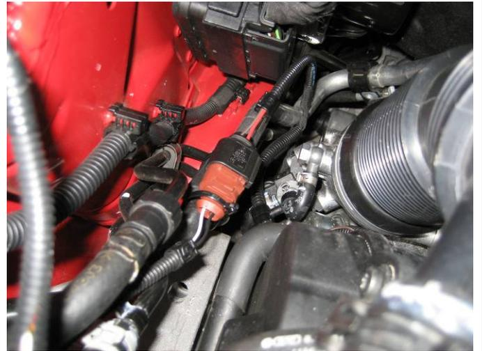
107 Install supplied hose for the Turbocharger Recirculation from the Recirculation Valve flange, under the A/C service hose, to the Turbocharger Inlet hose. Attach support clip to coolant service line above alternator. Install spring clamps at both ends of the hose.
