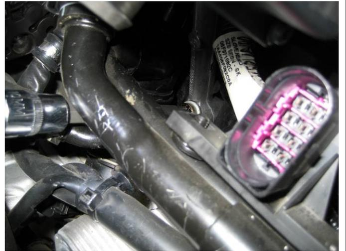
44 Disconnect electrical connector for Fuel Pressure Sensor G247. This is difficult to see and is below the intake manifold between cylinders 1 and 2.
