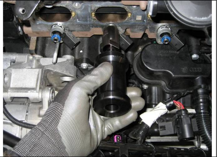
50 Using the pipe brush, clean out the fuel injector bores in the cylinder head to ensure a clean surface for the Teflon injector seal.
