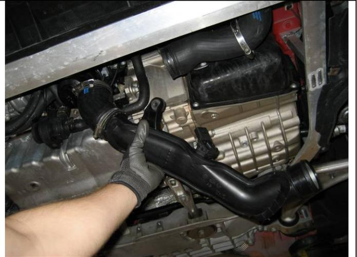
43 From above the vehicle, remove the M10 triple square bolt for the intake manifold support bracket to the engine. This bolt is difficult to see. The location is below the intake manifold and behind the throttle body. The electrical connector in the picture is for the fuel injectors from step 24. It's helpful to have a socket with a minimum shaft length of 4"
