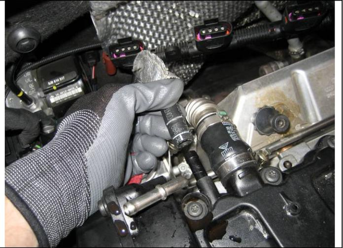
69 Loosen the two M6 bolts on the turbocharger inlet for the crankcase breather vent pipe
