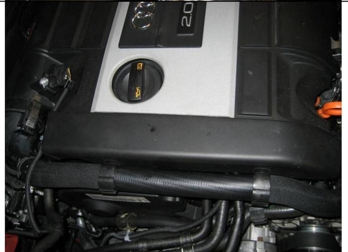
110 Add coolant/water mix to Coolant Reservoir until the system is full. Let the system degas and top off again.
