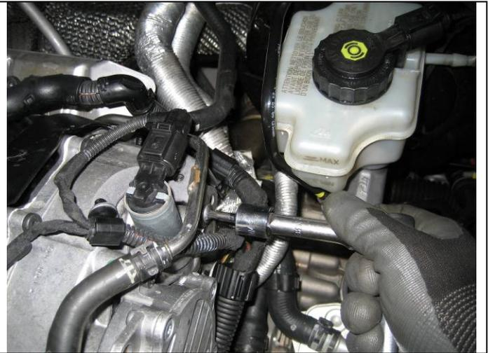
68 Disconnect the small crankcase ventilation vacuum line from the cylinder.
