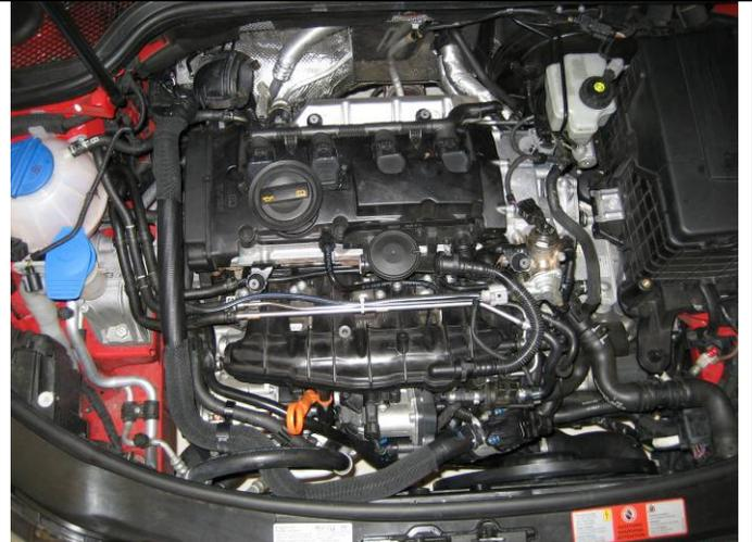
108 Drill two 0.242" (0.250 maximum) size holes in the Air Cleaner Assembly and install the support clips for the Turbocharger Recirculation hose. Measure from the rear corner, passenger side of the assembly (left side in the picture). Drill holes at 3 7/8" and 11 1/2" from corner and 1/2" up from the lower edge.
