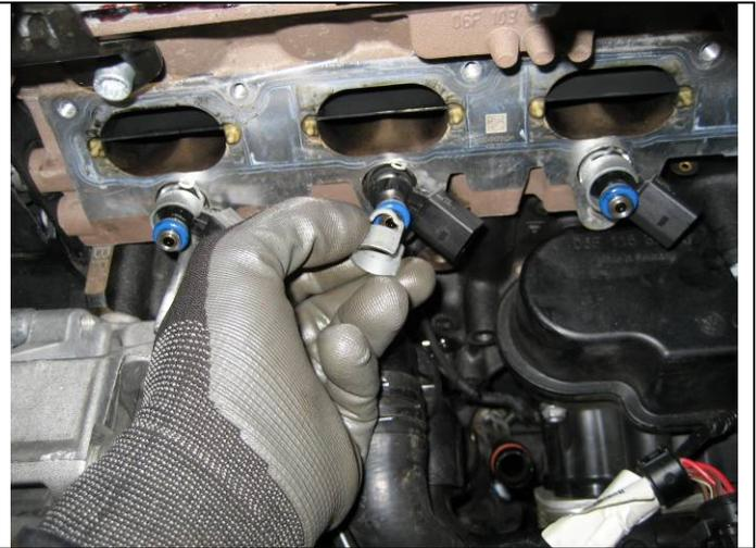
49c Using the slide hammer T10133/3 and puller T10133/2, guide the puller into the groove on the fuel injector, and slide hammer the injector out of the cylinder head.
