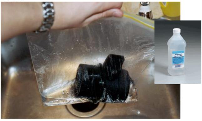
(5) Remove the MAF from the bag and let the alcohol drain off. I left mine overnight before reinstalling it in the car. It has to be COMPLETELY dry so rather be safe than sorry!
