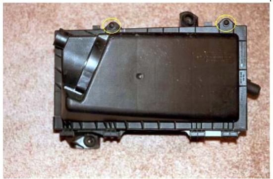
(2) Disconnect and remove MAF from air box lid – Two torx screws or Philips heads.
