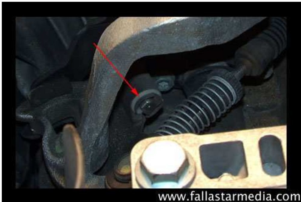
11. Locate the shifter weight retaining nut.
