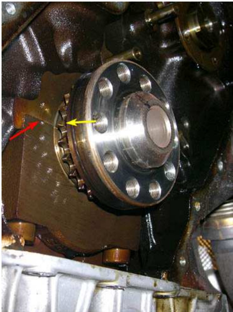
31. The picture below shows a close-up of the ground tooth (yellow arrow) and bearing split (red arrow). Note the difference between the ground tooth and the "normal" teeth adjacent to it (blue arrows).
