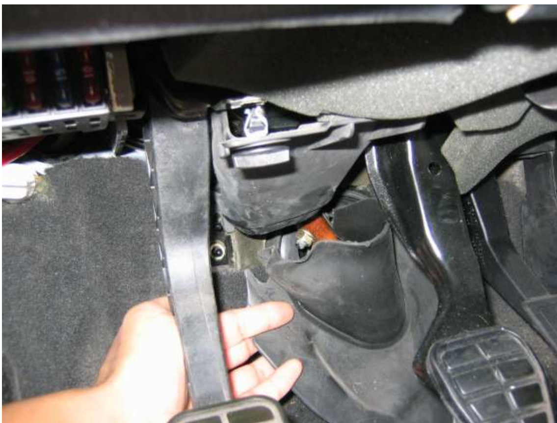
5) Remove the knee panel (remove the 5 screws at the bottom and pull straight down)
