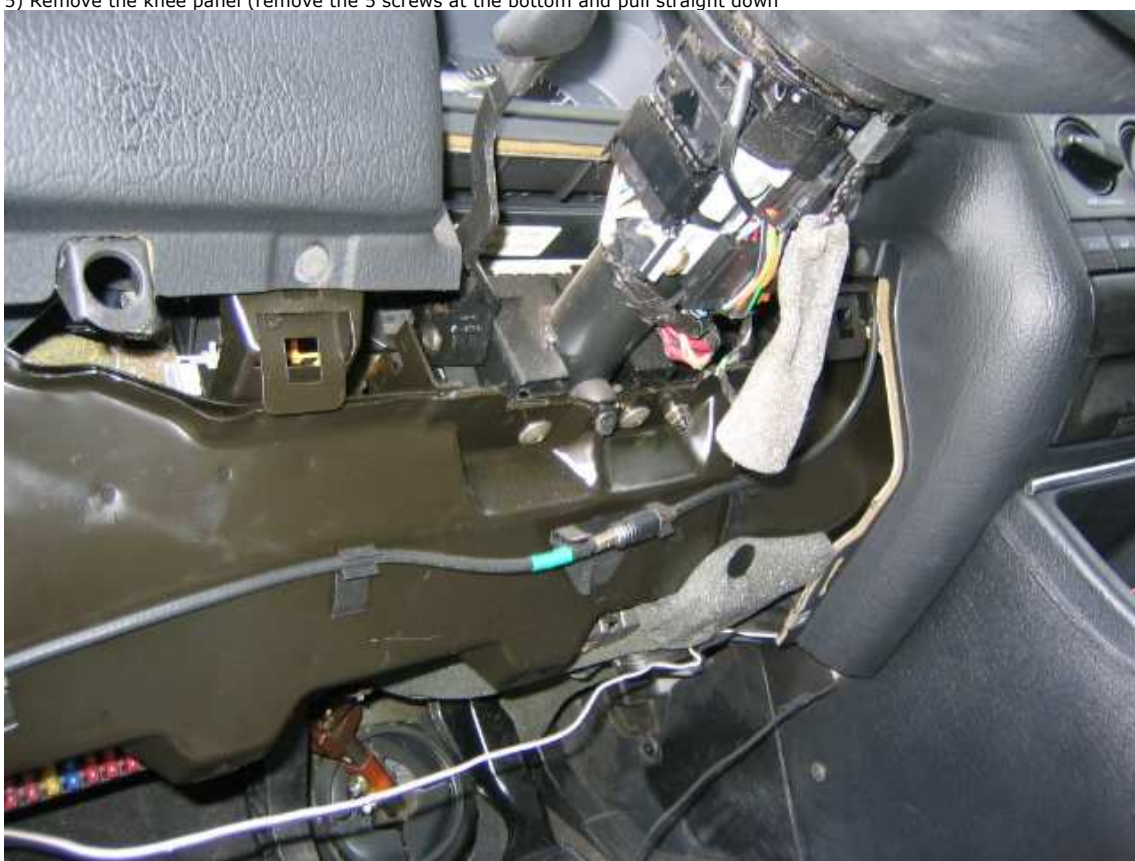
6) Unplug all (8?) wire connectors to the steering column
