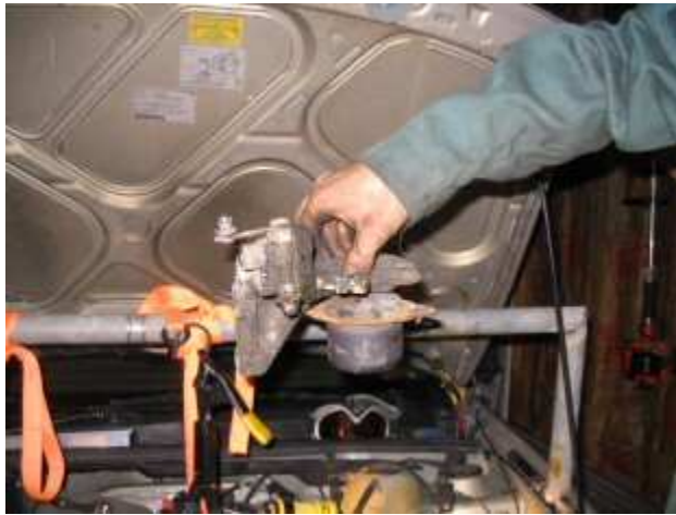
Step 18: Then it was time to remove the tranny mount (you can see it hiding back there). This one is similar to the first engine mount... difficult to remove. The bolt holding it in gave me quite a fight but I was successful in removing it. (as shown in the 2nd pic).
