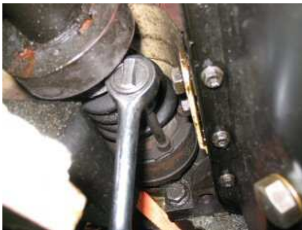
Step 19: Now comes the fun part... removing the drive shafts from the differential. First of all, put a couple of lug nuts back into the rotors of the car... this will prevent the drive shafts from spinning while removing the bolts. For this step you will also need what is called an 8mm "triple square" hex bit. Many people call this tool many different things, but it is available at Autozone (surprisingly) on their wall of special tools. Autozone carries a package of three different sizes, but what you need the the 8mm one... or whatever fits best. I used this tool and successfully managed to strip three of the 12 bolts that hold both drive shafts in place. Don't panic when this happens to you...
