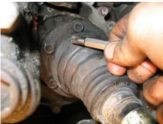
Step 19: Now comes the fun part... removing the drive shafts from the differential. First of all, put a couple of lug nuts back into the rotors of the car... this will prevent the drive shafts from spinning while removing the bolts. For this step you will also need what is called an 8mm "triple square" hex bit. Many people call this tool many different things, but it is available at Autozone (surprisingly) on their wall of special tools. Autozone carries a package of three different sizes, but what you need the the 8mm one... or whatever fits best. I used this tool and successfully managed to strip three of the 12 bolts that hold both drive shafts in place. Don't panic when this happens to you...
