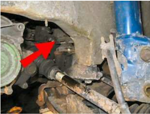
Step 18: Then it was time to remove the tranny mount (you can see it hiding back there). This one is similar to the first engine mount... difficult to remove. The bolt holding it in gave me quite a fight but I was successful in removing it. (as shown in the 2nd pic).
