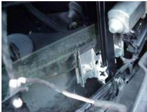
Plug in the switch and roll up and down the window to make sure you have the glass in straight, so the motor doesn't have to labor to roll up or roll down the window.
