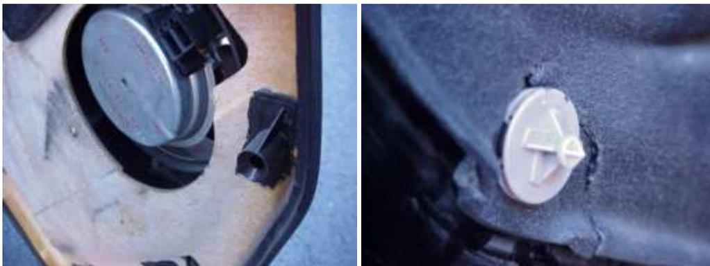
If you pull a pin from the door, don't worry it will go back in, but if you break a pin hole, its all over for that pin hole, so be careful (You shouldn't have any problems)
