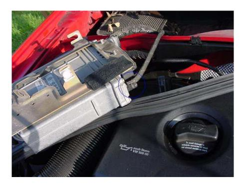
You must remove the boost line shown here. Simply loosen the clamp with a pair of pliers and slide it down the line away from the ECU. Then the boost line pulls off with a bit of force.
