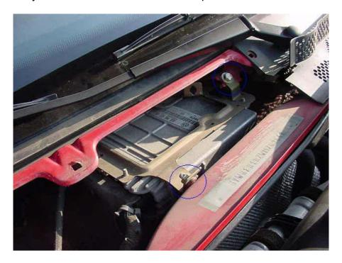
Here's a close up of the ECU. Outlined in blue, there is a 10mm nut and a 10mm bolt. Loosen the nut and remove the bolt to take out the ECU. Once it is loose, pull it to the left and then out of the cubby hole its in so you can access it on top of the engine. I found it useful to take the wire bundle and the boost line out of the first wire holder (see below).
