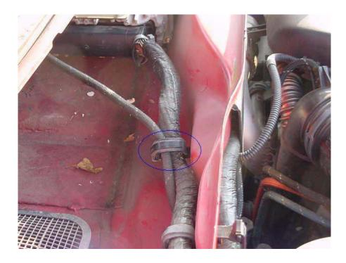
Remove the wire bundle and boost line from this clip for better access and to pull the ECU out onto the engine.
