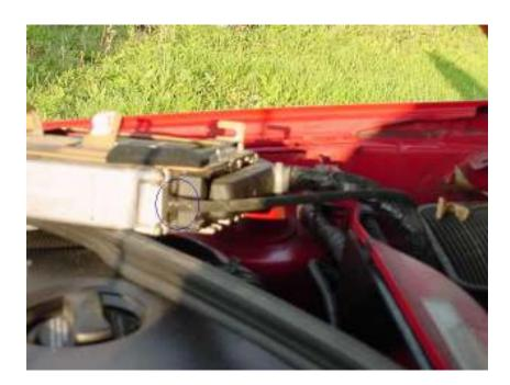
Reattach the electrical connections first, then the boost line.
