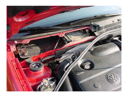
Here the plastic cowling is out of the way. Note the rubber seal that is also pulled out of the way. Inside you can see the ECU mounted in place.
