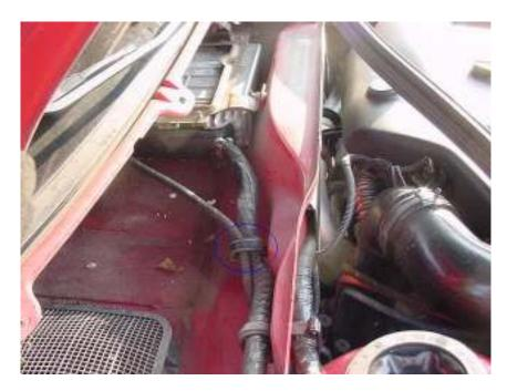
Hook the boost and wire bundle back into the clip so they aren't bouncing around.
