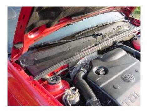
Seal everything back up! Remember, the screw was on the far left. The other three are all the same. Can you see which one I broke? Slide the connecting piece of plastic adjoining both plastic cowlings and reseat the rubber seal. You're all set!
