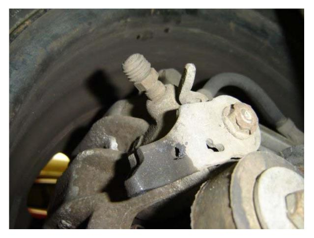
Step 8 -Unclip the brake cable from the back. This requires NO TOOLS.
