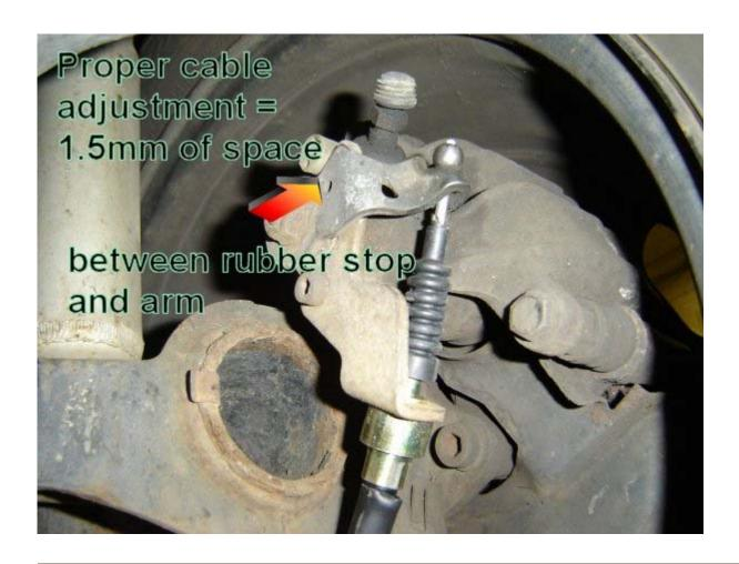
Step 12 - Make sure the wheels spin free, or have a \*little\* drag when the cable is released. And that they lock up within 3 clicks of the brake. Note wire tire (cut the slack off), since the old cable bracket was broken off the axle.. Oh well. Just make sure its not rubbing against the tire, or brake lines.
