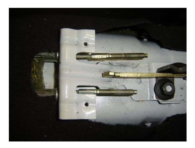
Step 5 - Remove nuts and equalizer bracket. Note how the brake guide tubes press into the white angle bracket.
