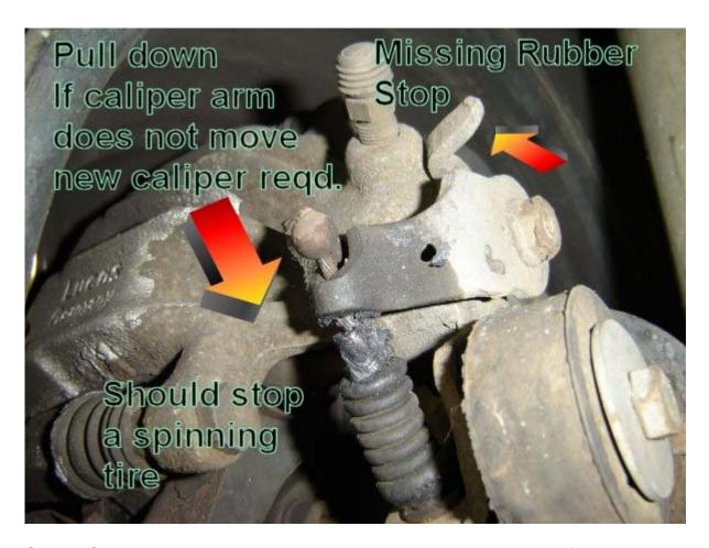
Step 6- Go under the car, and press down on the caliper brake arm. If you can move it by hand, and stop a spinning wheel, good. If not, you need a caliper. Bummer for you. Note the missing rubber stop. **HERE IS A VIDEO**
