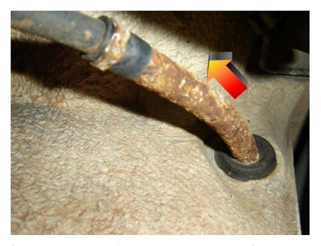
Step 7 - This is the backside of the brake guide tube under the car. Chances are its stuck to the brake cable. No matter, just pull it out.
