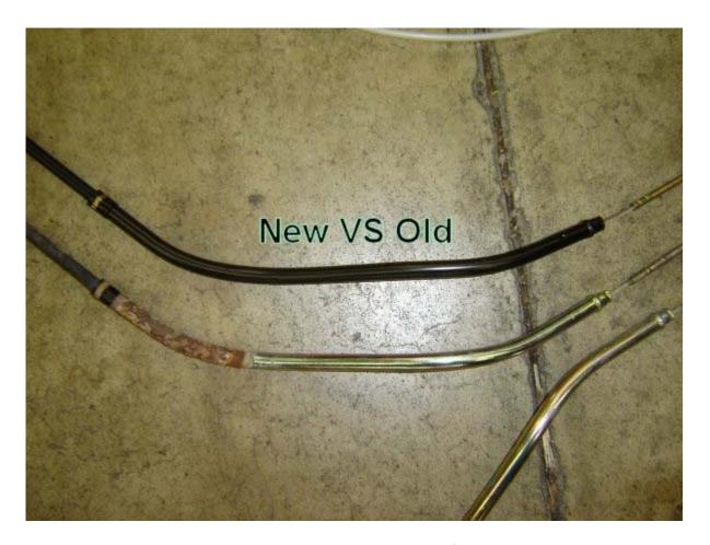
Lie the old cable next to the new cable, don't mix the left and right guide tubes up. The new guide tubes I got were about 1" longer than the older design. No issue here, The new one is the black guide, the old one is the half rust/gold model.
