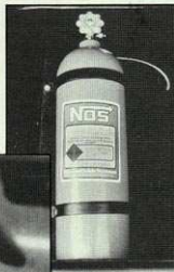
Nitrous oxide bottle mounts in trunk using brackets that are included in kit.
