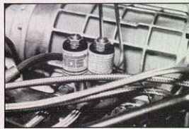
Separate solenoids control delivery of nitrous oxide and fuel to fogger nozzle.
