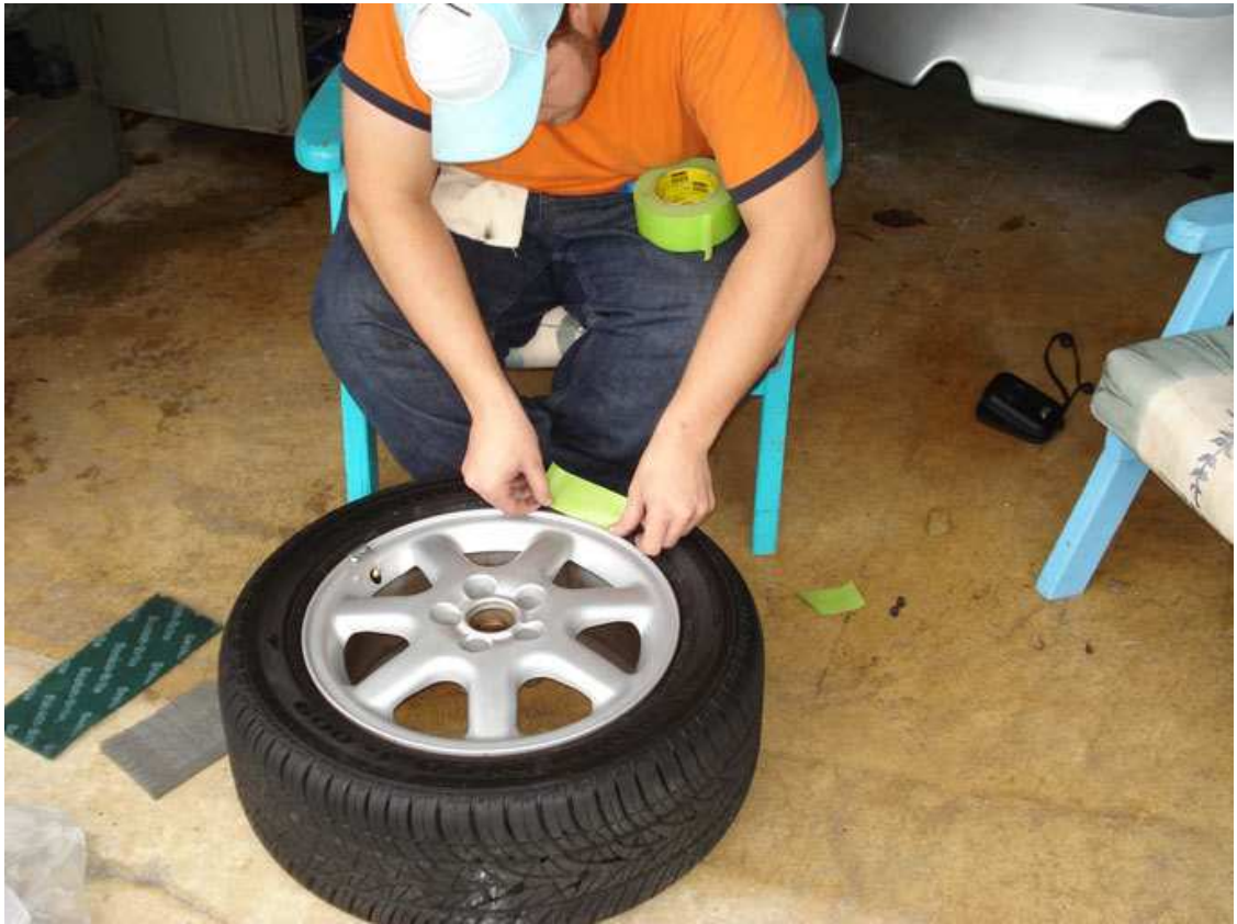
I used pieces of tape maybe 5 inches long, overlapping them to keep it as tight as possible to the edge of the wheel. Make sure to tape off your valve stem also.
