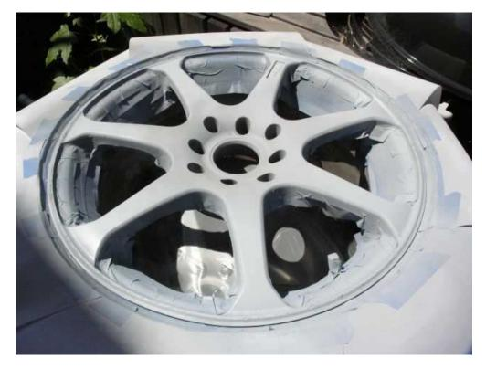
Once the final coat of primer is completely dry (doesn't take too long... follow the directions on the can) I then start painting it. Again, I use multiple thin coats allowing dry time between each coat.
