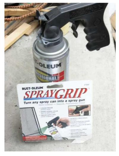
I made several complete passes rather than try to put the primer on too heavy and waited 10-20 minutes between passes to allow the primer to completely dry.
