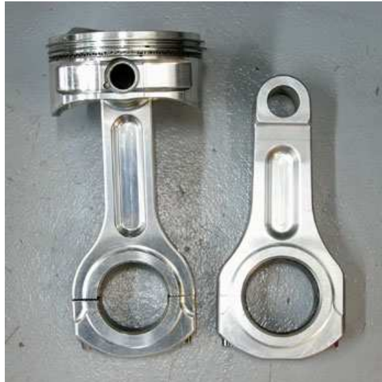
Aluminum rods are difficult to use in stroker engines because they have more mass and usually cause interference in the cam and cylinder bore area. The rod on the left has more clearance than the rod on the right, but it is also weaker.
