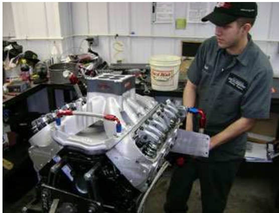
This engine tech is putting the finishing touches on a 400-plus cubic inch small-block Ford. Ford small-blocks have more deck height to work with than small-block Chevys and a little more room inside of the crankcase.
