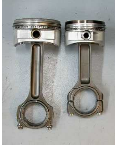
These piston/rod assemblies illustrate a couple of important things to keep in mind when working with stroker motors. No.1, if at all possible, keep the piston pin out of the ring land area, especially for street engines. Both of these pistons are pushing the limit. No. 2, pay attention to rod length if possible. Try to keep the rod/crank ratio as near to stock for street engines and shoot for 1.8:1 for race motors (rod length divided by stroke).
