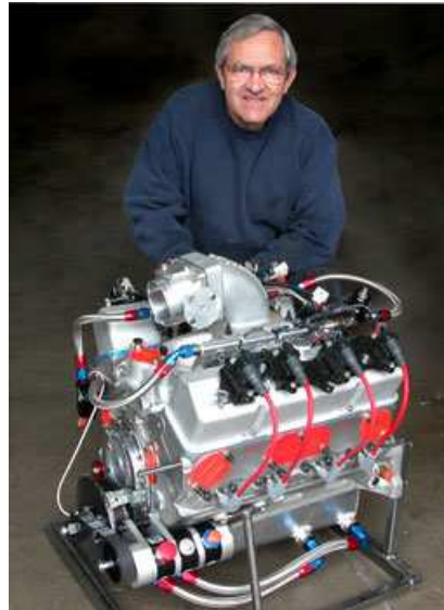
Kenny Duttweiler poses here with an aluminum small-block Chevy awaiting shipping to a customer. This one will be turbocharged, but it shows to what extent you can up-sell the customer if needed. Dry sump oil system and direct-fire ignition system were required for this custom setup.
