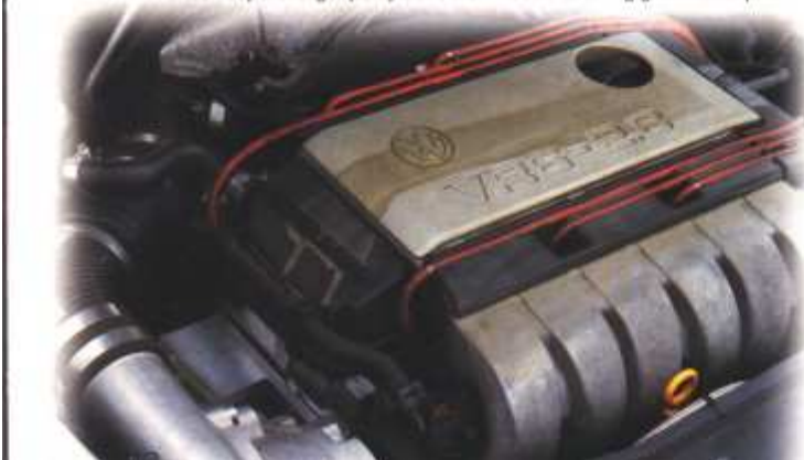
Vortech supercharger pumps this 2.8 VR6 to a chuffing great 250bhp
