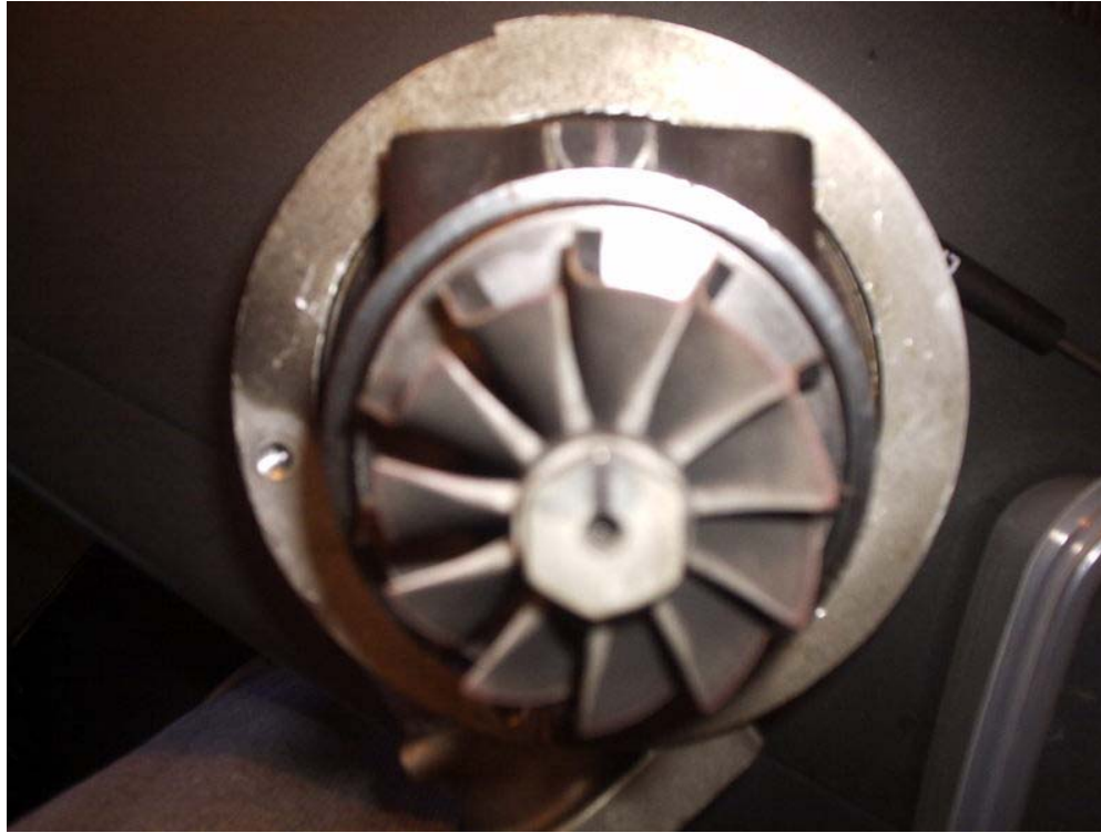
Above shows the relationship markings between the turbine wheel and the CHRA
