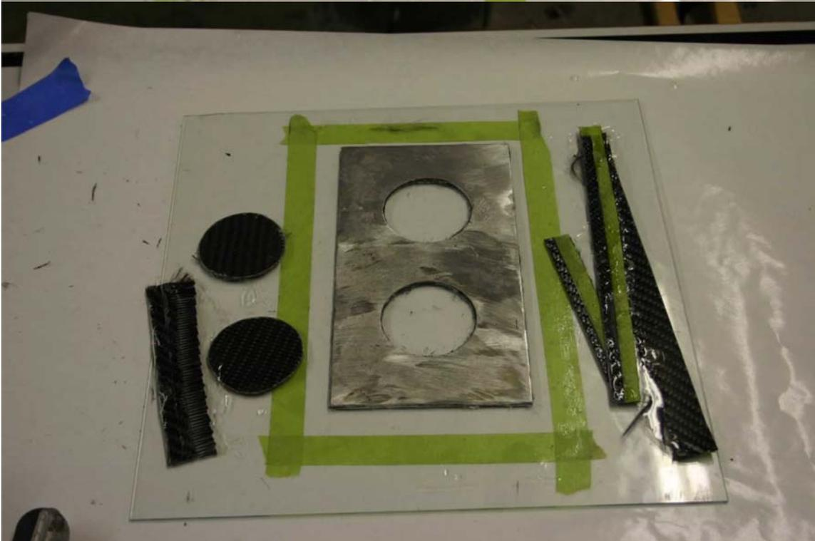
The piece should separate from the glass with little effort. You can use the bondo spreader to ease the part from the glass. The edges will need some trimming. For this the easiest is a dremel tool with a cut off disc and a sanding drum. A sharp xacto blade also
