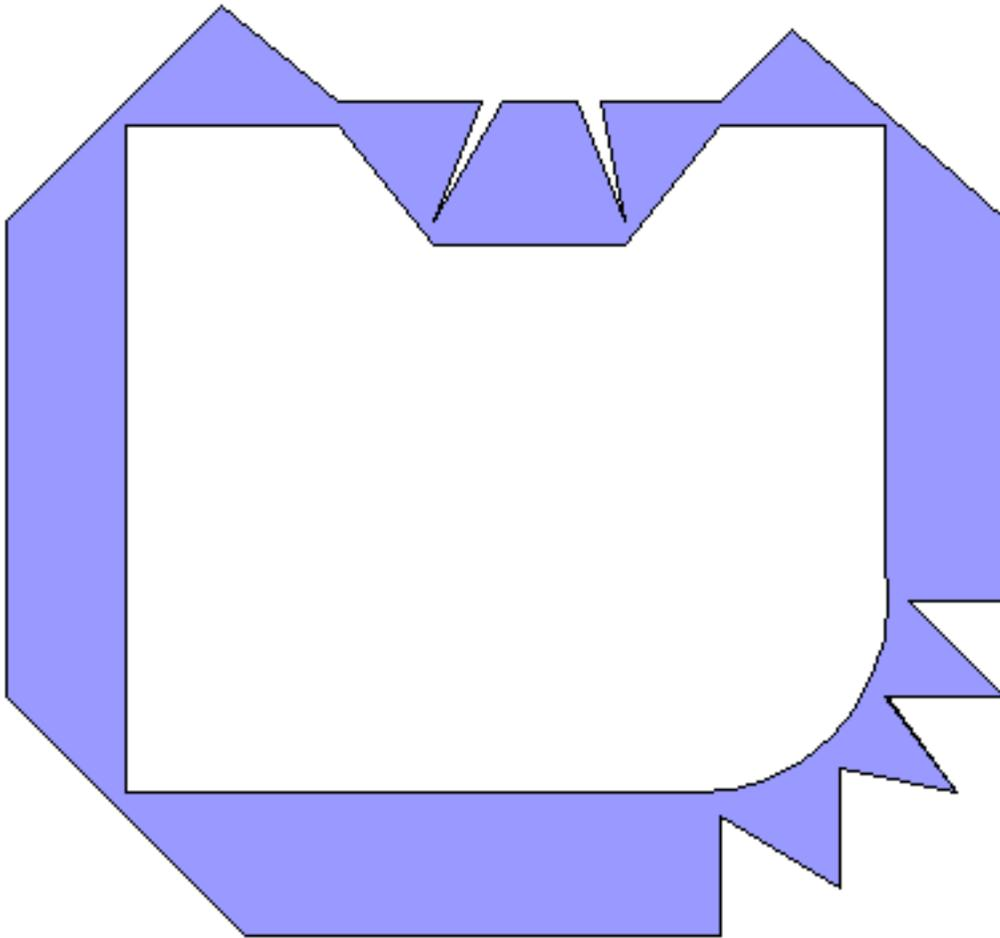
Leave about 1/8" extra material to fold around the edges. This varies with the thickness of the piece. You will need to experiment here.
