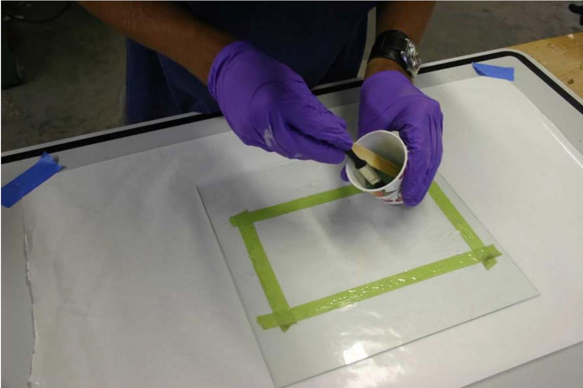
Now lay down your carbon fiber on the wet resin. Pour more resin on the back of the carbon fiber and spread out.
