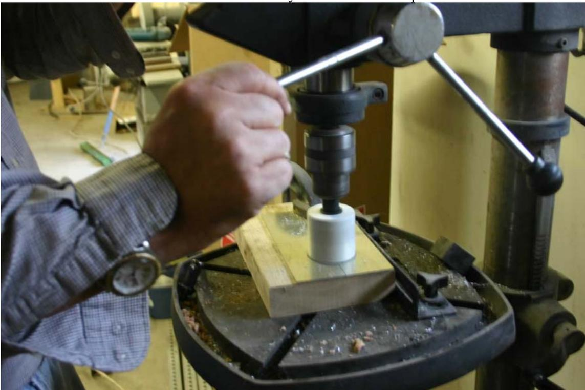
Holes are drilled with a hole saw available at any hardware store. Several places have these cheaply Harbor Freight for one.
