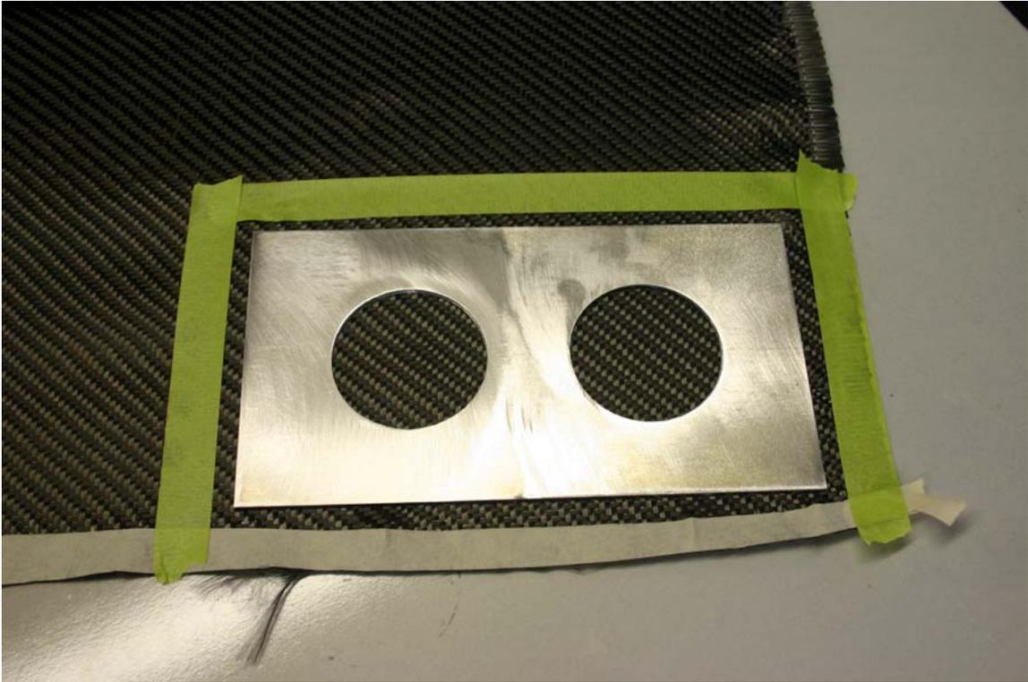
The purpose of taping out the cloth is to maintain the weave without distortion or fraying. By following this simple method you'll keep your carbon pattern straight and will waste very little.
