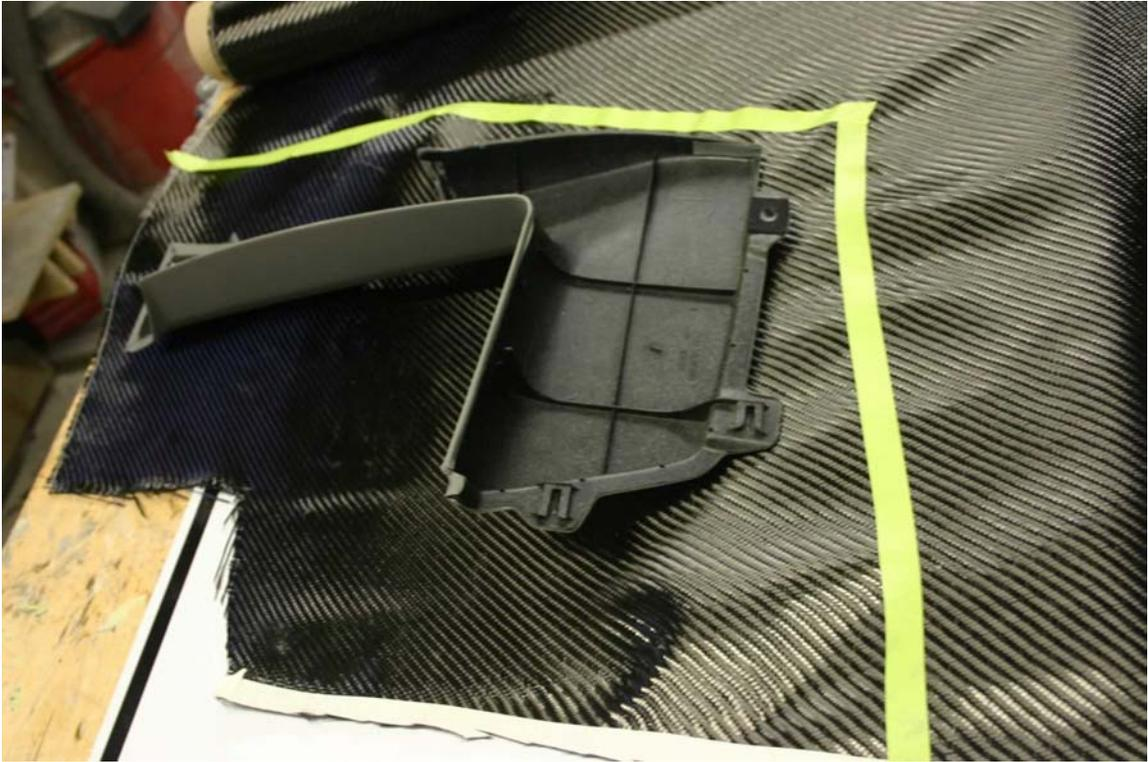
Just like before, place the piece on the carbon and tape the edges.
