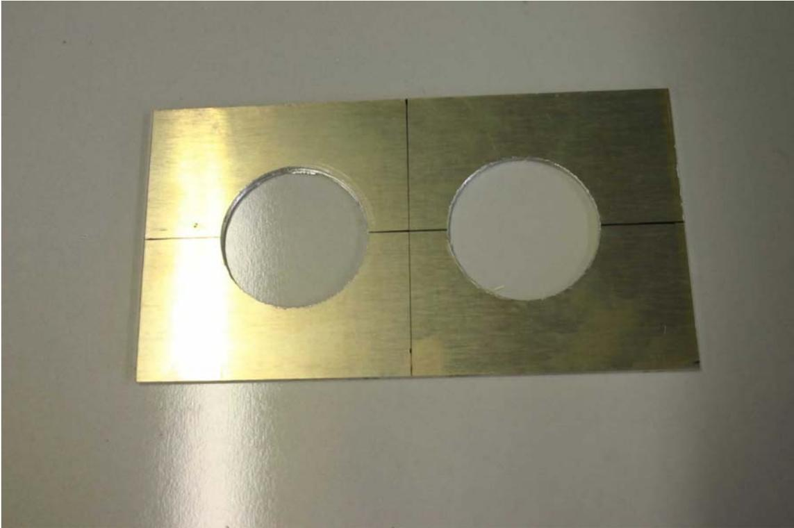
Once the aluminum base is made and fitted carefully to your car opening sand the face side thoroughly with 100 grit sand paper. This is so the resin will adhere to the aluminum, it's very important! After sanding wipe the aluminum with acetone.
