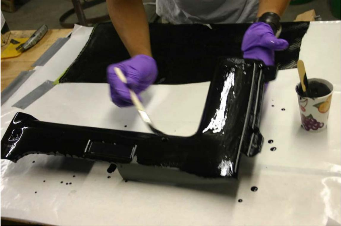
Lay down a coat of resin mixed with hardener over the surface of the piece. Because the part is a light gray I tinted the resin so the gray would not show through the carbon. Tint is very cheap and a little goes a long way. It won't bleed through the carbon fiber. Let the resin dry enough so that when you touch it with your finger it leaves an imprint but doesn't come off on your finger.
