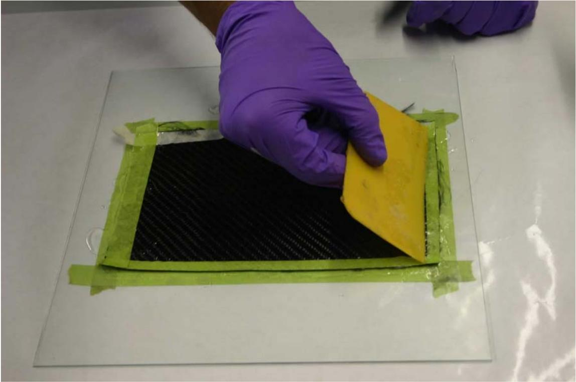
Coat the sanded aluminum side with resin. Place the aluminum down onto the carbon fiber.
