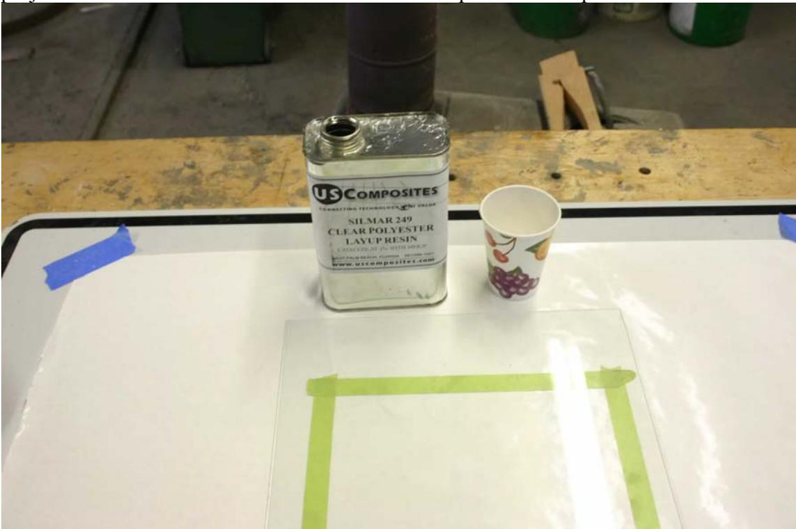
For this step only mix about 1/8 a cup of resin and 5 drops of hardener. Pour the resin on the glass and brush it out to cover completely.
