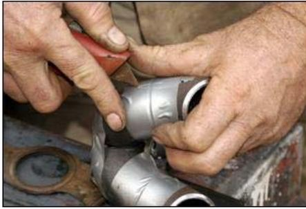
A small portion of the tape was cut away to allow a tack to be made. With the pipe bends then held together, the tape could be stripped off and more tacks – and then a proper weld – made.
