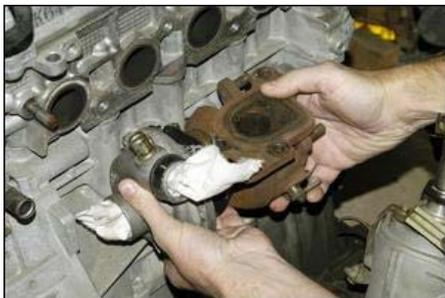
The location of the turbo relative to the head was decided by simply holding the turbo in different positions and judging clearances. From this it could be seen that the manifold runners would probably need to head upwards a little before coming down towards the turbo inlet – that way, the turbo could be kept close to the block without the runners having to bend too sharply.
