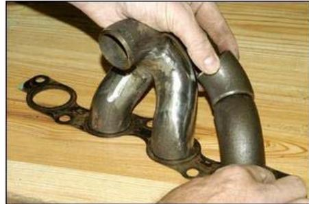
With the centre pipes shaped and then welded together, the outside cylinders could be organised. As can be seen here, again the head gasket is being used to determine pipe spacing. Ninety degree and a 45 degree bends are being used to form this runner, with a substantial amount of the 45-degree bend needing to be cut away. Again a hacksaw was used to do this.
