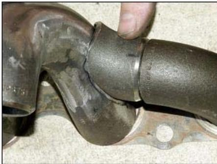
Here's what the 45-degree bend looks like when shaped to match the other runner. An oval-shaped hole was cut on the side of the runner to suit the entering pipe.
