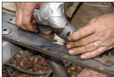
The metal exhaust gasket was used whenever the spacing of the runners needed to be checked. Here the centre two runners can be seen taped together prior to welding. To allow them to nestle together, a section was cut from each 90-degree bend with a hacksaw.
