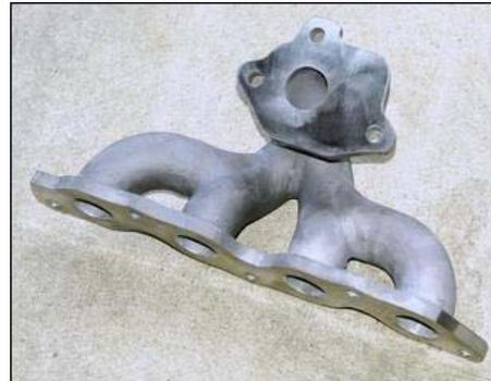
work done by a machine shop, it's also a good time to have the manifold drilled and tapped to take a pressure tapping point and thermocouples (either one per cylinder or one just prior to the turbo).
