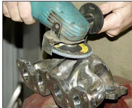
The welds were cleaned-up with an angle grinder spinning a multi-flap sanding disc, and a high speed electric tool using a cutting burr. A round hand file was also used.
