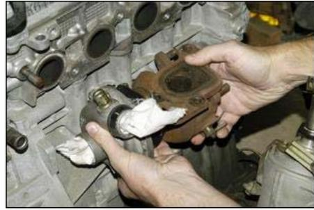
Before any welding is done, it's wise to play around with the bends and manifold plate until the best possible outcome is realised. In addition to gas flow considerations (we'll come to those in a moment), you should also very carefully consider:
