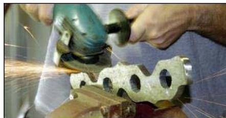
The rough edge resulting from the oxy cutting was smoothed by an angle grinder. The port holes were not smoothed until the runners were welded in place, so that they could then be matched to the ports and the runner internal diameters in the one operation.
