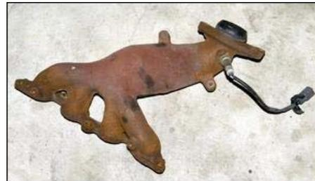
The standard exhaust manifold is a cast iron design that uses short runners grouped 4>2>1 and primary runners about 2¼ inches long. These flow into a large volume before exiting via a 1.5 inch outlet.
