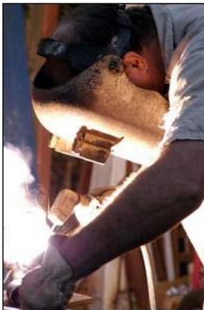
The welding can be done by MIG or stick. Stick (arc) welding allows the selection of a high-strength electrode to suit the application – in the case of the manifold shown here low hydrogen rods were used which are both very strong and also reduce the chance of hydrogen embrittlement.
