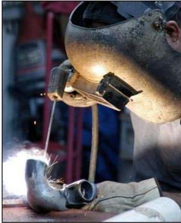
....access for an oxy cutting torch to clean-up the internal transition at the pipe junction. If the 90-degree bend had been welded to the 45-degree bend first, the welding torch would not have been able to gain access to the junction.
