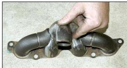
The exhaust gasket is extremely useful as a template for laying out the manifold pipes and showing the required shape of the head mounting plate and the position of the bolt holes. If a gasket for the turbo exists, it can be used in the same way to determine the shape and hole positions of the turbo mounting flange.
