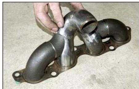
With both 45-degree bends cut to suit, and appropriate holes made in the existing runners, here's what the assembly looked like. Note again how the exhaust manifold gasket is being used for sizing – if you buy a spare gasket and take careful under-bonnet clearance measurements, you can build the manifold without having your car off the road.
