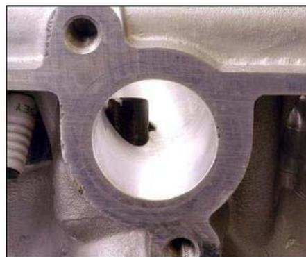
The diameter of the bends is normally matched to the diameter of the ports (or with non-round ports, the cross-sectional area). However, if the ports are very large, a smaller diameter fitting may be used with a transitional cone either incorporated into the first section of pipe or formed within the manifold flange thickness.
