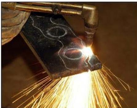
An oxy acetylene torch was used to cut out the manifold plate. The cut was made on the outside of the line so that the resulting plate is a little larger than the gasket. The holes were cut on the inside of the marked line. A local welder did all the cutting and welding – his total time was 5 hours.
