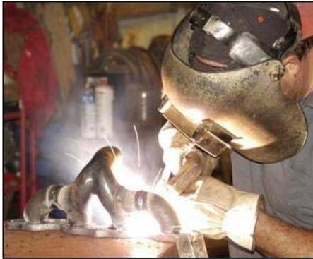
The rest of the runners could then be welded in place, and then welded to the manifold plate. This done, the previously cut out turbo mounting plate could be welded to the collector tube.
