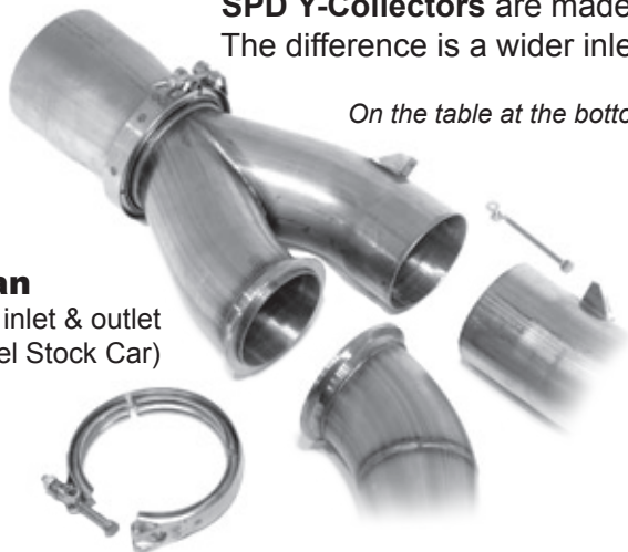
Double Slip shown w/ CWT100 Wing Tabs (Typical SCCA Trans-Am)
