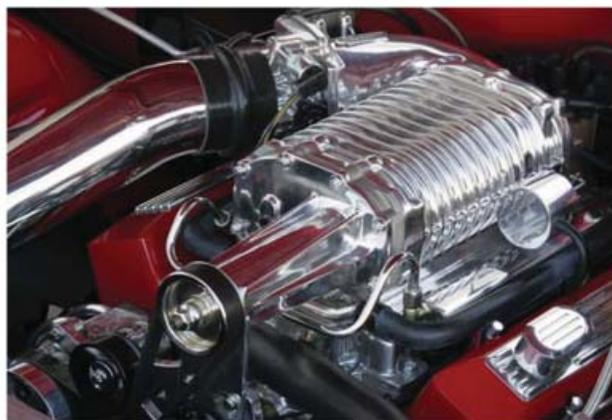
The Gen 1 and Gen 1E Fuel-Injected kit features a MP112 supercharger. This Kit is an Intercooled assembly including Intercooler Assembly, Intake and Top Plate, 42 LB Injectors, Fuel Rails, 78mm Intake, Crank Pulley, Idler Assembly, Dist. Hold Down, Alternator Bracket, 6-Rib Belt, Gaskets, Spacers, and ALL hardware necessary for a complete assembly. One part number includes everything needed for installation! This Kit is available in Raw, Polished, or Silver finish.
