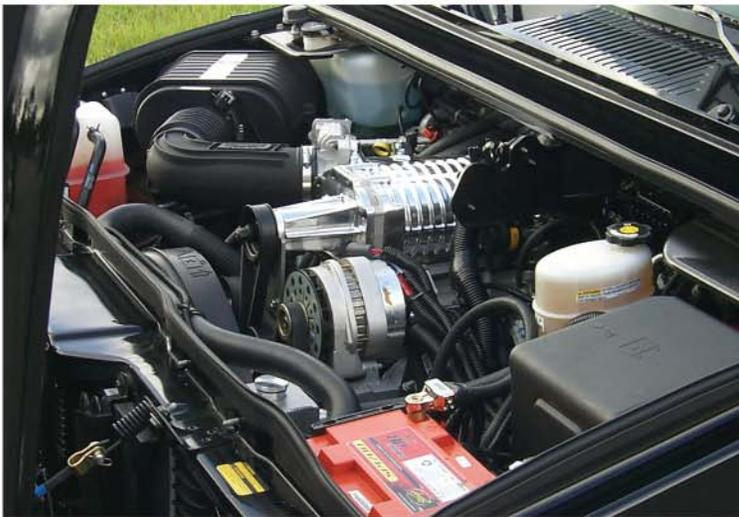
The H2 systems are complete with all components necessary for installation. Included in the kit is the patented cast aluminum intake manifold with equal length runners. Intercooler core, coolant circulation pump, heat exchanger and all necessary hardware to complete the entire installation makes a complete installation package. This kit requires no hood modifications.
