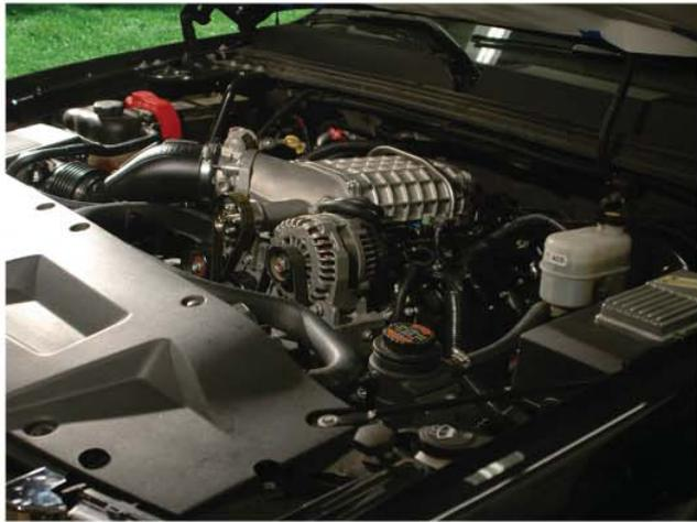
Intercooled systems are complete with all the components necessary for installation. Included in the kit is a new patented cast aluminum intake manifold with equal length runners (replacing the factory nylon manifold), intercooler core, coolant circulation pump, heat exchanger, and all the necessary hardware to complete the entire installation. This system does not require any hood modifications.
