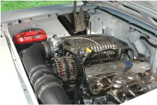
Intercooled systems are complete with all the components necessary for installation. Included in the kits is a new patented cast aluminum intake manifold with equal length runners (replacing the factory nylon manifold), intercooler core, coolant circulation pump, heat exchanger, and all the necessary hardware to complete the entire installation. This system generally does not require any hood modification.
