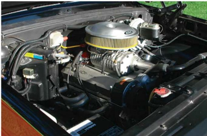
The Gen. 1 & 1E MP-122 H systems are complete with all components necessary for this installation. Included in the kit is the cast aluminum intake manifold and lid assembly, idler, belt tensioner, belt, crank pulley, and new intake manifold gaskets are included as well. This supercharger system is designed to accept any standard flanged carburetor.
