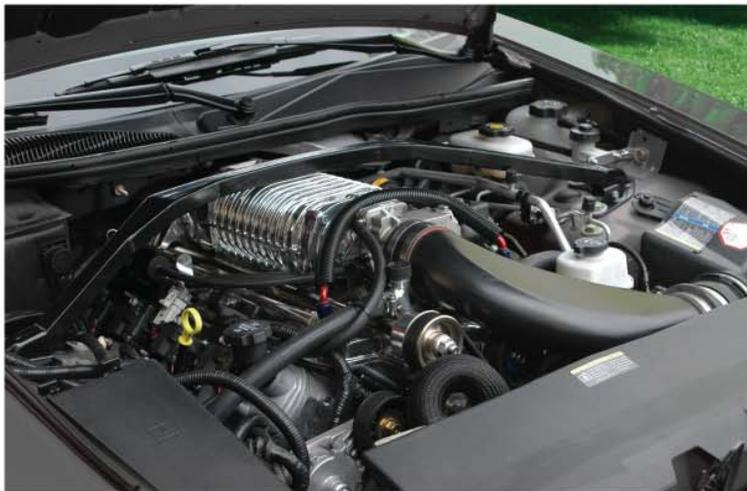
Intercooled systems are complete with all the components necessary for installation. Included in the kit is a new patented cast aluminum intake manifold with equal length runners (replacing the factory nylon manifold), intercooler core, coolant circulation pump, heat exchanger, and all the necessary hardware to complete the entire installation. This system does not require any hood modifications.
