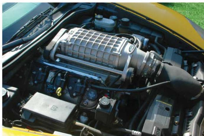
MagnaCharger supercharger kits are complete with all components necessary for installation. Included in the kit is the cast aluminum intake manifold, factory “push - lock connectors” are utilized in the fuel system for installation ease, intercooler core, coolant circulation pump, heat exchanger and all necessary hardware to make a complete installation package. This system requires hood modifications. Magnuson has both C5 and C6 hood suggestions available.
