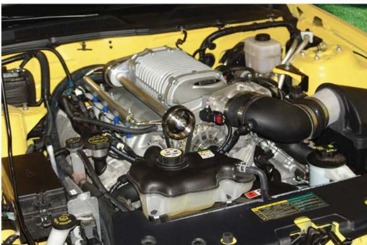
Mustang 3V supercharger systems are complete with all components necessary for installation. Included in the kit is the cast aluminum intake manifold, factory "push - lock connectors" are utilized in the fuel system for installation ease, intercooler core, coolant circulation pump, heat exchanger and all necessary hardware to make a complete installation package. This system does not require any hood modifications.
