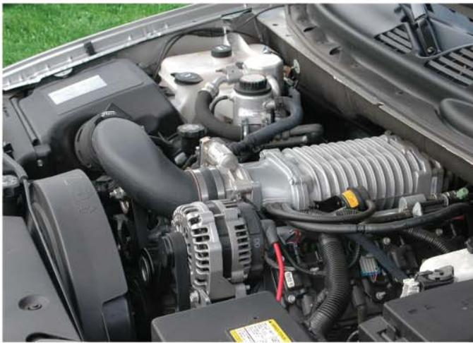
Intercooled systems are complete with all the components necessary for installation. Included in the kit is a new cast aluminum intake manifold (replacing the factory nylon manifold), intercooler core, coolant circulation pump, heat exchanger, and all the necessary hardware to complete the entire installation. This system does not require any hood modifications.
