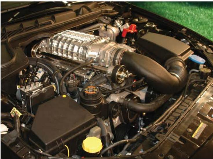
Pontiac G-8 supercharger systems are complete with all components necessary for installation. Included in the kit is the cast aluminum intake manifold, factory "push - lock connectors" are utilized in the fuel system for installation ease, intercooler core, coolant circulation pump, heat exchanger and all necessary hardware to make a complete installation package. This system does not require any hood modifications.
