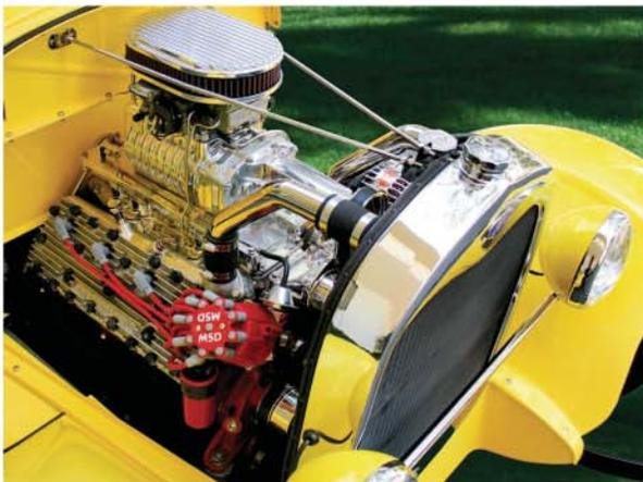
The Ford Flathead system accommodates virtually any 4-barrel carburetor with a standard Holly foot print. Recommended air intake should be in the 500 to 850 CFM range. Patented cast aluminum manifold with pop-off safety valve and cross-flow equal-length intake runners that result in higher torque. The internal bypass valve virtually eliminates parasitic loss, now that's real efficiency.
