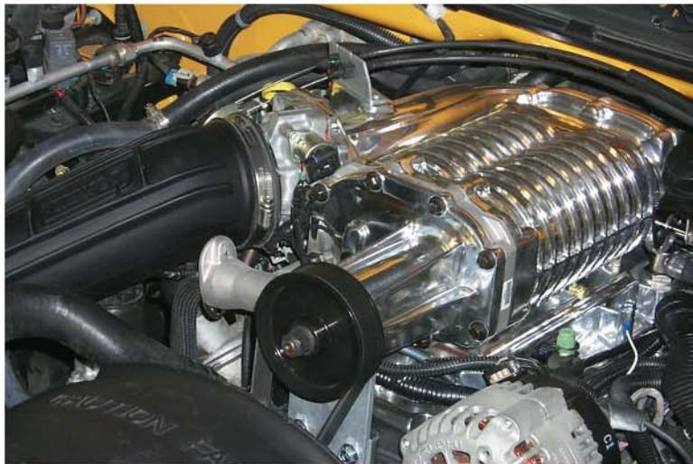
Magna Charger Radix systems are complete with all components necessary for installation. Included in the kit is the patented cast aluminum intake manifold with equal length runners. Intercooler core, coolant circulation pump, heat exchanger and all necessary hardware for the entire installation makes for a complete installation package. This kit doesn't require any hood modifications.
