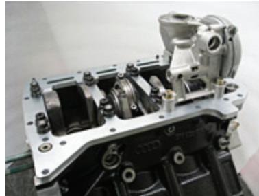
Main Bearing Girdle S4
