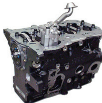
2 Liter 058 Type with Main Bearing Girdle*
