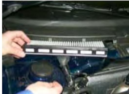
4. Remove used filter from top housing plate and replace with clean cabin filter. Make sure to line up the four notches on the top side of the filter with the ribs on the top housing plate. Replace filter and top housing plate by pushing it down until the two tabs click into place. Reattach cover.
