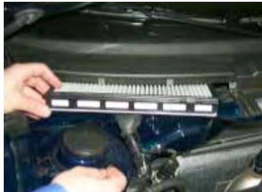
4. Make sure to line up the four notches on the top side of the filter with the ribs on the top housing plate. Replace filter and top housing plate by sliding into place and pushing down until the two tabs click into place. Reattach cover.
