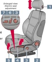
Adjusting seat height and moving seat backwards or forwards (electrical adjustment)
