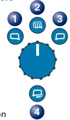
Press the adjuster to move the mirror surface in the desired direction.
