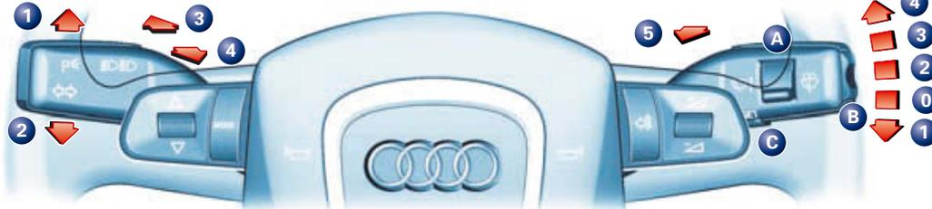
**[11] Control lever for windscreen wipers/washer and on-board computer**
