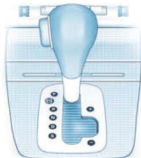
To move the selector lever out of position P or N, or into position P or R, press the interlock button on the selector lever handle and the brake pedal simultaneously.
