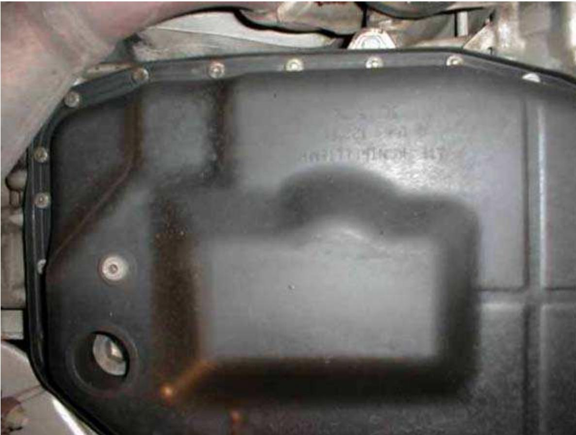
*This is the transmission pan. The small bolt is the drain, the large one is the fill. The bolts are Torx bolts, size T-27. Why Torx and not Allen? Why T-27 instead of the more common T-25 or T-30? We must all make sacrifices to the Audi Gods.*
