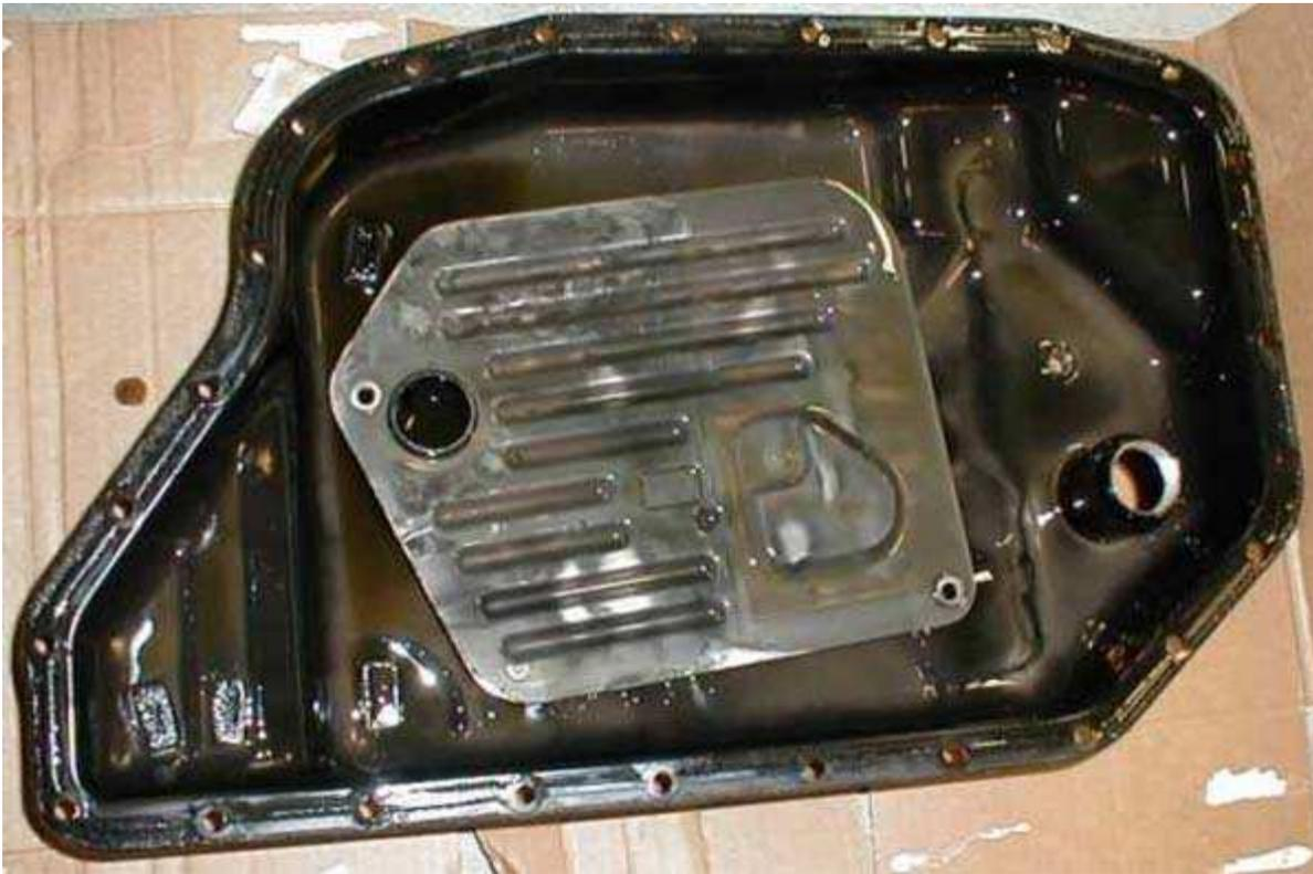
*The filter has been removed. Here you can see that it is also covered in sediment.*
