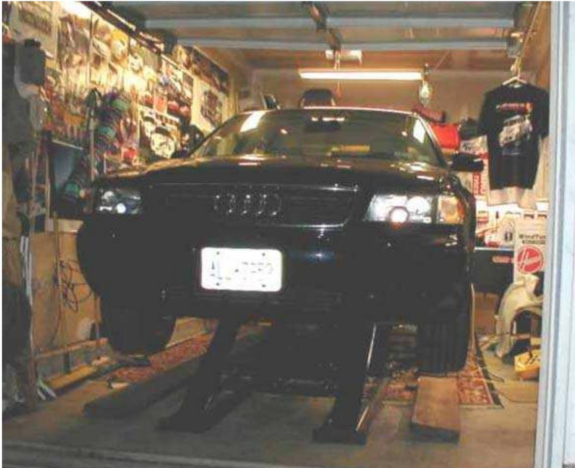
*The victim ready for work. Note that the car should be level for this procedure. If not, you can't properly fill the transmission. Put the car up on four jack stands if you don't have your own lift. See picture at top of this procedure for jacking points. Use jackstands at the rocker panel jack points to support the car. It must be level to perform this procedure.*
