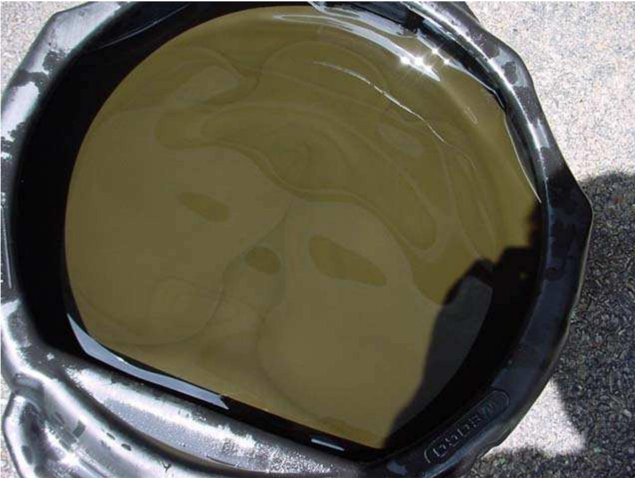
*Transmission fluid from above transmission. See how bad it can get? It's NOT a lifetime fluid!
