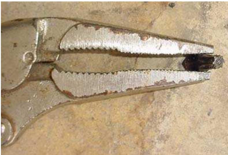
*Ground down T-27 bit in vice grips. This will allow you to get the two hidden T-27 screws out without dropping the exhaust.*
