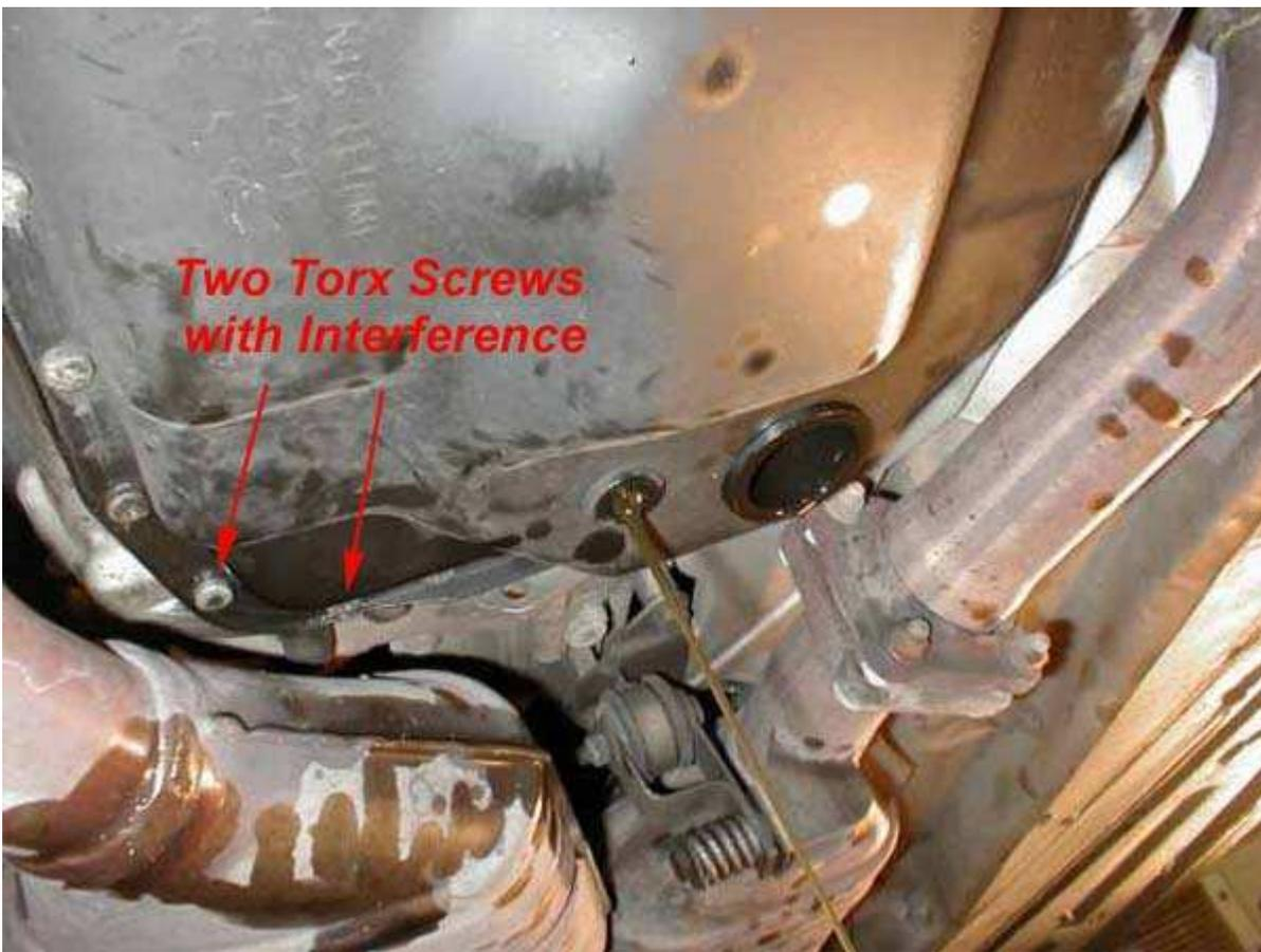
*Transmission fluid draining. Be prepared for about 6-7 quarts to drain. Note that the Audi fluid is not red like every other transmission fluid. It's sort of yellowish green. Mine was in much better condition than I anticipated. It was still clear, not burnt and did not smell rancid or overheated.*
