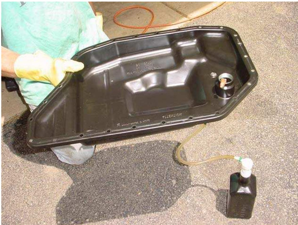
*How pan stand pipe works to control level. Fluid is pumped into the transmission pan until the level reaches the top of the stand pipe. It then overflows out of the transmission. This level is higher when the car is not running versus running due to the hydraulic pump pumping fluid through the transmission.*
