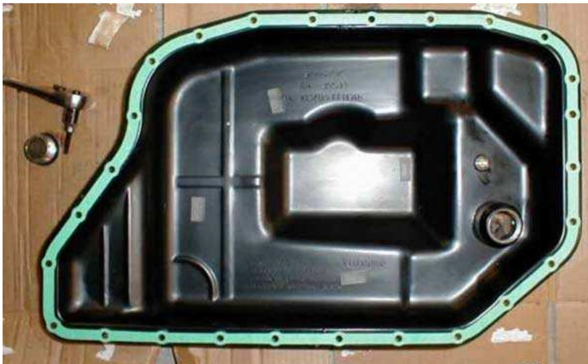
*Clean pan, drain bolt installed, gasket placed. I use a dab of vaseline to hold the gasket in position until it can be bolted in place.*
