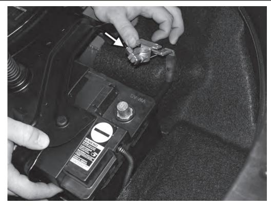
55) Reinstall the negative battery terminal, and secure with the 10mm nut.
