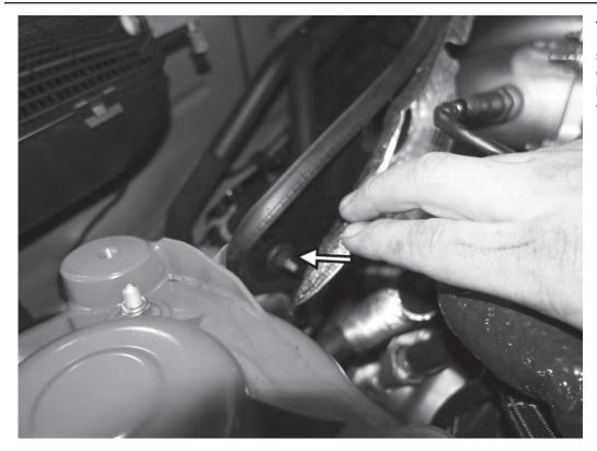
47) Secure the bulkhead with the 10mm nut located under the right side of the front bulkhead heat shield. Once installed, bend the heat shield back and reinstall the metal clip over the threaded stud.
