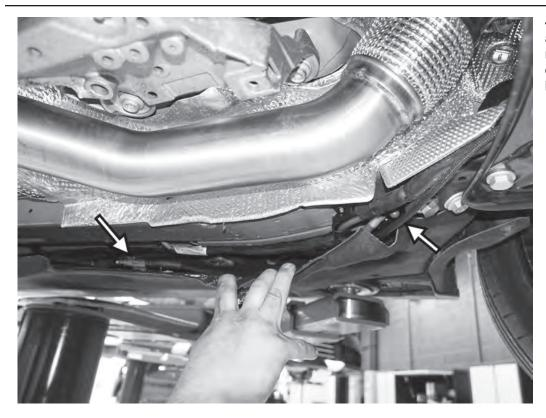
43) Pull down the underbody panels and route the oxygen sensor harnesses with the extensions on the outside of the frame rail, where other harnesses and hoses are routed.
