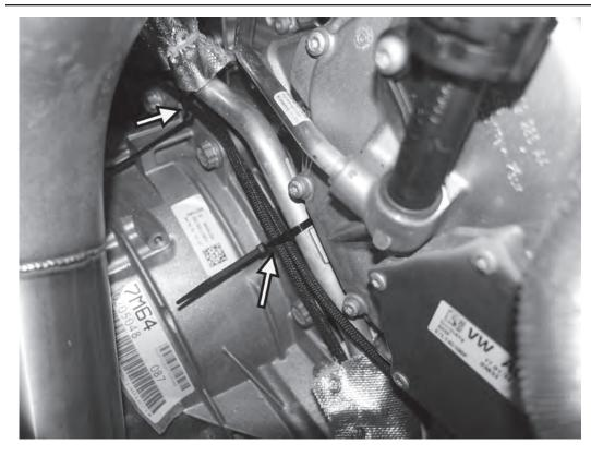
29) Secure both APR extension harnesses (the left one going to the right and the right one going to the left) to the coolant pipe that runs over the top of the transmission.
