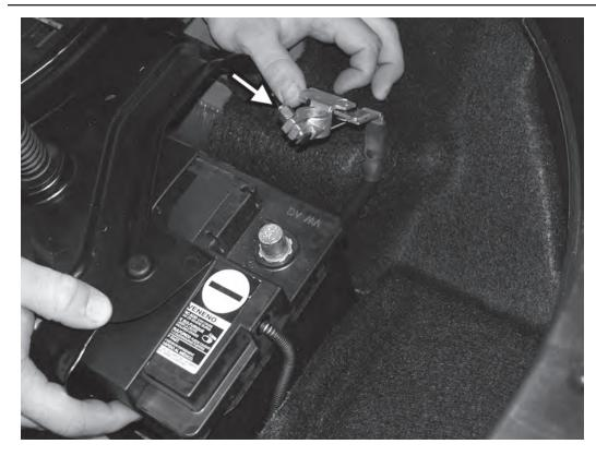
3) In the trunk, disconnect the 10mm nut securing the negative battery terminal, and remove the negative terminal from the battery.
