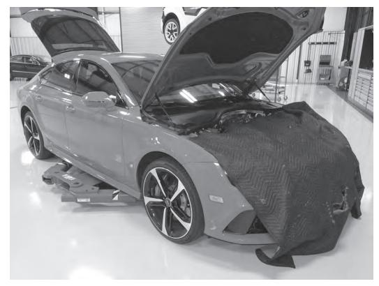
1) Secure the vehicle on a lift or jackstands.
