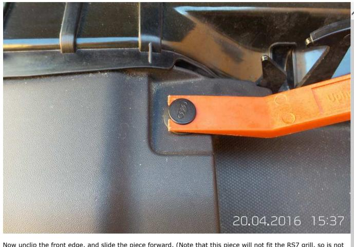
Now unclip the front edge, and slide the piece forward. (Note that this piece will not fit the RS7 grill, so is not reusable - you will need to purchase the RS7 specific piece)
