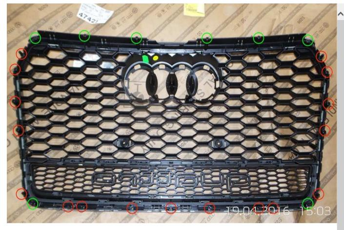
Alignment of the original S7 grill is through the use of the lock tabs on the grill itself, and the alignment tabs located around the bumper opening. Each of the bumper tabs locates into the channel that runs around the outside of the original S7 grill.
