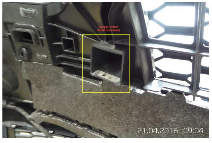
Ensure you align the bottom bumper screw holes with the front of the bottom <u>engine</u> cover tray. The blank tabs go on top, the screw tabs go underneath.
