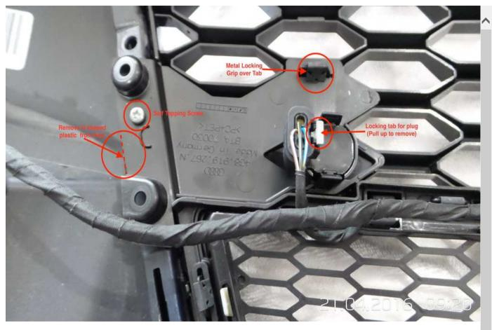
If you're A/S7 has the black optics pack, then the <u>parking sensors</u> will already be coloured black. If they are grey, simply remove the rubber grommet from the sensor and spray paint them black. Two coats (no primer) was plenty. Allow to dry then push fit into the mounting points you have just fitted. You can now reconnect the cables to the sensors and tidy the wires up.
