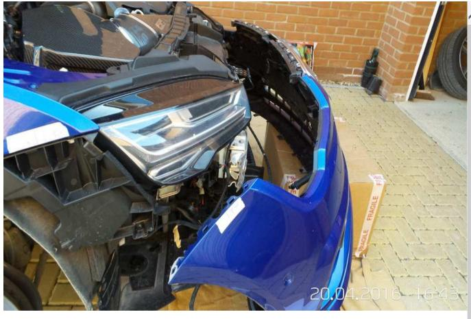
• Support the bumper (on boxes) while disconnecting the following connections, where relevant to your model: o <u>Parking sensors</u> – single plug assembly on the right hand side (as you face bumper) It's a b\*tch to unplug, as the locking tab is hidden underneath the plug as installed. You can unclip the plug from the bumper and use a small bladed screwdriver to help with separation.
