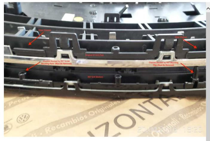
There are no locking tabs on the RS7 grill, only mounting pegs (to guide alignment) and T20 Torx screw mounting points. The only useable screw mounting points are the 6 across the top of the grill, and the bottom left and bottom right ones. Everything else must be removed – pegs and screw mounting points.
