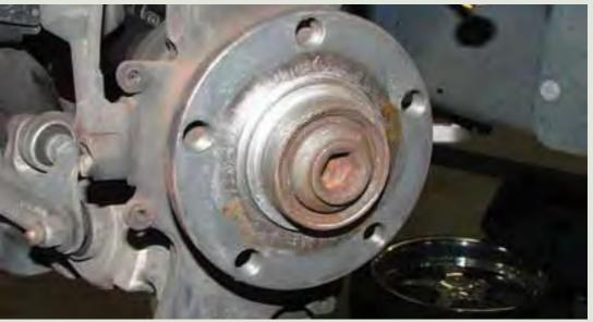
This step applies only to early B5S4 models fitted with steel knuckles (*bearing holders* in Audi-speak). Omit this step if your car has aluminum knuckles.
