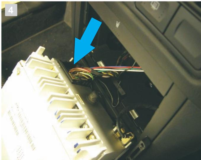
4. CD changer interface will be on left hand side of radio, it is the smaller left-hand connector on the bottom of the harnesses.
