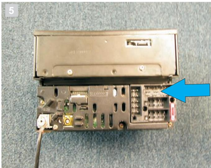
5. Shown is the CD Changer harness through the back of the radio. The vehicle specific cable will be interfacing from this point.
