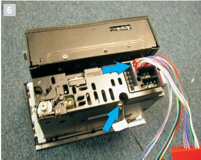
6. Insert the vehicle specific cable into the specified connector. Make sure the connector is fully inserted and that it snaps in place.
