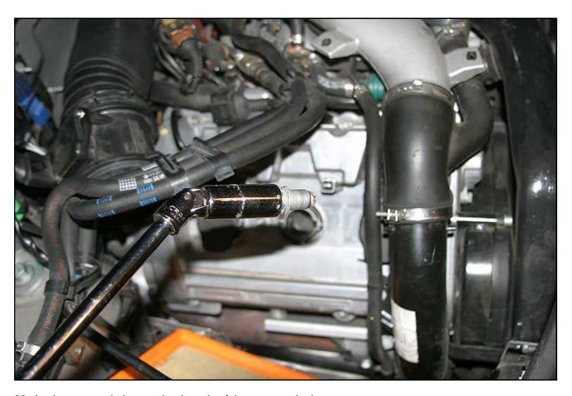
22. Apply some anti-sieze to the threads of the new spark plug.
