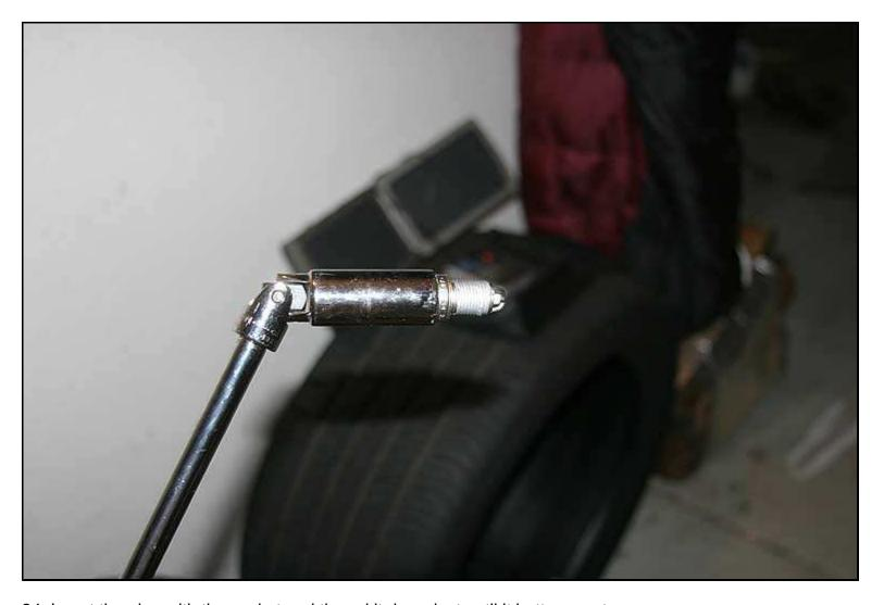
24. Insert the plug with the socket and thread it down just until it bottoms out.
