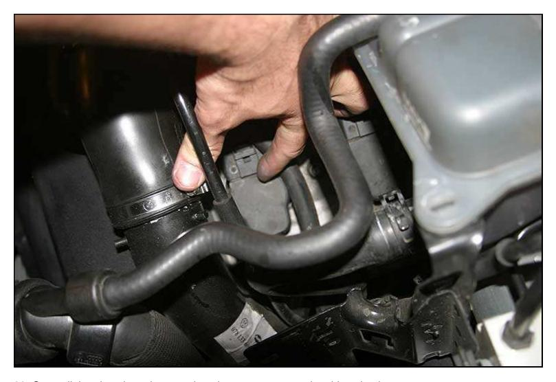
29. Once all the plugs have been replaced, you can start putting things back together. Prepare the airbox by inserting the O-ring into the round airbox opening. You'll see three tabs around the circumference of the opening that hold it in place.
