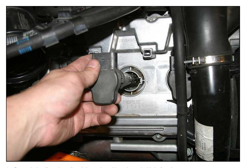
27. Reattach the clip to the coil pack (sometimes it's easier to do this before the coilpack is fully inserted).
