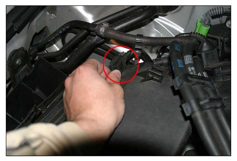
10. Release the pressure clips holding the top of the airbox down. There are four clips, one near each corner. Just push them outward, away from the center of the airbox and they will snap out of their locked position into an open position. The clip on the bottom nearest the firewall is the hardest to get at. Using a screwdriver and pushing on the clip can make it easier.
