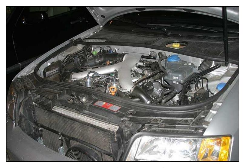
The first things we're going to do is prep everything for the replacement of the plugs. This requires removing the airbox and the coolant tank / resevoir from their mounted locations. First, the airbox.
