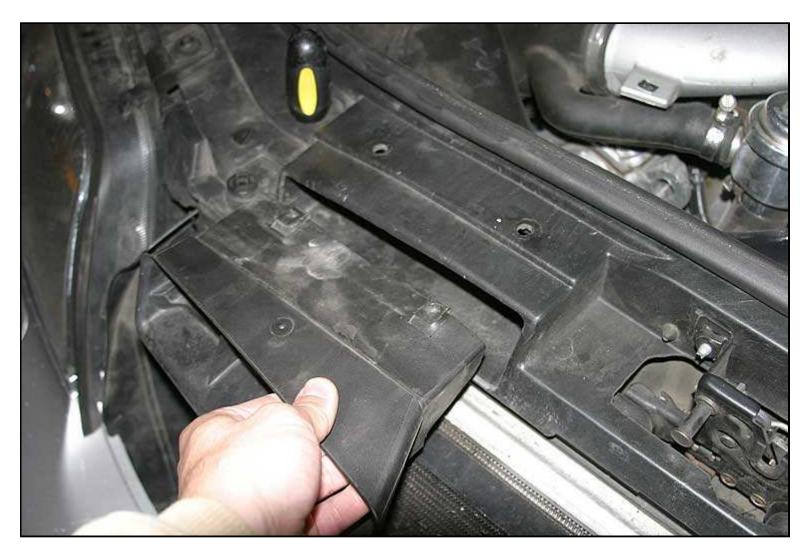
6. After removing the scoop, remove the plastic neck by pulling up on the end closest to the airbox (the end will release easily from a clip) and then by sliding the neck rearward and up.
