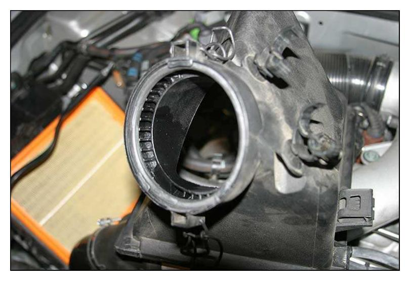
30. Re-seat the top of the airbox and close the 4 clips back to the locked position by snapping them back in place. Use the clothes-hanger airbox clip puller tool to hook onto the bottom clip near the firwall, and just give it a gentle tug to snap that otherwise hard-to-reach clip into place.
