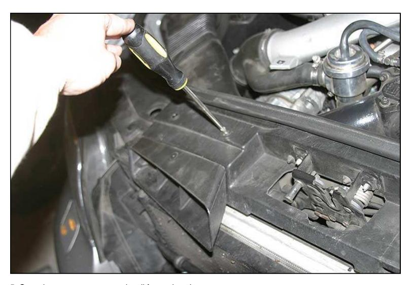
5. Once the screws are removed, pull forward on the scoop.
