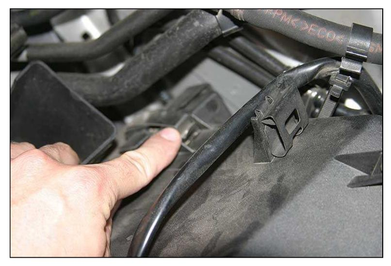
11. Once all the clips are opened,remove the MAF housing from the airbox. Be carefull, because there is an O-ring in there that might want to jump out. Set the O-ring aside.
