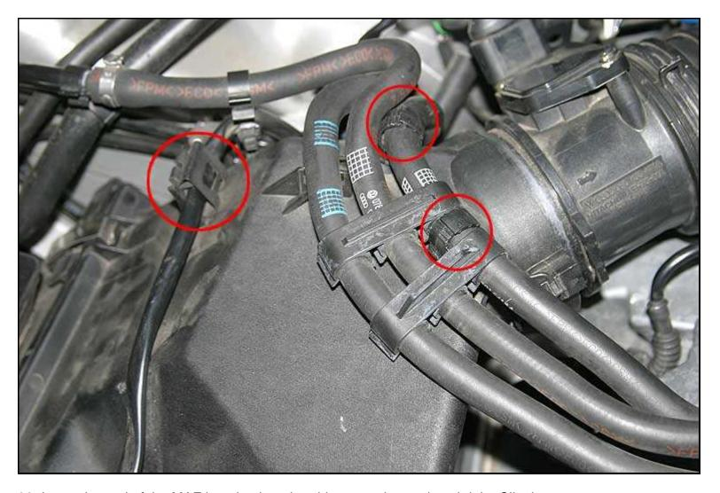
32. Insert the end of the MAF housing into the airbox opening and push it in. Clip the ends of the Grolsch style clips into the MAF housing, and close the clips.
