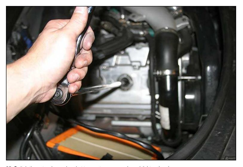
25. Switch the extension and socket to your torque wrench, and tighten the plug down with torque set at 22ft/lbs.
