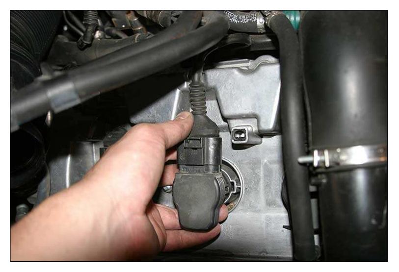
28. Repeat the process for the rest of your plugs. The plug closest to the front of the car on each side are the hardest to work with. You will have to navigate the coilpack through some hoses. Just be patient. In some cases, it may be easier to remove the clips from the coilpacks after they have been raised a bit.
