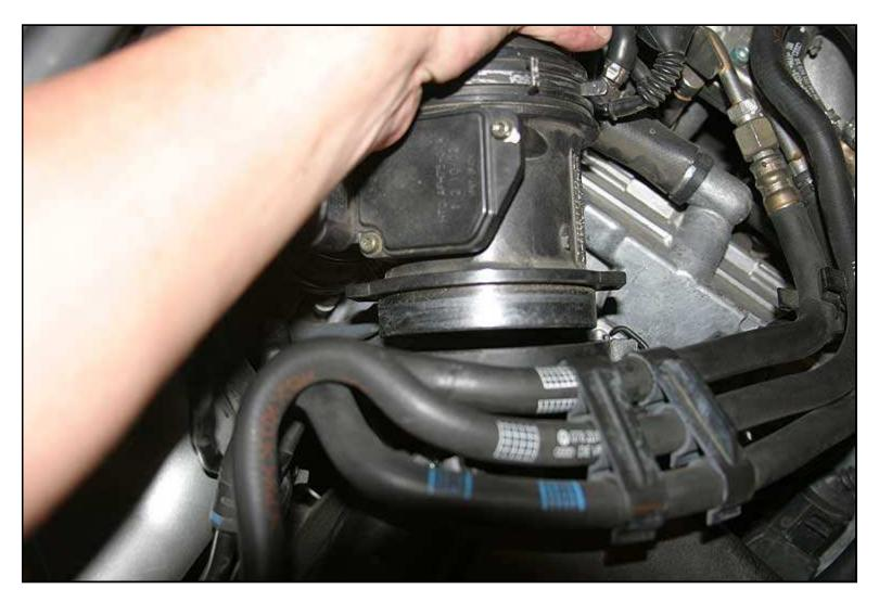
12. Remove the top of the airbox. You might have to finesse it out a bit to get it to clear the wiring and hoses you uncliped from the top (BTW, now would be a good time to check your air filter or clean it, while you're in there).
