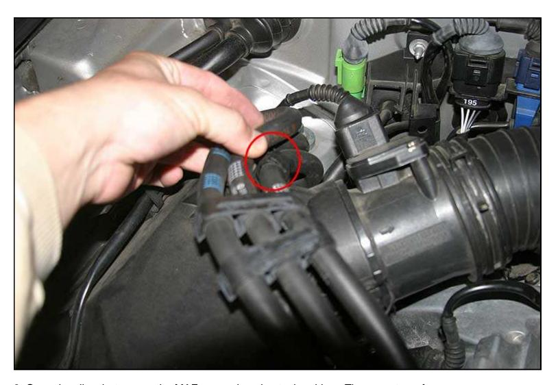
8. Open the clips that secure the MAF sensor housing to the airbox. There are two of them - one facing foward, and one between the MAF housing and the firewall. The operate just like the clips on top of bottles of Grolsch.
