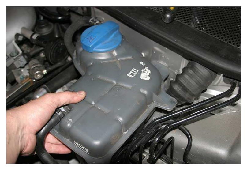
17. Use a flat-head screwdriver to release the clip and sensor from the bottom of the coolant resevoir.
