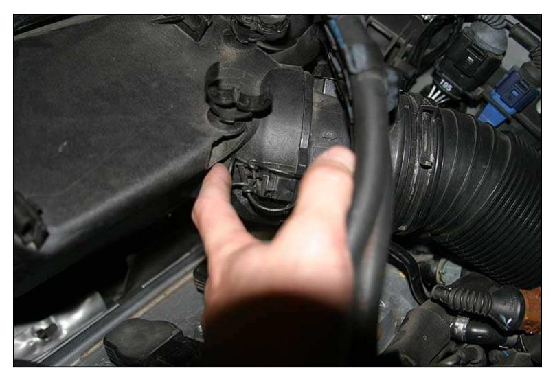
9. Remove the wiring from the clip on the top, fender-side of the airbox.
