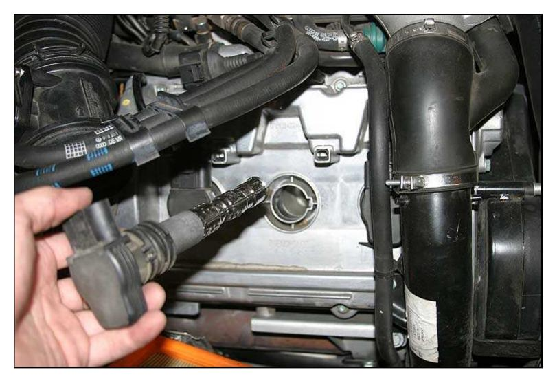
20. Get your socket and stick that baby down in there. That's what I'M talking about! NOW we're having fun! Rotate the socket until it mates with the plug. Once you've got it on, apply firm pressure to loosen and remove the plug. Don't try to impact it loose - you don't want to break it off in there. Just apply firm, controlled pressure and it will come free and out.
