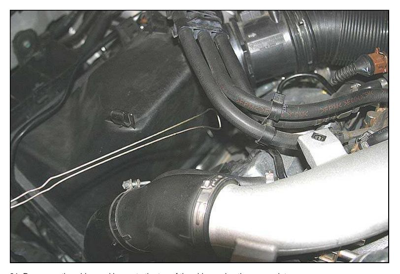
31. Re-secure the wiring and hoses to the top of the airbox using the appropriate clips.
