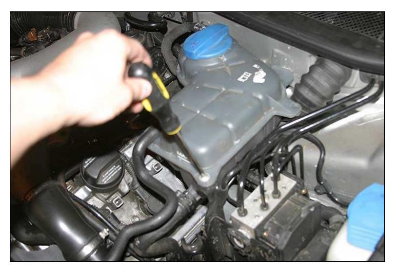
16. Dismount the tank by pulling forward and up, with a scooping motion. Don't pull too hard, though, as there's a sensor on the bottom that you'll need to disconnect.
