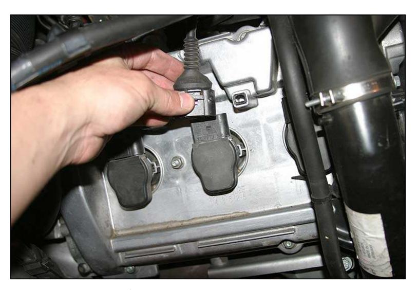
19. Pull the coilpack straight out firmly but smoothly, and set it aside.
